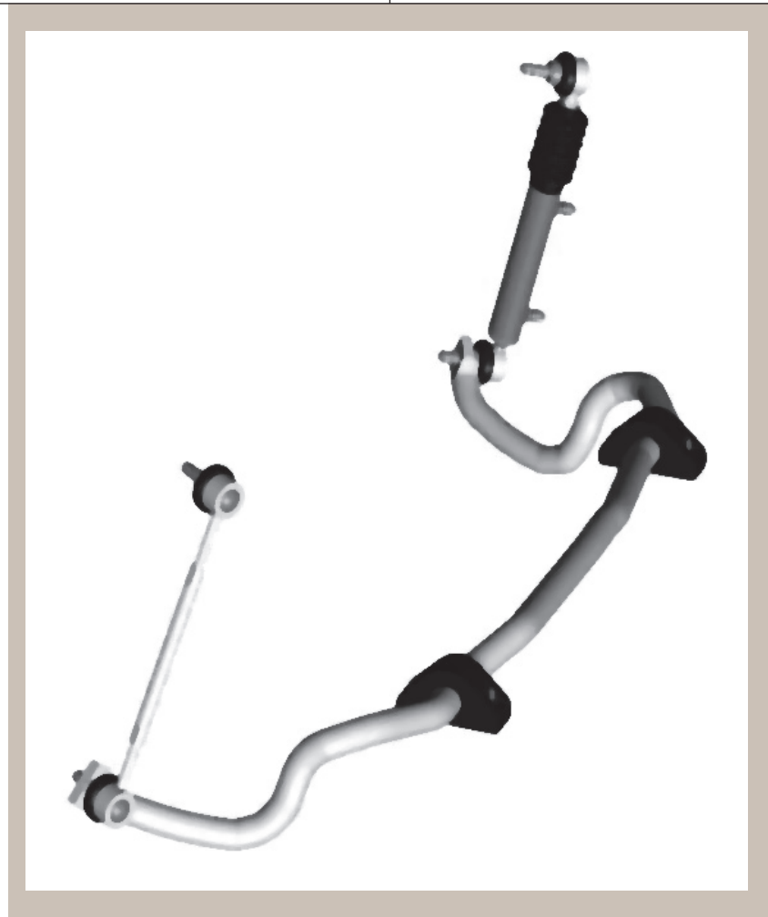
Figure 3. An active stabilizer bar includes a roll control actuator, a stabilizer bar, bushings and a rigid drop link.
