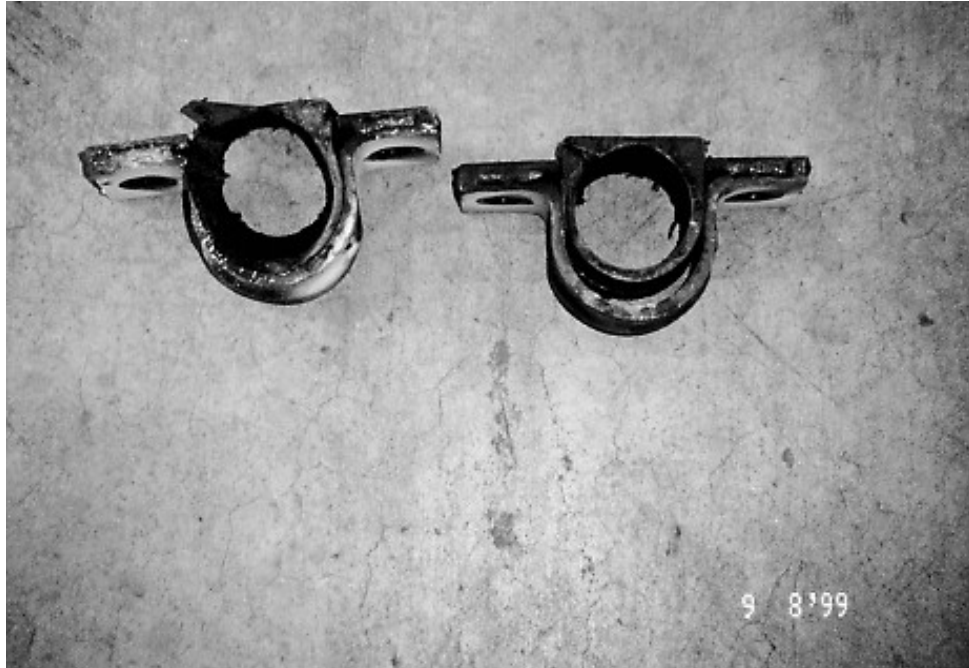
WORN FRONT STABILIZER BAR BUSHINGS (217 TEST MILES)
