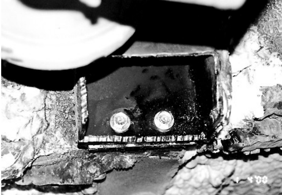
BROKEN BODY SUPPORT BETWEEN THE DRIVE AND TAG AXLES (2,167 TEST MILES)
