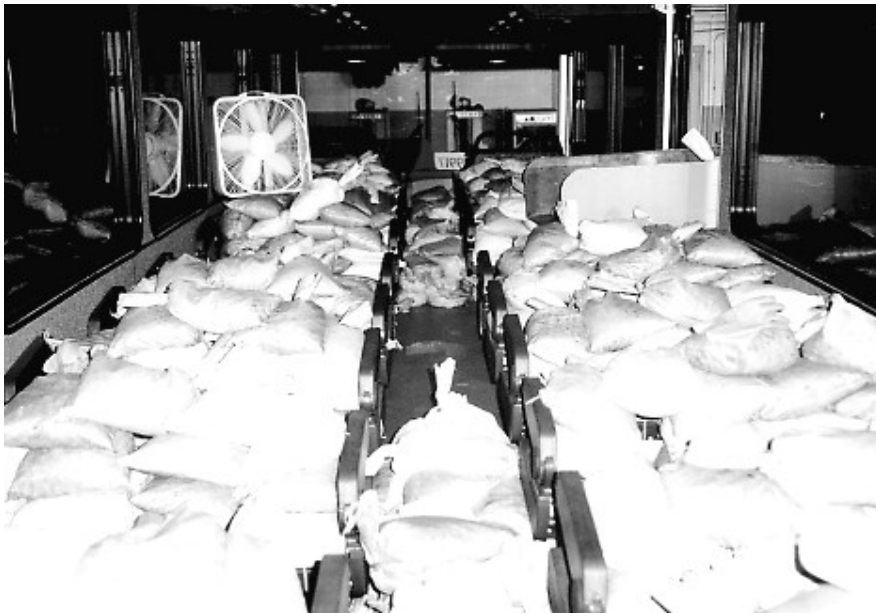
TEST BUS LOADED TO 2.5 TIMES GVL (25,500 LB)
