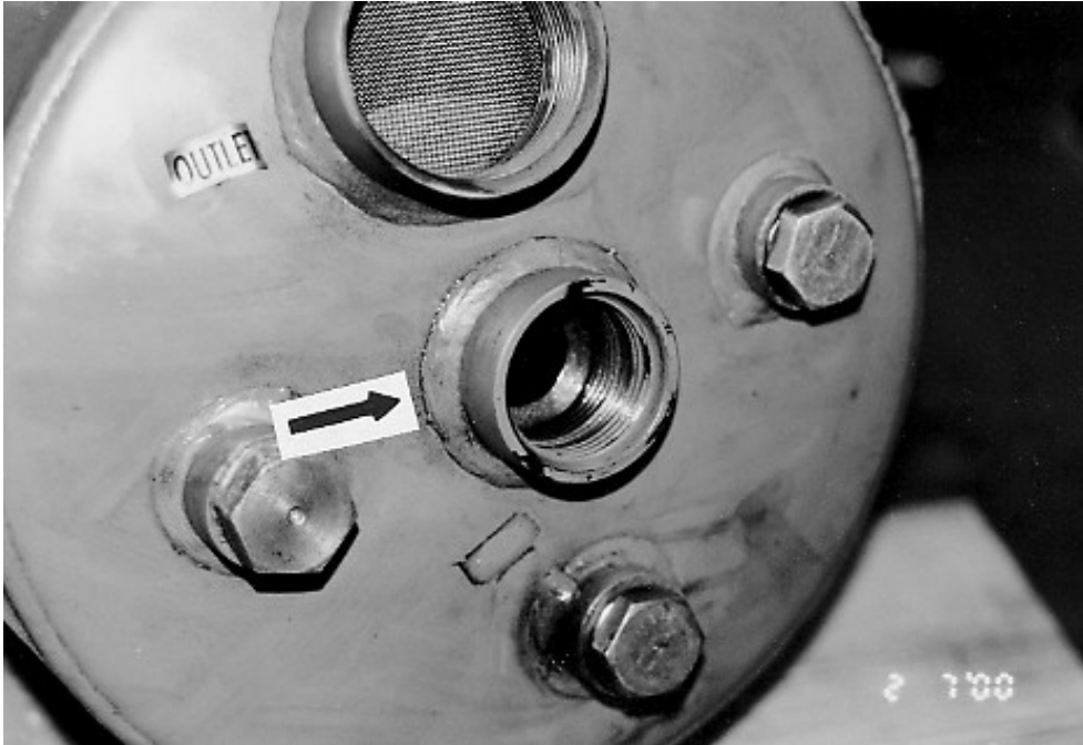
HYDRAULIC RESERVOIR IS LEAKING AT THE WELD ON THE CENTER FITTING
