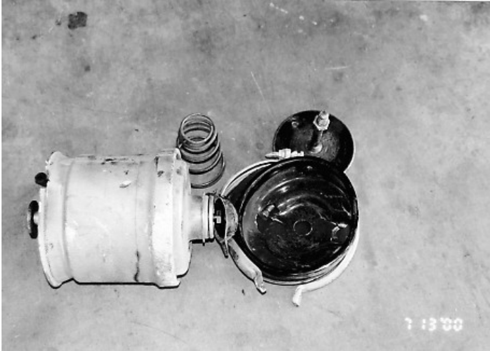
FAILED RIGHT SIDE BRAKE CHAMBER (14,305 TEST MILES)
