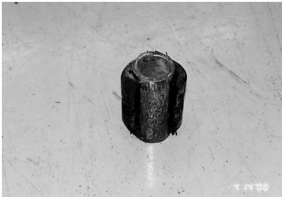
WORN CENTER BUSHING FROM THE LEFT TAG AXLE TRAILING ARM (10,937 TEST MILES)
