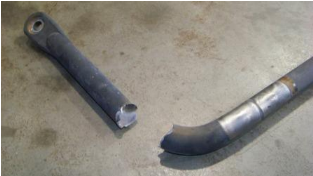
BROKEN RETAINING PLATE BOLT: LOWER, LEFT RADIUS ROD DRIVE AXLE (7,729 TEST MILES)
