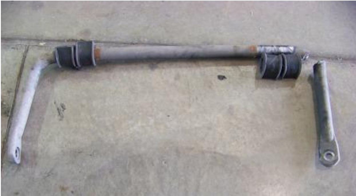
BROKEN FRONT SWAY BAR (5,848 TEST MILES)
