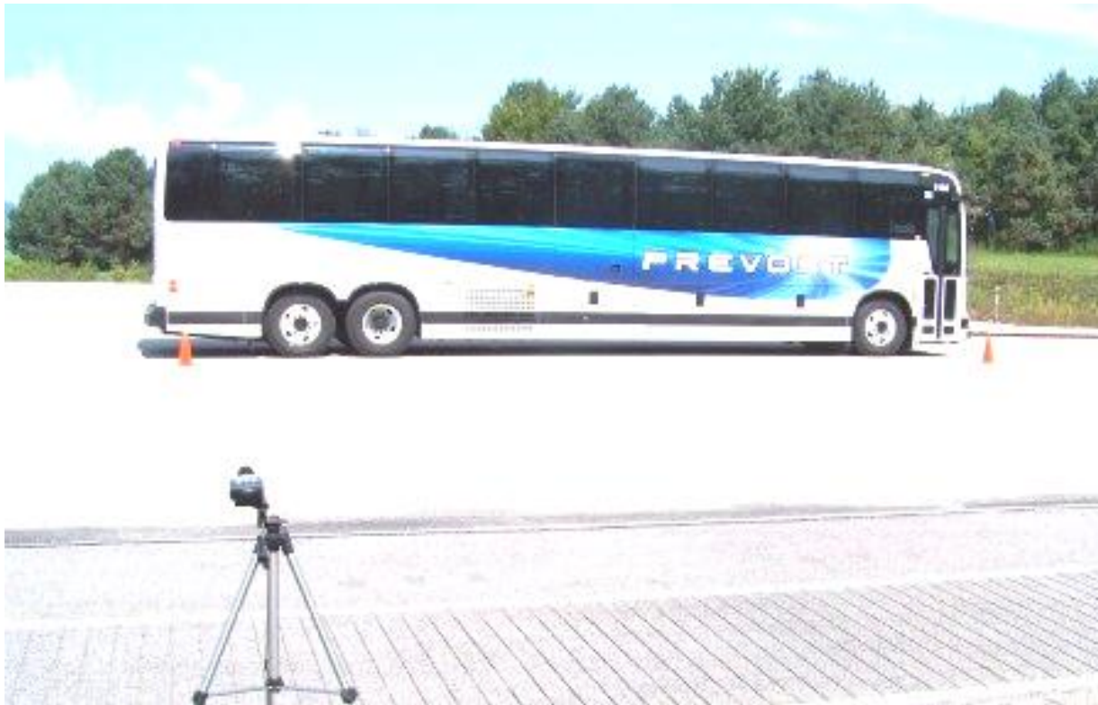
TEST BUS UNDERGOING EXTERIOR NOISE TEST
