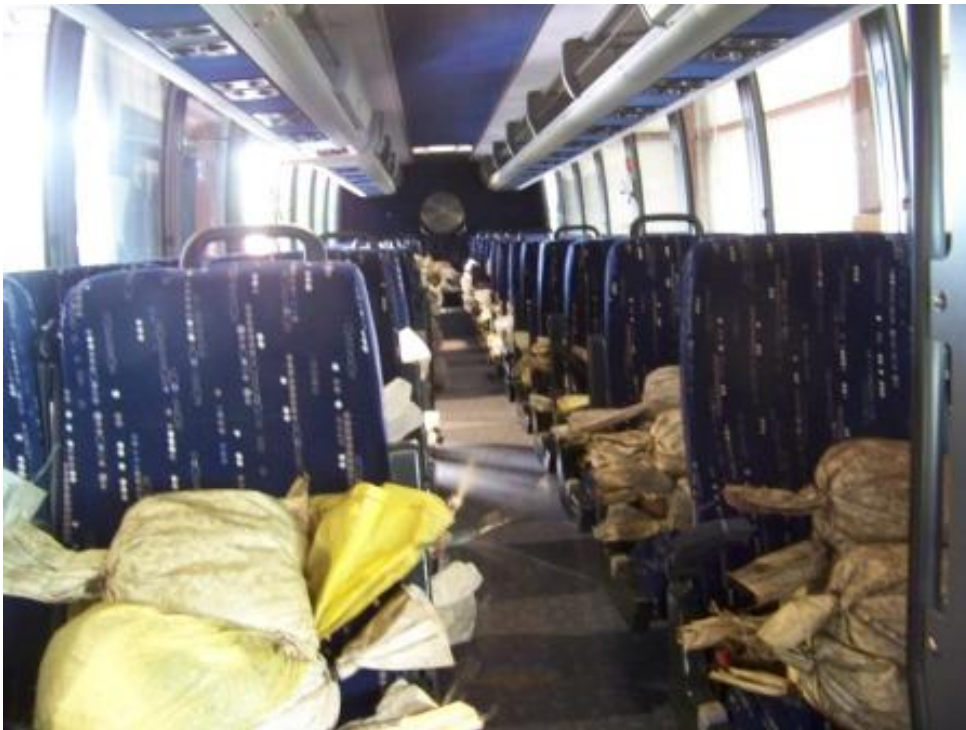
BUS LOADED TO 2.5 TIMES GVL (21,750 LBS)
