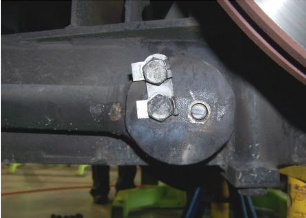
BOLT BROKEN; LEFT, REAR, LOWER RADIUS ROD RETAINING PLATE (6,324 TEST MILES)
