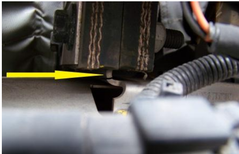
BROKEN FLEX EXHAUST PIPE (11,902 TEST MILES)
