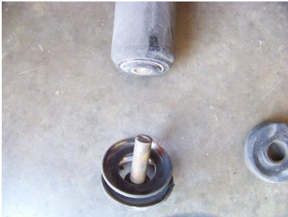
BROKEN LEFT FRONT SHOCK (10,913 TEST MILES)
