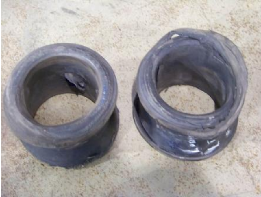
WORN UPPER & LOWER RADIUS ROD BUSHINGS; DRIVE AXLE (4,968 TEST MILES)
