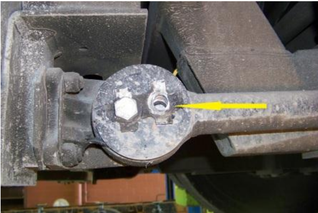
BROKEN RETAINING PLATE BOLT: LOWER, LEFT RADIUS ROD DRIVE AXLE (7,729 TEST MILES)
