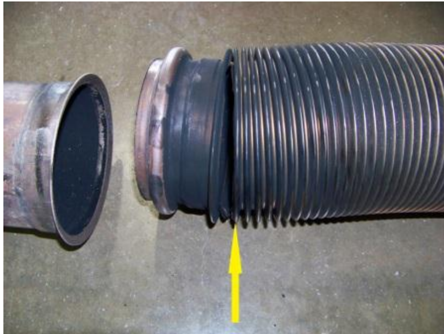
BROKEN FLEX EXHAUST PIPE (11,902 TEST MILES)
