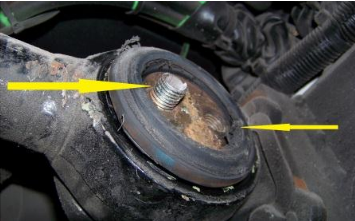
UPPER RADIUS ROD DRIVE AXLE; BROKEN RETAINING PLATE BOLTS (12,109 TEST MILES)
