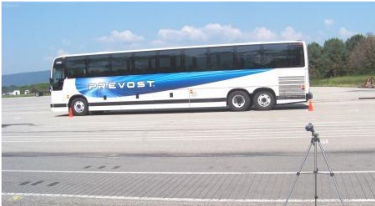
TEST BUS UNDERGOING EXTERIOR NOISE TEST
