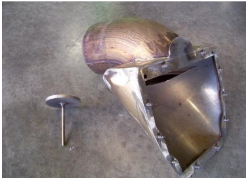
BROKEN COUNTERWEIGHT PIVOT ON EXHAUST DIFFUSER (11,902 TEST MILES)
