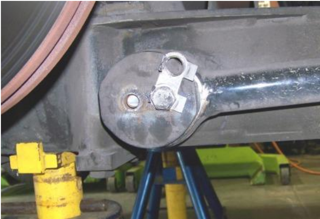
DRIVE AXLE; BROKEN LOWER RADIUS ROD RETAINING PLATE BOLTS (5,848 TEST MILES)
