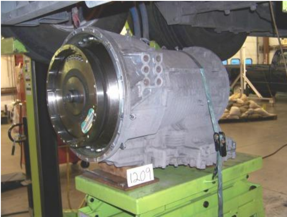
TRANSMISSION REMOVAL AND REPLACEMENT (8.50 MAN HOURS)
