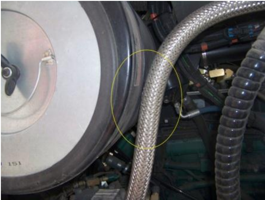
A/C LINE RUBBING ON AIR CLEANER CANNISTER (4,968 TEST MILES)
