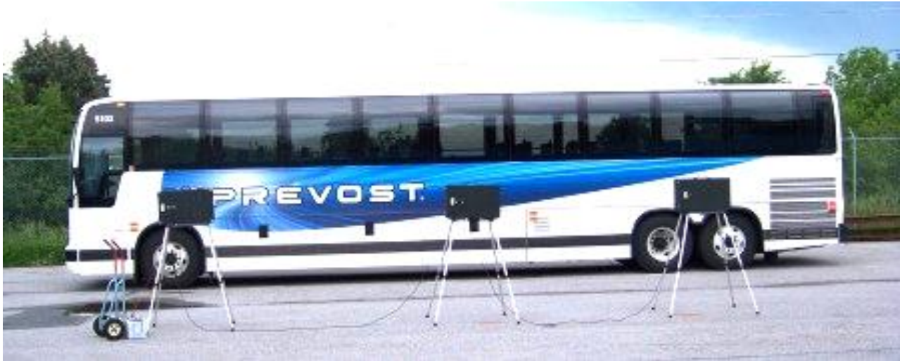
TEST BUS SET-UP FOR 80 dB(A) INTERIOR NOISE TEST
