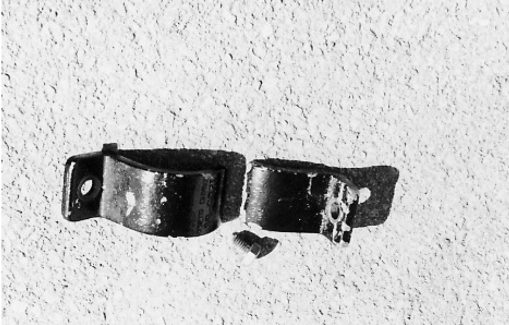
BROKEN RIGHT, OUTSIDE SWAY BAR BRACKET (213 TEST MILES)
