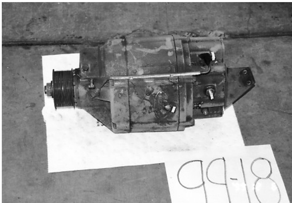
GENERATOR REMOVAL AND REPLACEMENT (1.5 MAN HOURS)
