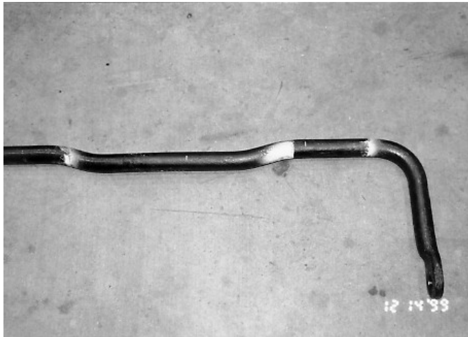
CRACKED TAG AXLE SWAY BAR (4,181 TEST MILES)
