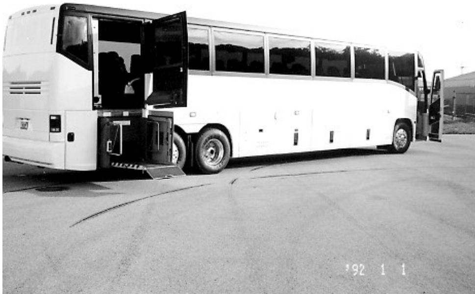
MOTOR COACH INDUSTRIES MODEL RENAISSANCE EQUIPPED WITH A STEWART AND STEVENSON MODEL SS BL 3761 HANDICAP DEVICE
