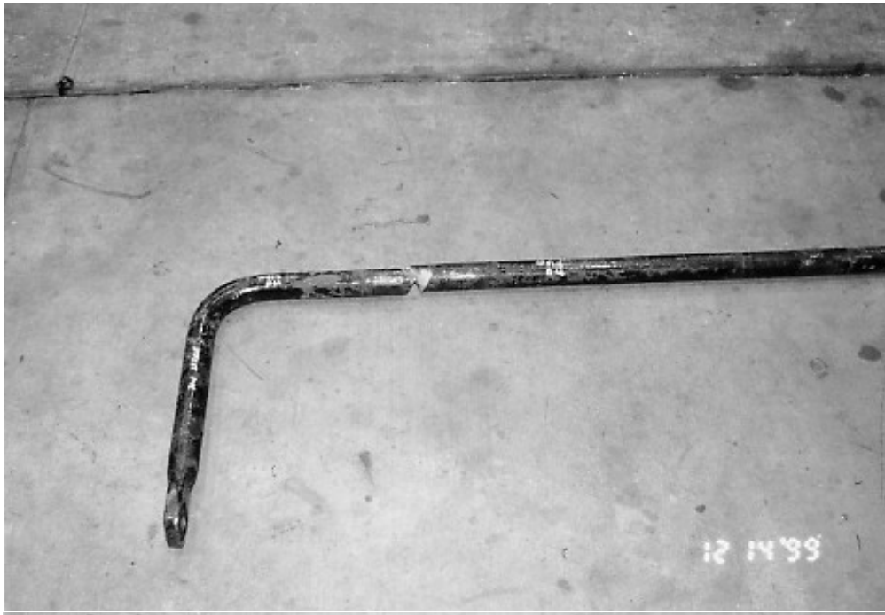
BROKEN FRONT SWAY BAR (4,181 TEST MILES)
