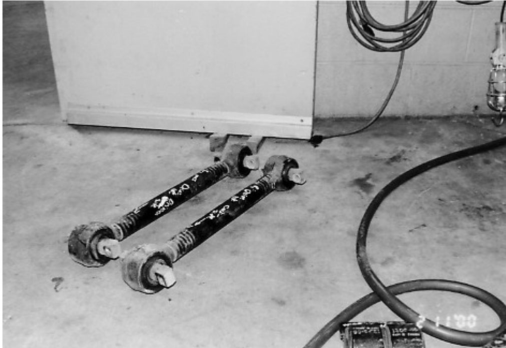
DRIVE AXLE RADIUS ROD BUSHINGS ARE WORN (10,100 TEST MILES) CHAFFED LEFT FRONT AIR BAG
