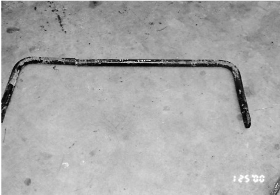
BROKEN FRONT SWAY BAR (8,116 TEST MILES)
