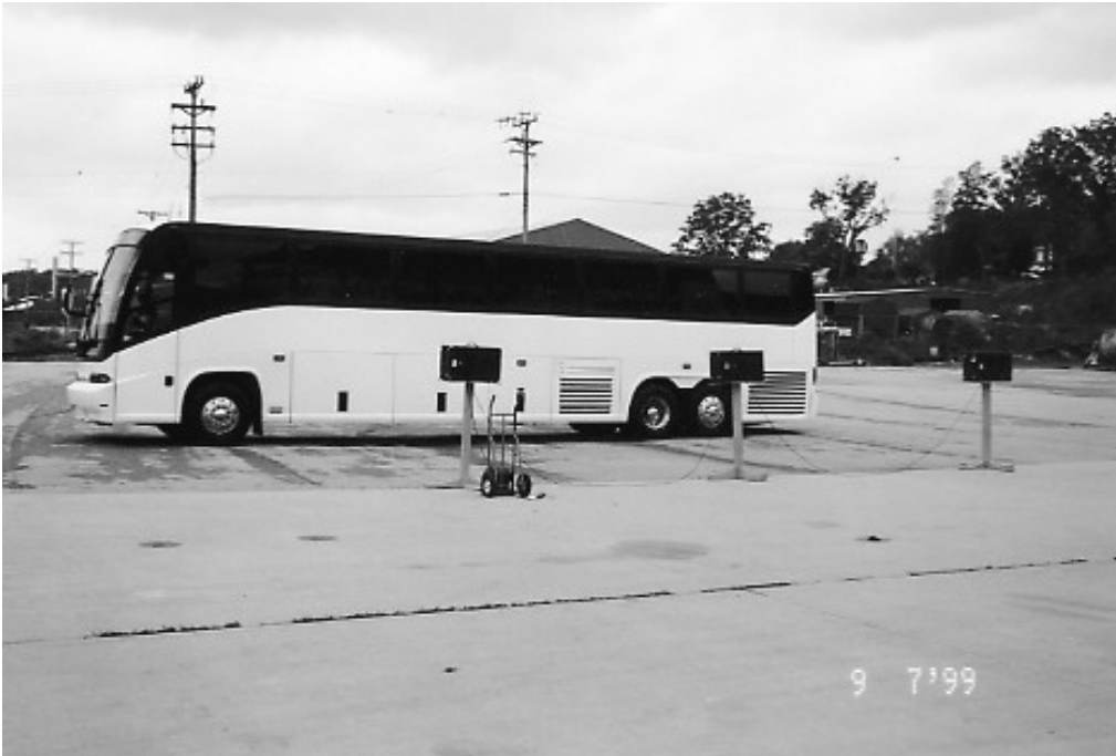
TEST BUS SET-UP FOR 80 dB(A) NOISE TEST
