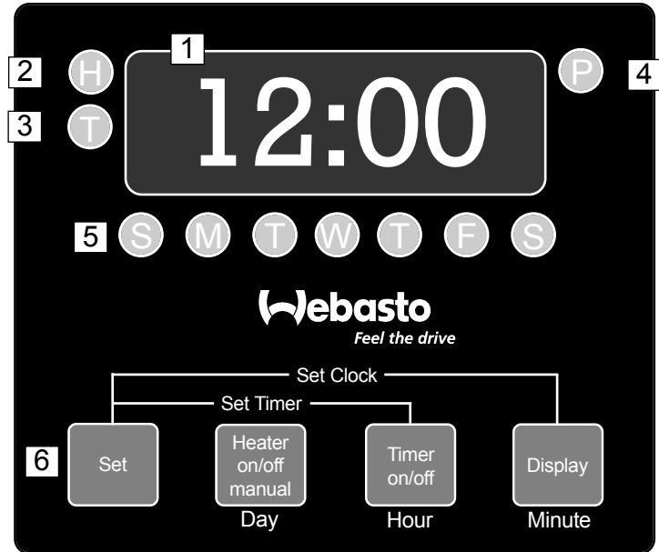
Fig. 5: 7-Day Electronic Timer Model CDN-1224
