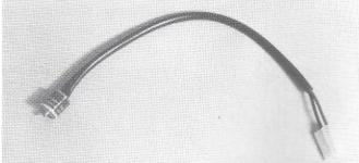
**Description:** The pre-heat thermostat is installed in the burner on the back wall (2010) or on the disc (2020, 300, 350). It switches the heating element (24) which warms up the fuel in the nozzle holder.
