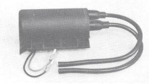
**Description:** Within the electronic ignition unit, a high voltage of approx. 8000 volt is generated and brought to the two ignition electrodes. The electronic ignition unit is only in operation during the starting phase.
