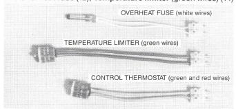
**Description:** The overheat fuse protects the heater against too high and inadmissable temperatures. The overheat fuse contains a fusible link reacting when the admissable temperature is exceeded (138° C [280° F]), and switches the heater off with a purge cycle.
