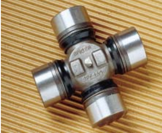
Photo 5, Permanently Lubricated Plug Style
