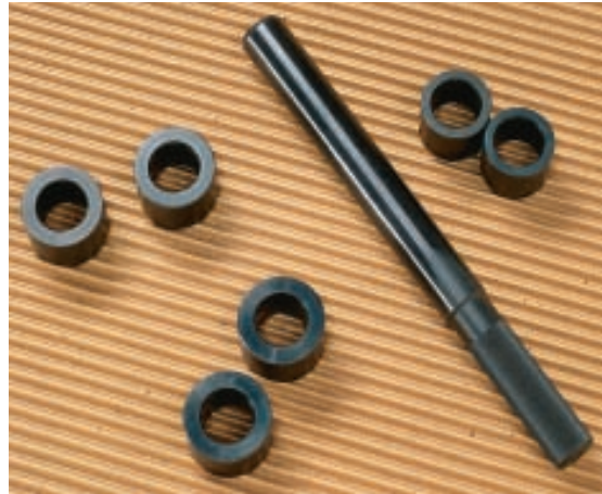
Photo 81, Spicer Alignment Bar Kit, Quick Disconnect Style
