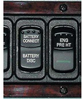
The house and engine batteries are charged from either the alternator or the inverter battery charger. The auxiliary battery switch is in the ON position in order for the inverter battery charger to operate, either the generator must be running or the motor home must be connected to a shoreline supply.
