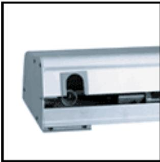
A hand crank is supplied with every awning and easily telescopes from 50 to 82 inches. Simply insert the end of the crank into the receiver, which is located at either the right or left side of the awning. Push up and rotate the handle one-quarter turn clockwise, then let the handle drop about a half-inch. You should then feel the handle lodge in the receiver. You are now ready to extend the awning.
