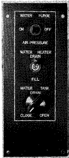
Figure 5-2. Water Purge Air Pressure, Water Heater Drain and Water Tank Drain Controls
