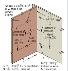
Note: These holes and dimensions are used only if adjustability through the use of slotted holes in catch is desired.
