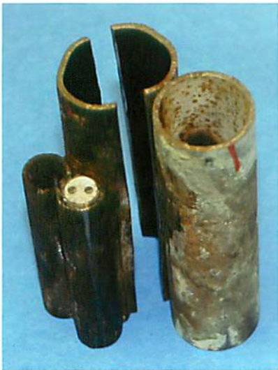
FIGURE 8 —Upper portion of a boiler which has been sectioned axially to view inner surfaces.
