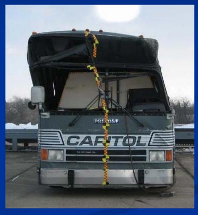
■ Both buses the front residual space template struck the side window in the front
