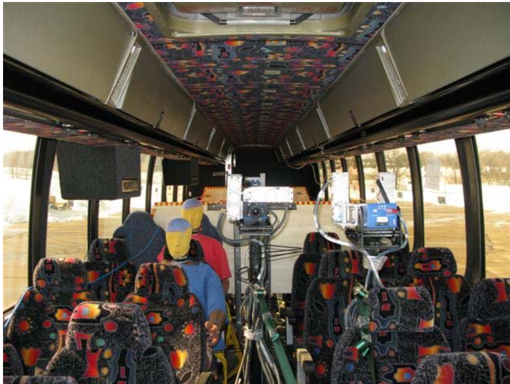
Figure 36: Prevost pretest ATD placement
