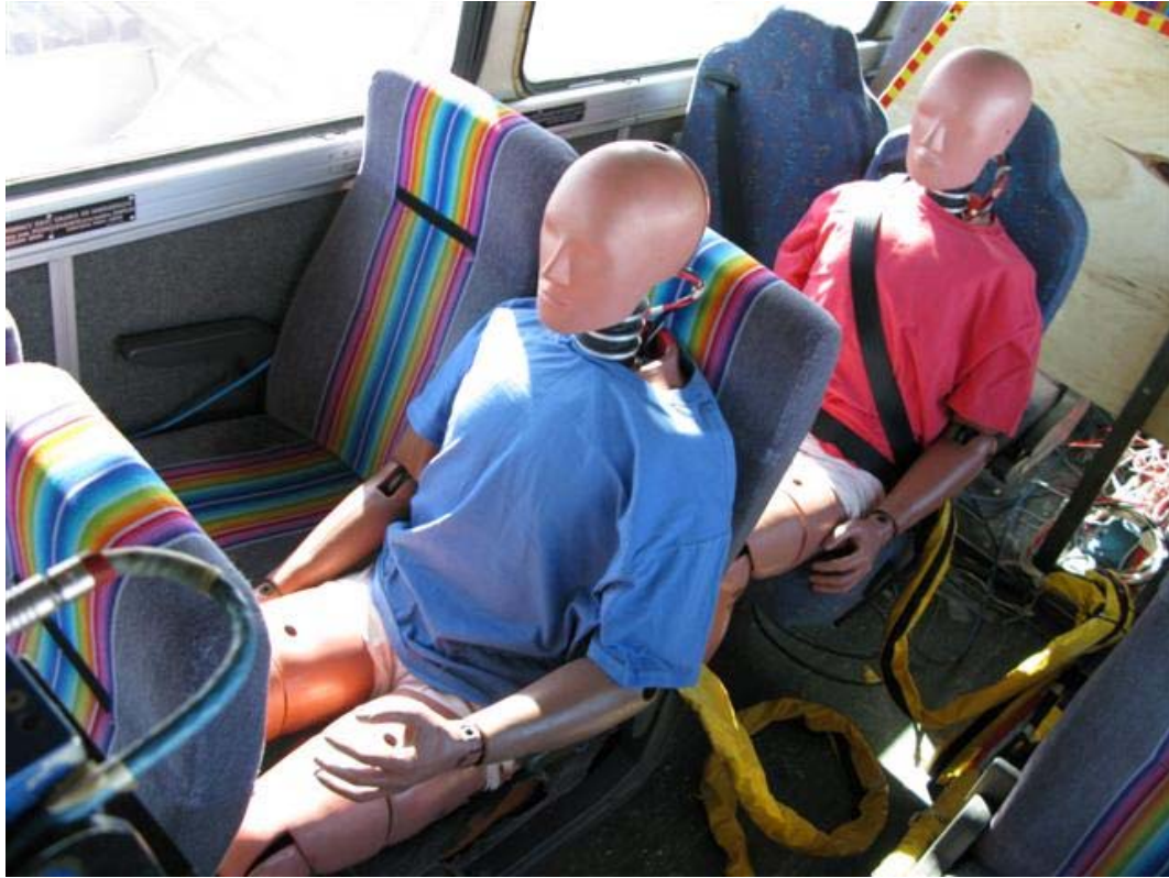
Figure 24: MCI pretest ATD placement
