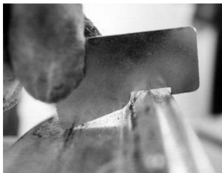
Photo 1. Acceptable Rim Flange Wear Condition
