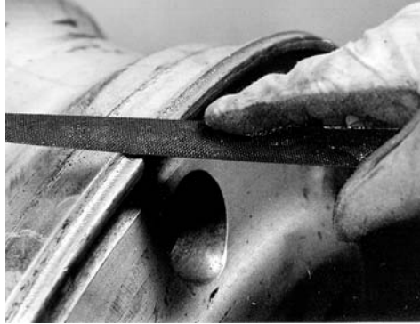
Photo 4. Removing sharp edge by hand with a metal file.
