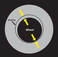
2. Measure and record the radial runout on the vehicle of each assembly with tire runout gauge. Mark the highest point of the assembly. Rotate each assembly until the high spot is at the 12:00 position (without allowing the assembly to turn). Loosen all lug nuts and re-torque in the proper sequence. Re-measure and record the radial runout of the assembly.
