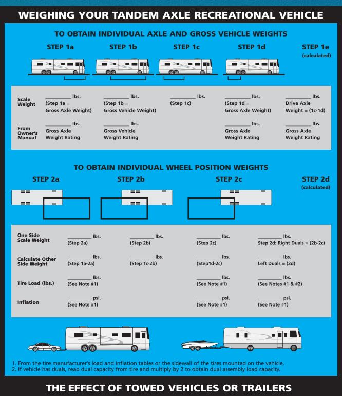
If you are towing a vehicle, you need to know your RV's G.C.W.R. (Gross Combined Weight Rating), the total actual loaded weight of your RV, plus the total actual loaded weight of the towed vehicle. Even though the G.C.W.R. has more to do with the design limits of the drivetrain (engine, transmission, axle, brakes and bearings), the additional weight can also affect the tires and your RV's handling. Also, always remember to consider the tongue weight of the trailer and its effect on handling.
