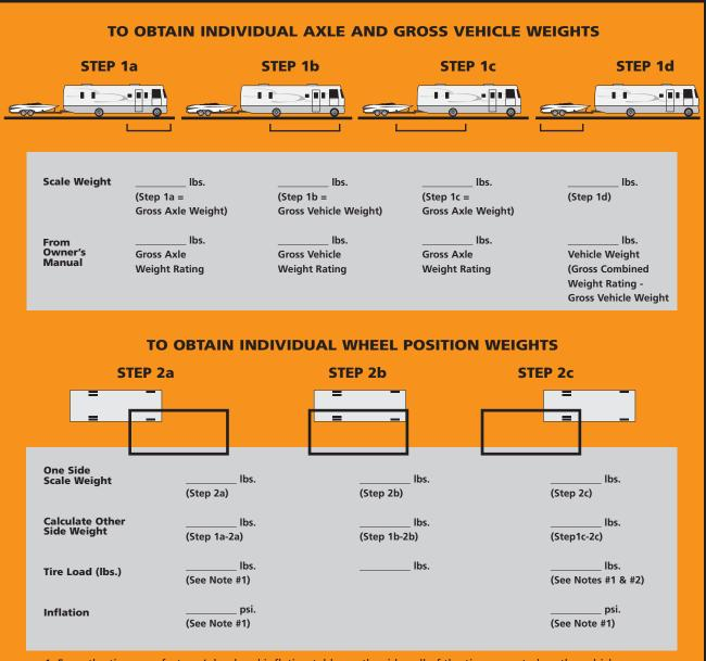
1. From the tire manufacturer's load and inflation tables or the sidewall of the tires mounted on the vehicle. 2. If vehicle has duals, read dual capacity from tire and multiply by 2 to obtain dual assembly load capacity.
