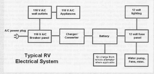
See.. there's really nothing to it! In the simplest terms, you have lights and other equipment such as water pump, fans, stereo, etc. that run on 12 volts, a battery that supplies the 12 volt power and
