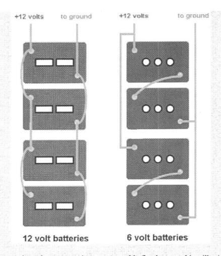
When replacing your batteries, remove the **negative** cable first because this will minimize the possibility of shorting the battery when you remove the other cable. Next remove the **positive** cable and then the hold-down bracket or clamp. If the hold down bracket is severely corroded, replace it. Dispose the old battery by exchanging it when you buy your new one or by taking it to a recycling center. Please remember that batteries contain large amounts of harmful lead and acid.
