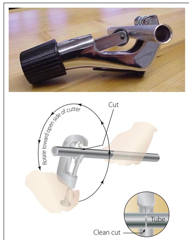
**Figure 7-2. Tube cutting.**
