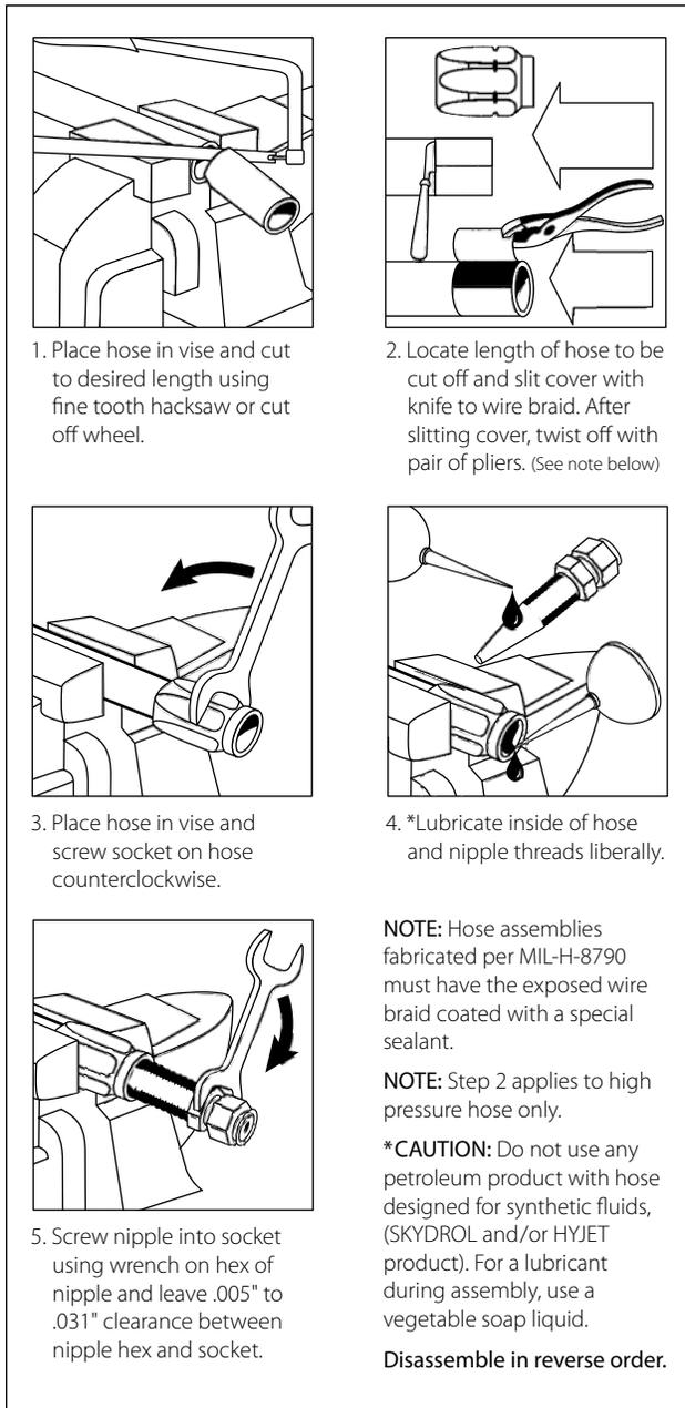
**Figure 7-28. Assembly of MS fitting to flexible hose.**
