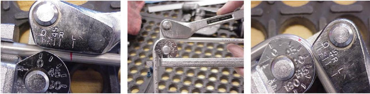
**Figure 7-4. Tube bending.**
