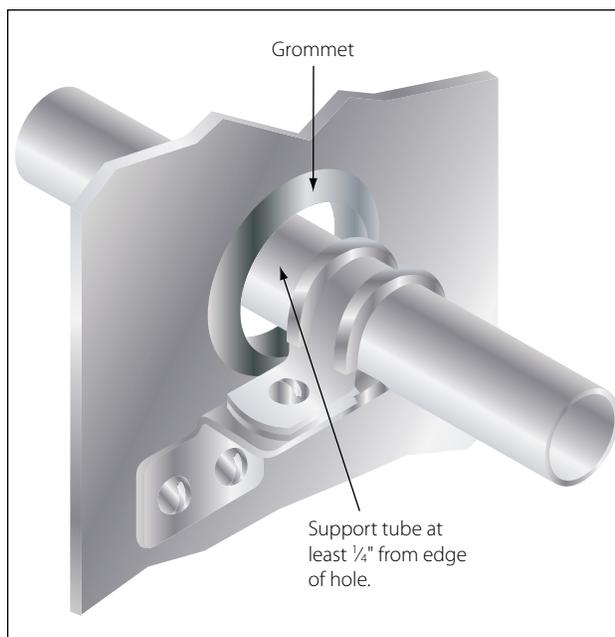
**Figure 7-32. Rubber-cushioned clamp.**
