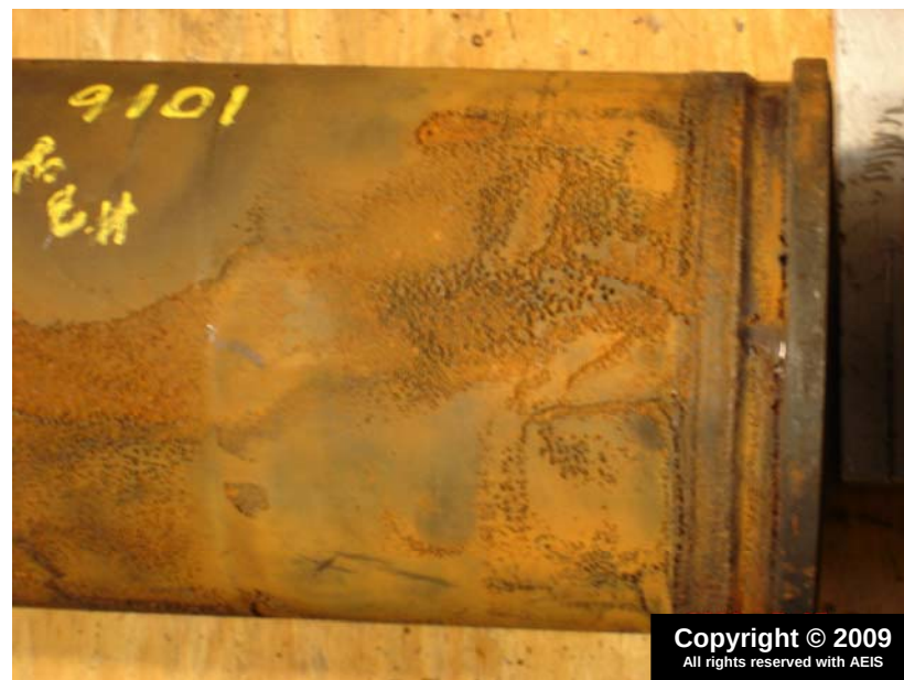
Figure 4: Cavitation patches on cylinder liner 1016
