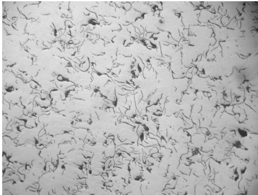
Figure 14: New Liner microstructure near the flange in as polished condition 100X Magnification
