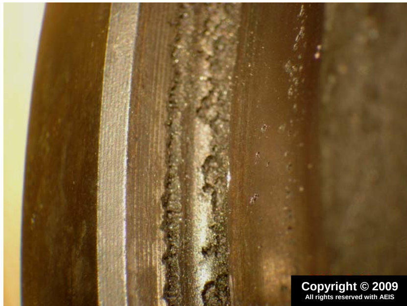
Figure 9: Cavitations immediately under the flange
