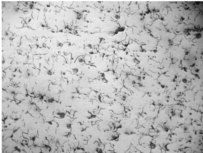
Figure 19: Liner 1016 Microstructure in the middle of the fire length in as polished condition. 100X Magnification
