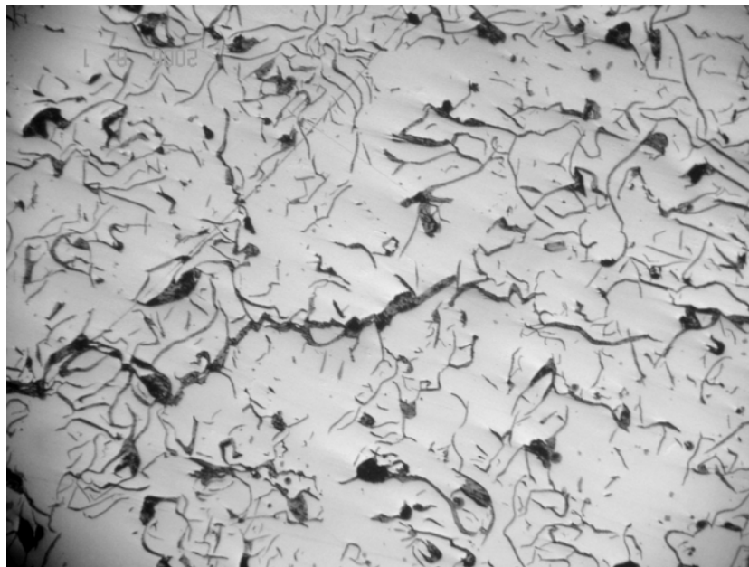
Figure 27: The crack propagation in liner 277 along the graphite flakes. 200X Magnification
