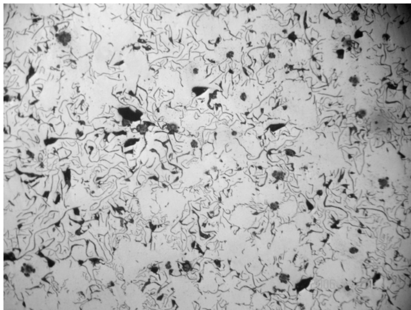
Figure 17: Liner 277 microstructure near the flange in as polished condition. 100X Magnification
