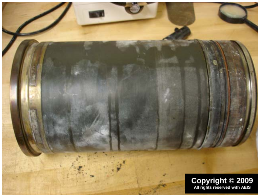
Figure 6: Outside surface of cylinder liner 1076 generally free of cavitations.
