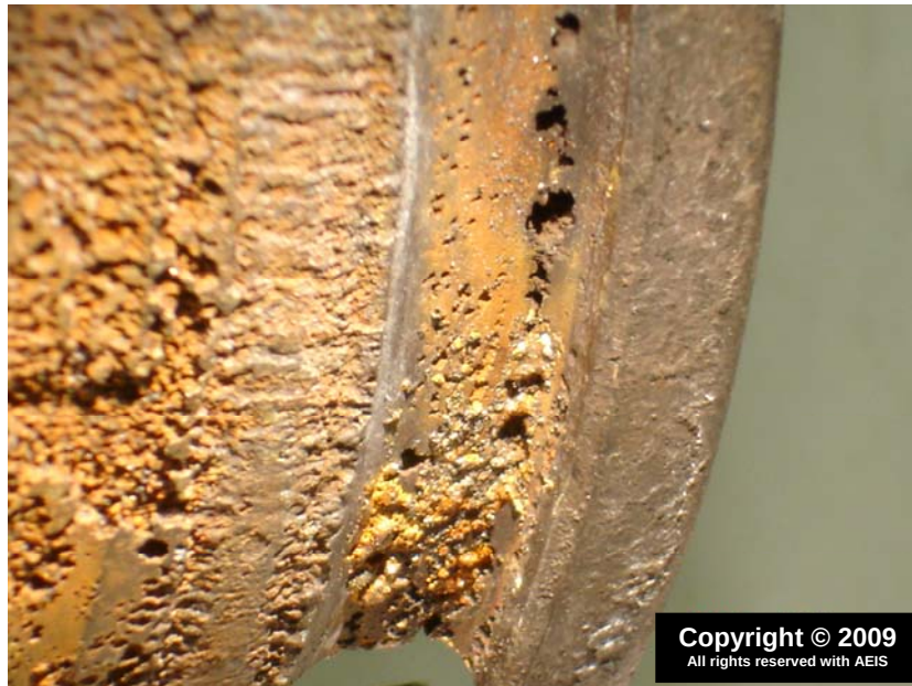
Figure 5: Close up of cavitation damage under the flange on cylinder liner 1016
