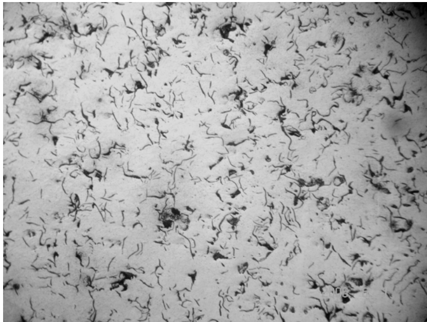
Figure 20: Liner 1016 Microstructure near the flange in as polished condition. 100X Magnification
