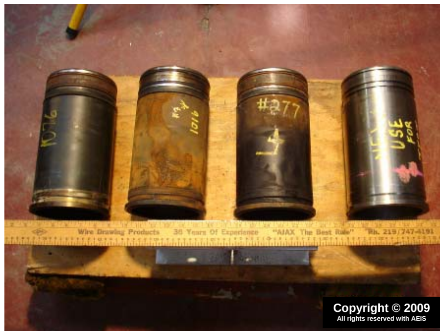
Figure 1: Cylinder liners in as received condition
