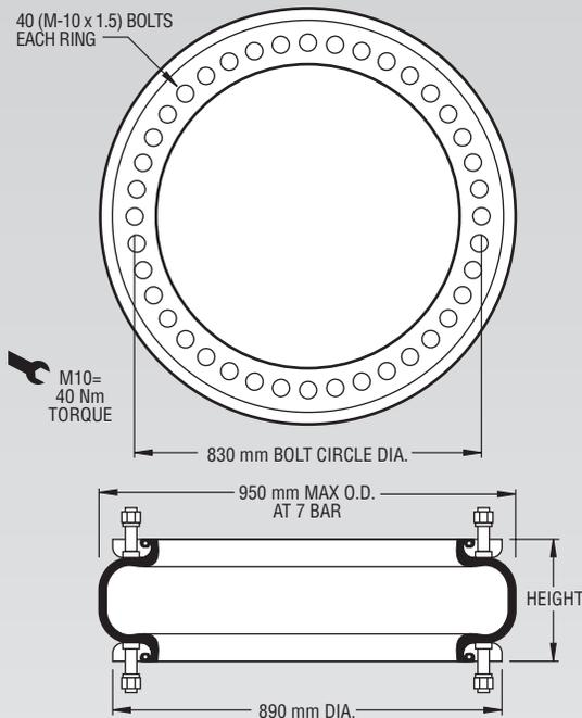
**NOTE: The effective length of the 45 mm bolt is 23 mm in this bead ring.**
