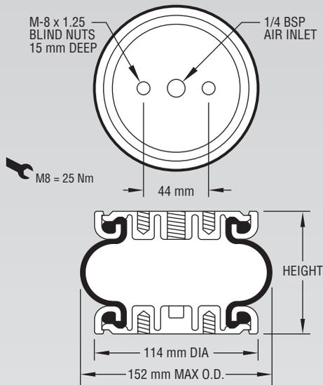
**NOTE:** The bellows extends beyond the bead plates at minimum height.
