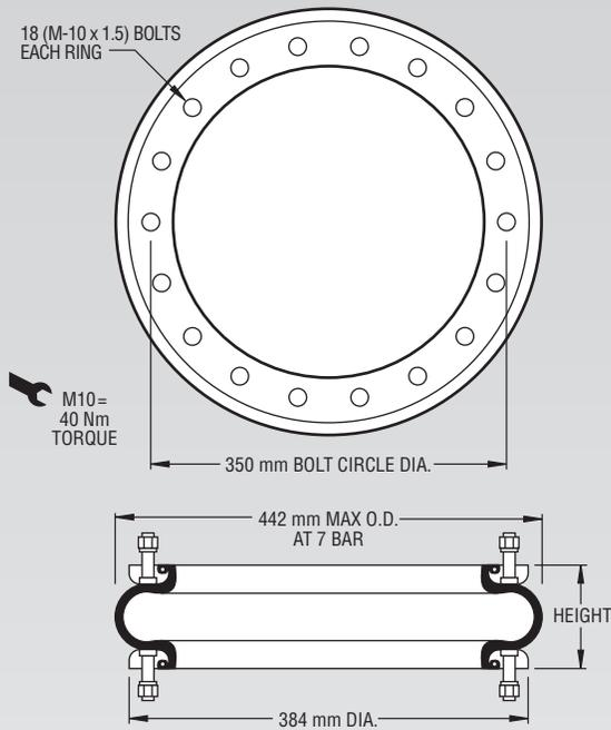
**NOTE: A bead plate part is shown. This part is also available with rolled plates. See page 11 for explanation.**
