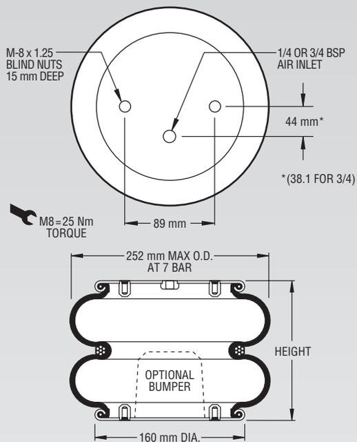
**NOTE: A bead plate part is shown. This part is also available with bead rings. See pages 8-10 for explanation.**
