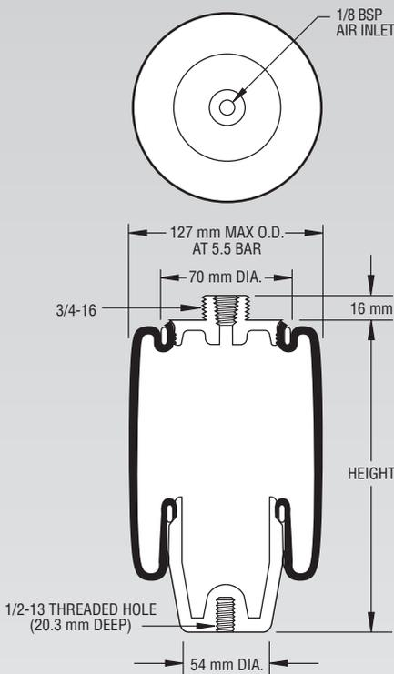
**NOTE: Bellows will not compress properly with less than .7 BAR internal pressure.**
