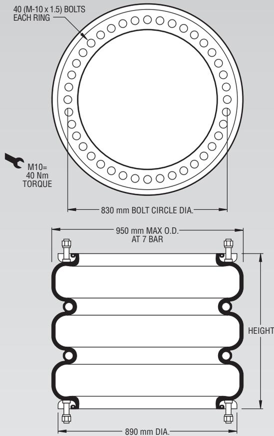
**NOTE: The effective length of the 45 mm bolt is 23 mm in this bead ring.**
