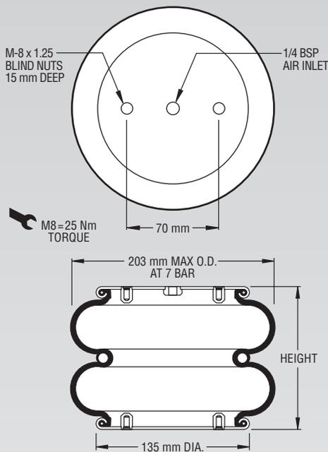
**NOTE: A bead plate part is shown. This part is also available with bead rings. See pages 8-10 for explanation.**
