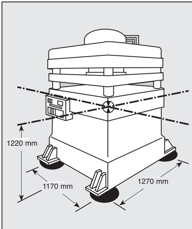
In the above example, the most narrow distance between two Airmount isolators is 1170 mm. The height to the c.g. is 1220 mm; therefore, this system does not meet our guideline. Two possible solutions would be:
