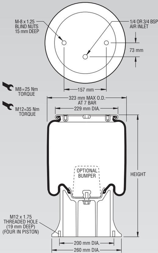
**NOTE: Bellows will not compress properly with less than .7 BAR internal pressure.**
