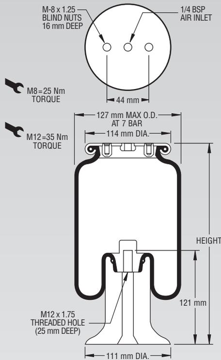
**NOTE: Bellows will not compress properly with less than .7 BAR internal pressure.**
