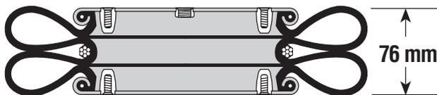
The bellows can be damaged if allowed to constantly bottom-out as shown above; therefore, a downstop is required to prevent this. An external downstop can be something as simple as a steel block and should be sized
