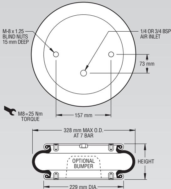
**NOTE: A bead plate part is shown. This part is also available with bead rings. See pages 8-10 for explanation.**
