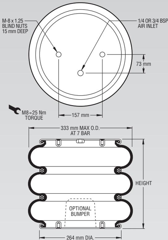
**NOTE: A bead plate part is shown. This part is also available with bead rings. See pages 8-10 for explanation.**
