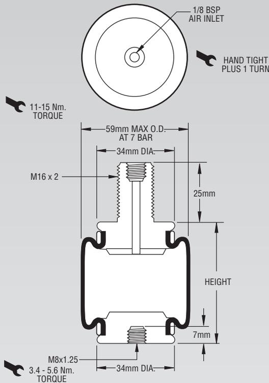
**NOTE:** This Airstroke actuator must be guided throughout the stroke.
