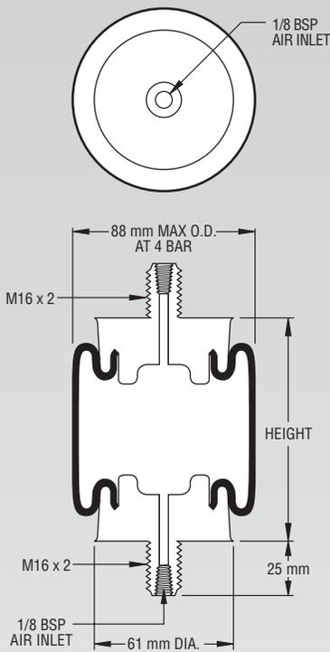
**NOTE:** This Airstroke actuator must be guided throughout the stroke.
