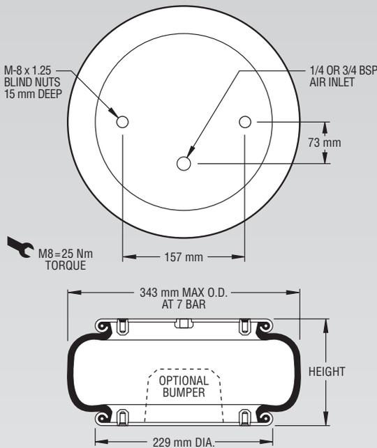
**NOTE: A bead plate part is shown. This part is also available with bead rings. See pages 8-10 for explanation.**
