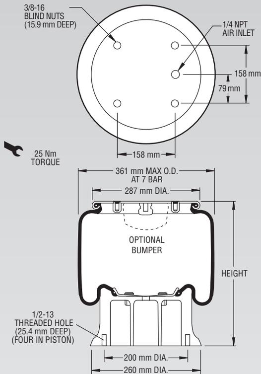
**NOTE: Bellows will not compress properly with less than .7 BAR internal pressure.**
