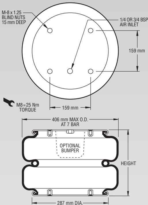
**NOTE: The bellows extends beyond the bead plates at minimum height.**
