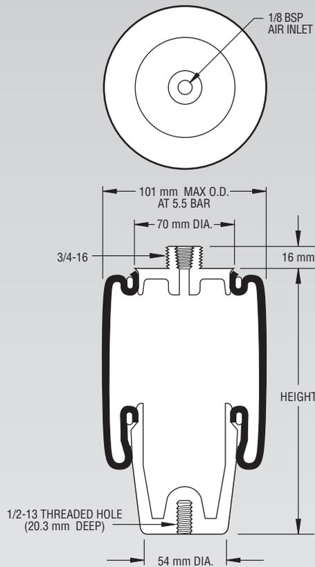
**NOTE: Bellows will not compress properly with less than .7 BAR internal pressure.**
