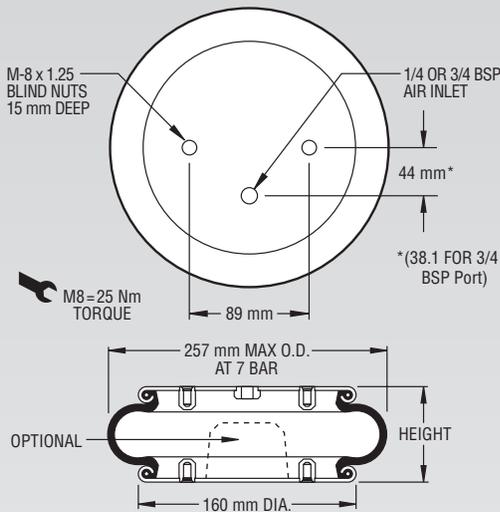
**NOTE: A bead plate part is shown. This part is also available with bead rings. See pages 8-10 for explanation.**
