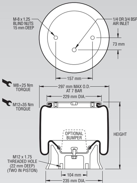
**NOTE: Bellows will not compress properly with less than .7 BAR internal pressure.**
