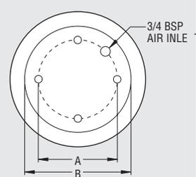
Note: Threads conform to ISO 228-1; gauge to ISO 228-2.
