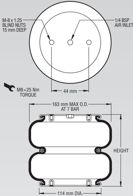
**NOTE: A bead plate part is shown. This part is also available with bead rings. Bolts are not included. See pages 8-10 for explanation.**
