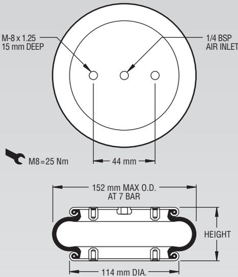
**NOTE: A bead plate part is shown. This part is also available with bead rings. Bolts are not included. See pages 8-10 for explanation.**
