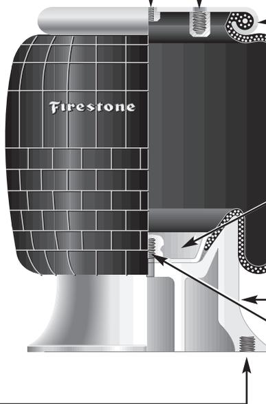
**AIR INLET** 1/4 BSP parallel is standard. 3/4 BSP parallel is also available for most parts. (See the data sheet order block on each specific part).
