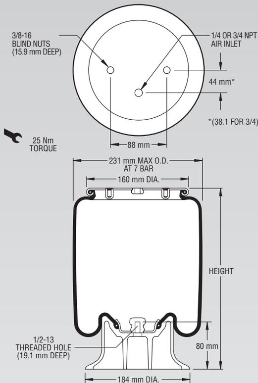
**NOTE: Bellows will not compress properly with less than .7 BAR internal pressure.**
