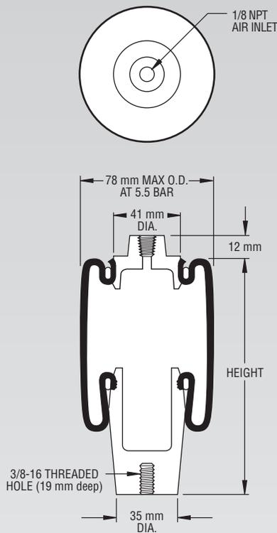
**NOTE: Bellows will not compress properly with less than .7 BAR internal pressure.**
