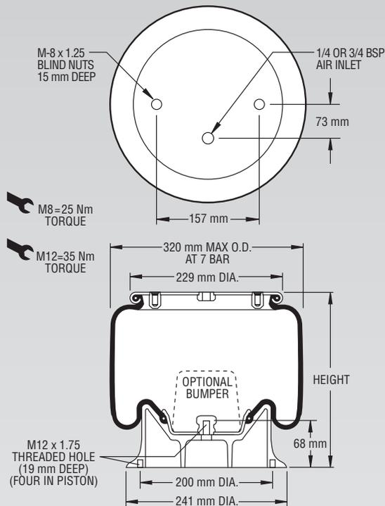
**NOTE: Bellows will not compress properly with less than .7 BAR internal pressure.**
