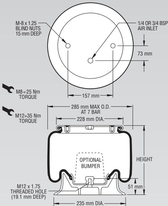
**NOTE: Bellows will not compress properly with less than .7 BAR internal pressure.**
