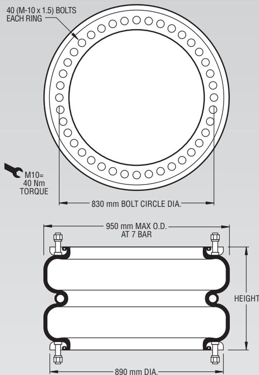
**NOTE: The effective length of the 45 mm bolt is 30 mm in this bead ring.**
