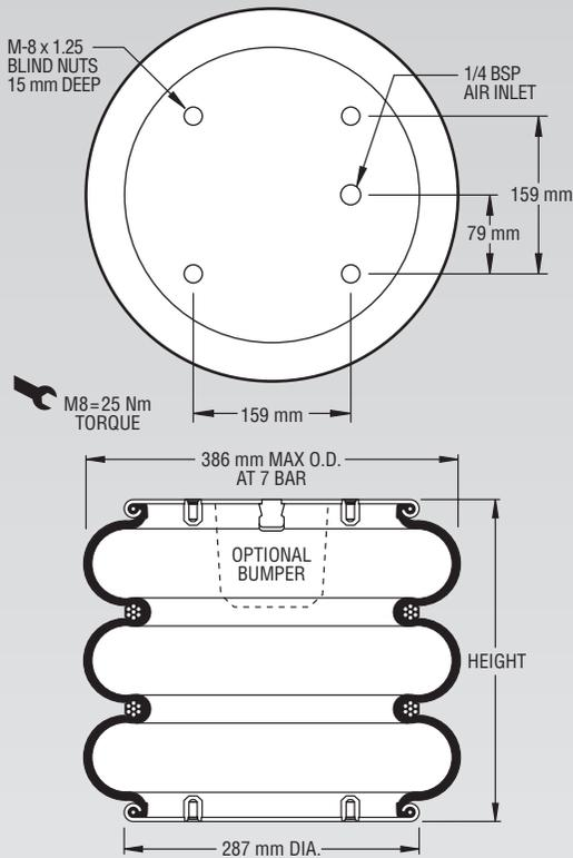
**NOTE: A bead plate part is shown. This part is also available with bead rings. See pages 8-10 for explanation.**
