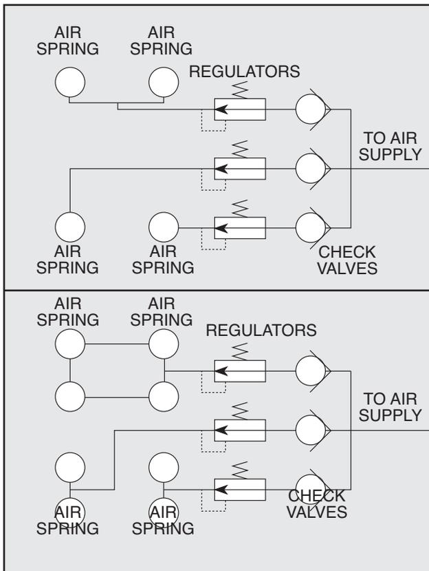
This eliminates the need for periodic inspections. The air springs should always be connected in clusters so the mass is supported with only THREE REGULATORS. This is illustrated below (in the previous column) for both a four and eight Airmount system:
