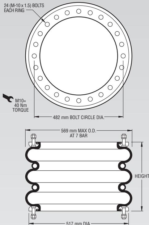
**NOTE: A bead ring part is shown. This part is also available with rolled plates. See page 11 for explanation.**
