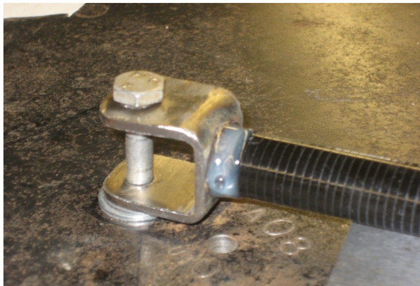
Figure 18: Bond between Steel joint and Carbon Fiber Tube
