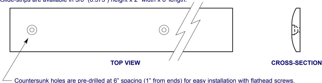
Countersunk holes are pre-drilled at 6" spacing (1" from ends) for easy installation with flathead screws.
