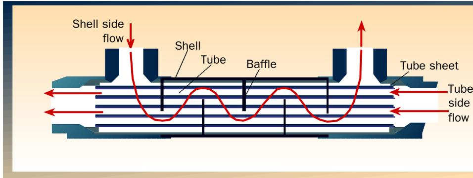
**Figure 5. Shell-and-tube heat exchanger with counter-current flow.**
