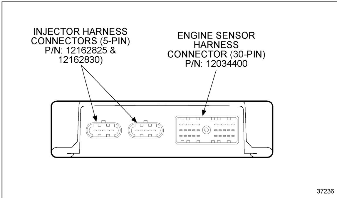
**Figure 3-35 ECM Left Side, Engine Harness Connections**
