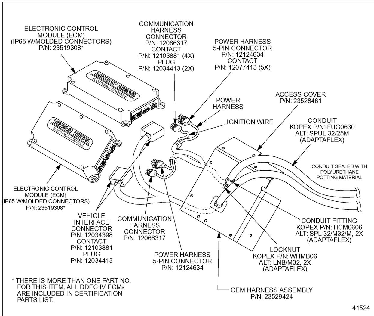
**Figure 3-127 Series 2000 Equipment Side Connectors and Cables**
