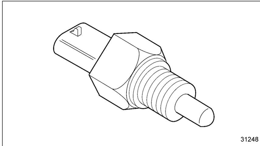
**Figure 3-69 Air Temperature Sensor**
