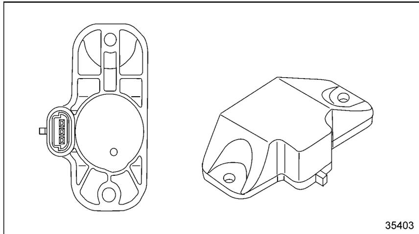
**Figure 3-92 The Turbo Boost Sensor - On-highway Applications**
