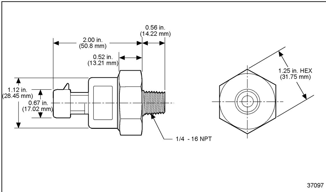
**Figure 3-109 The Fire Truck Pump Pressure Sensor**
