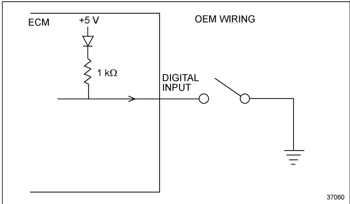
**Figure 3-14 DDEC IV Digital Input Circuit**
