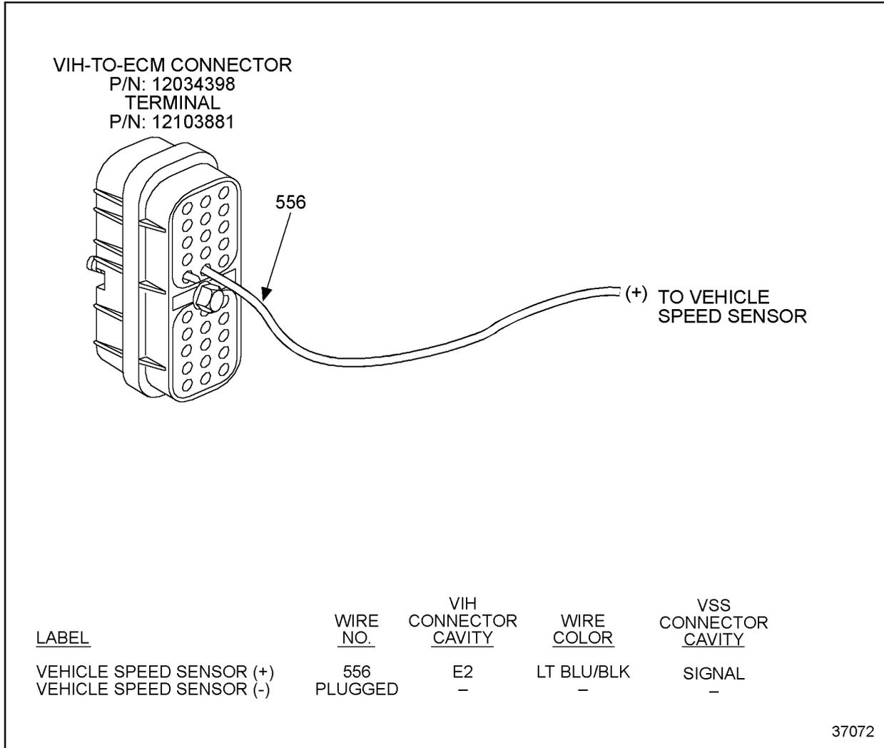
**Figure 3-113 Open Collector Vehicle Speed Sensor Installation**
