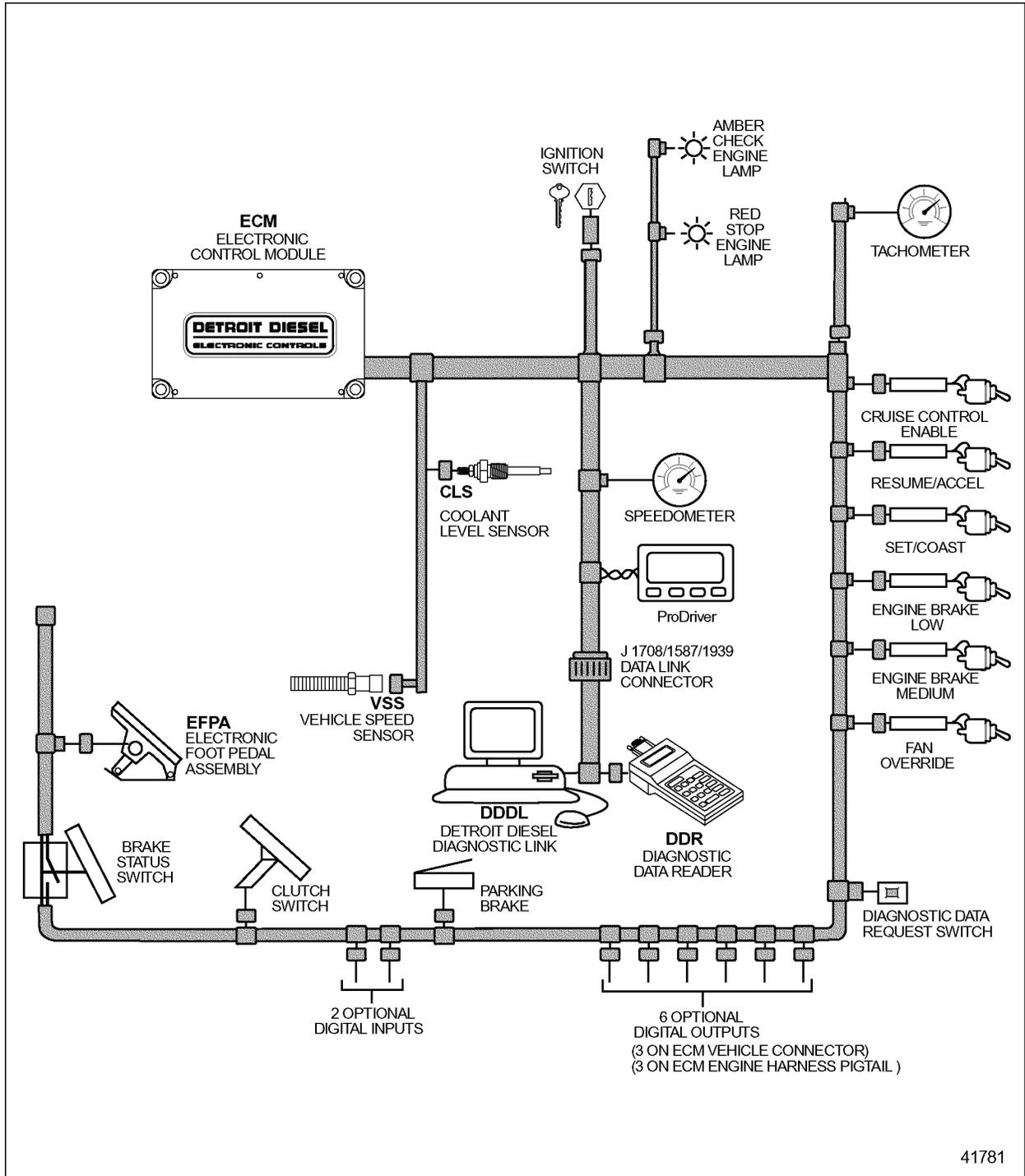
Figure 3-8 Typical On-highway Vehicle Interface Harness
