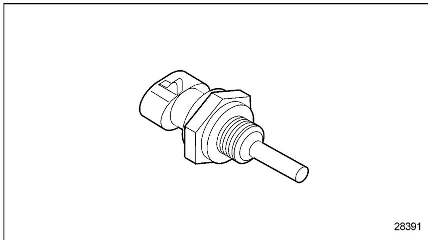
**Figure 3-81 Fuel Temperature Sensor - Series 2000**
