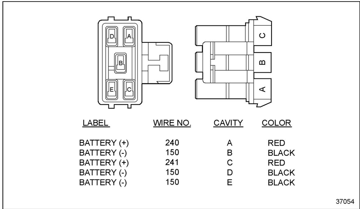
**Figure 3-33 Five-Pin Power Harness Connector**
