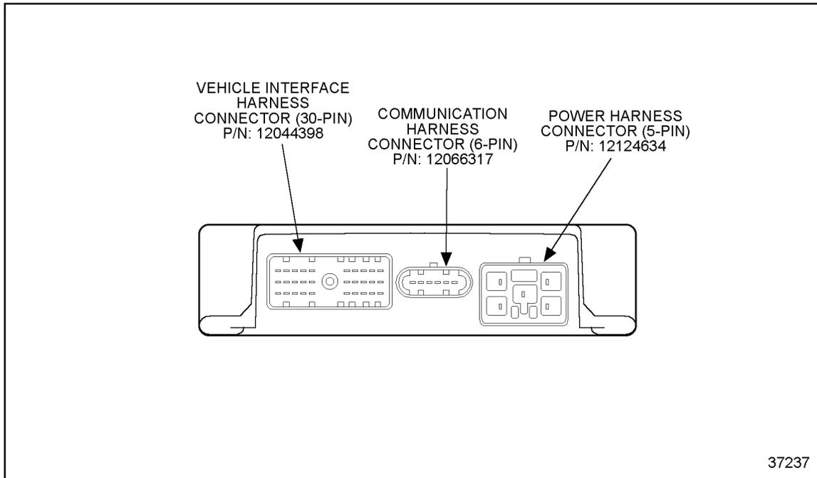
**Figure 3-31 ECM Right Side, Vehicle Harness Connections**
