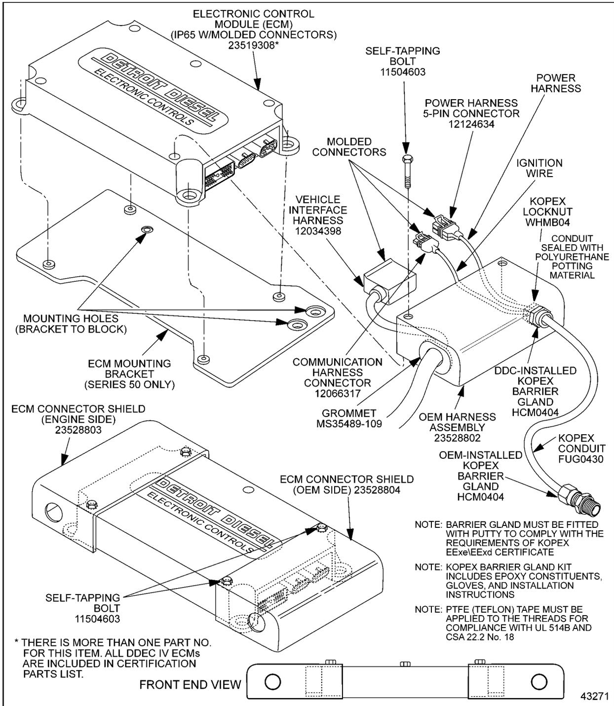
**Figure 3-124 Series 50/Series 60 OEM Side Connectors, Cables, and Shield** is intended to be connected to an EExe junction box.
