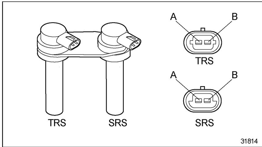
**Figure 3-88 The SRS and TRS - Series 92 6/8V and Series 71 12V Engines**
