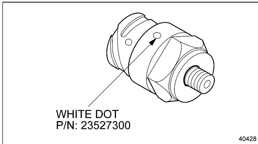
**Figure 3-78 Fuel Pressure Sensor - Series 4000**
