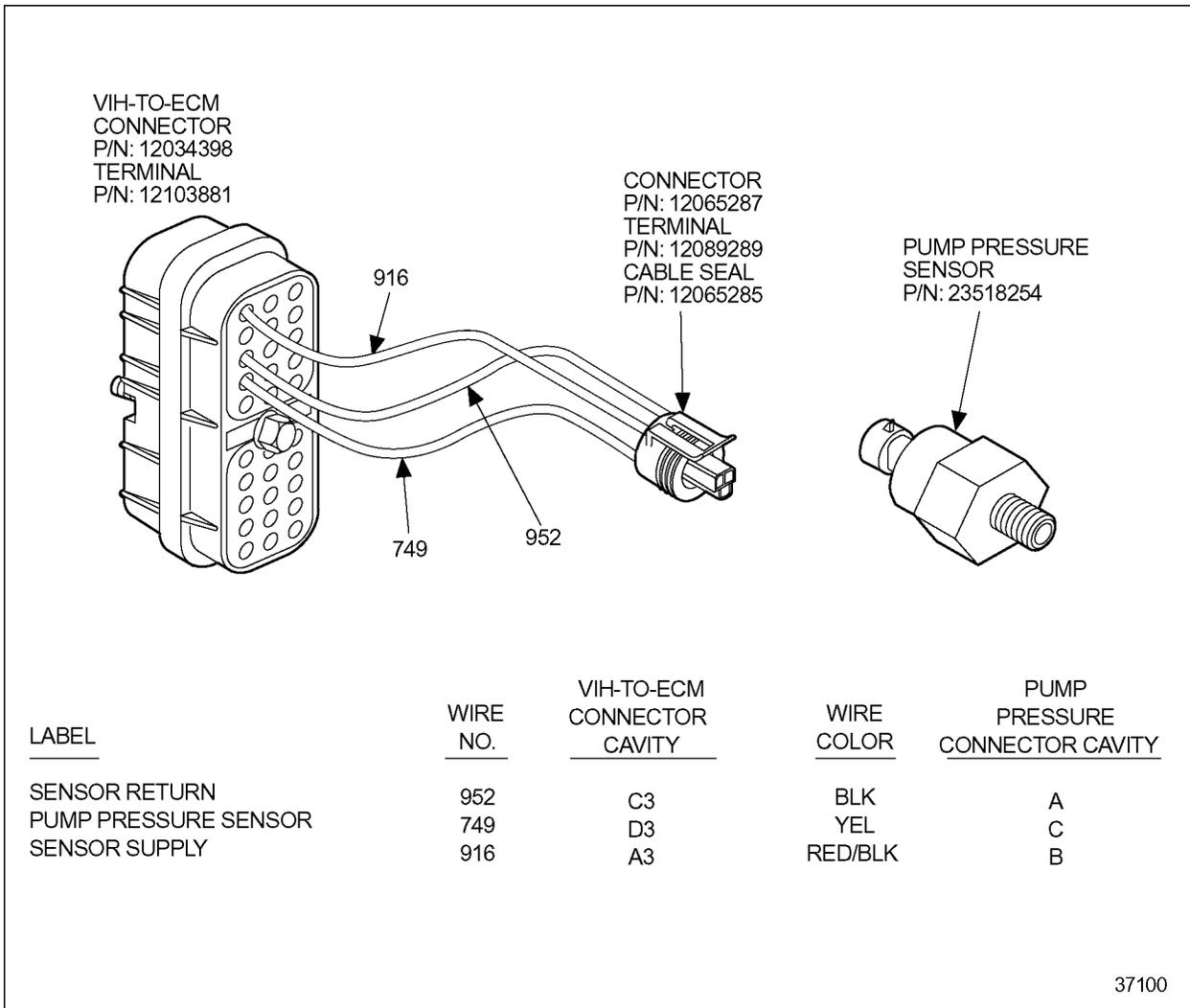
**Figure 3-110 Fire Truck Pump Pressure Sensor Installation**
