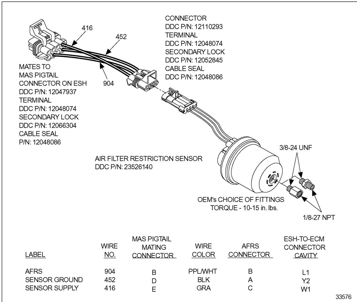
Figure 3-98 Air Filter Restriction Sensor Wiring Diagram
