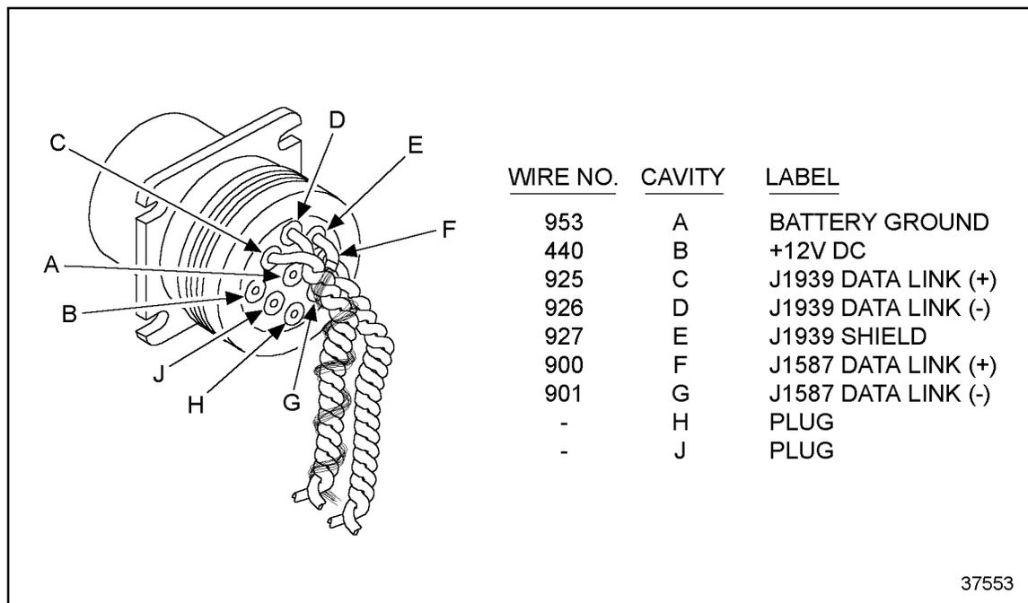
**Figure 3-37 Wiring for Nine-pin Data Link Connector**
