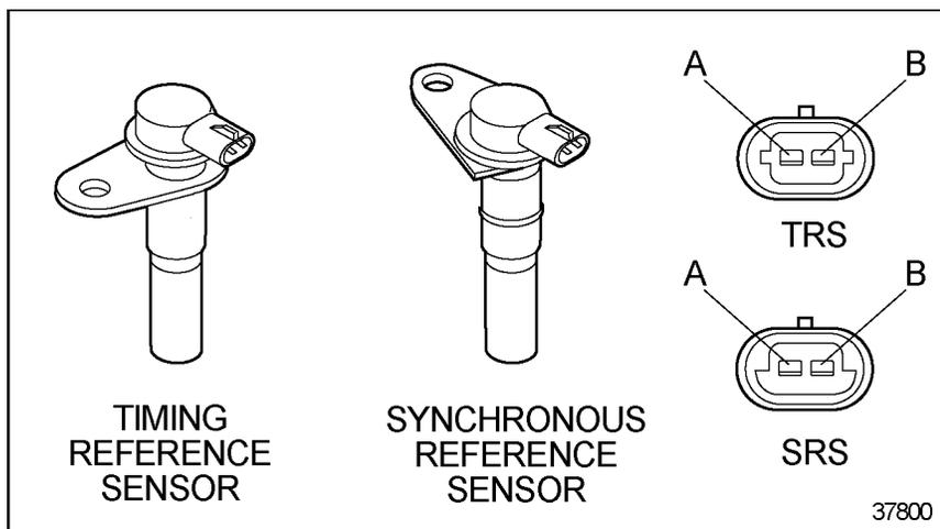
**Figure 3-87 The SRS and TRS - Series 4000**
