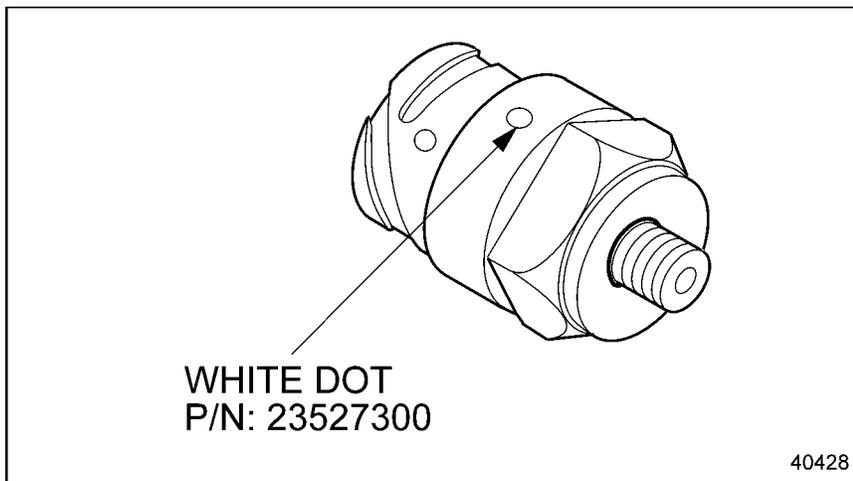
Figure 3-83 Oil Pressure Sensor - Series 2000 and Series 4000
