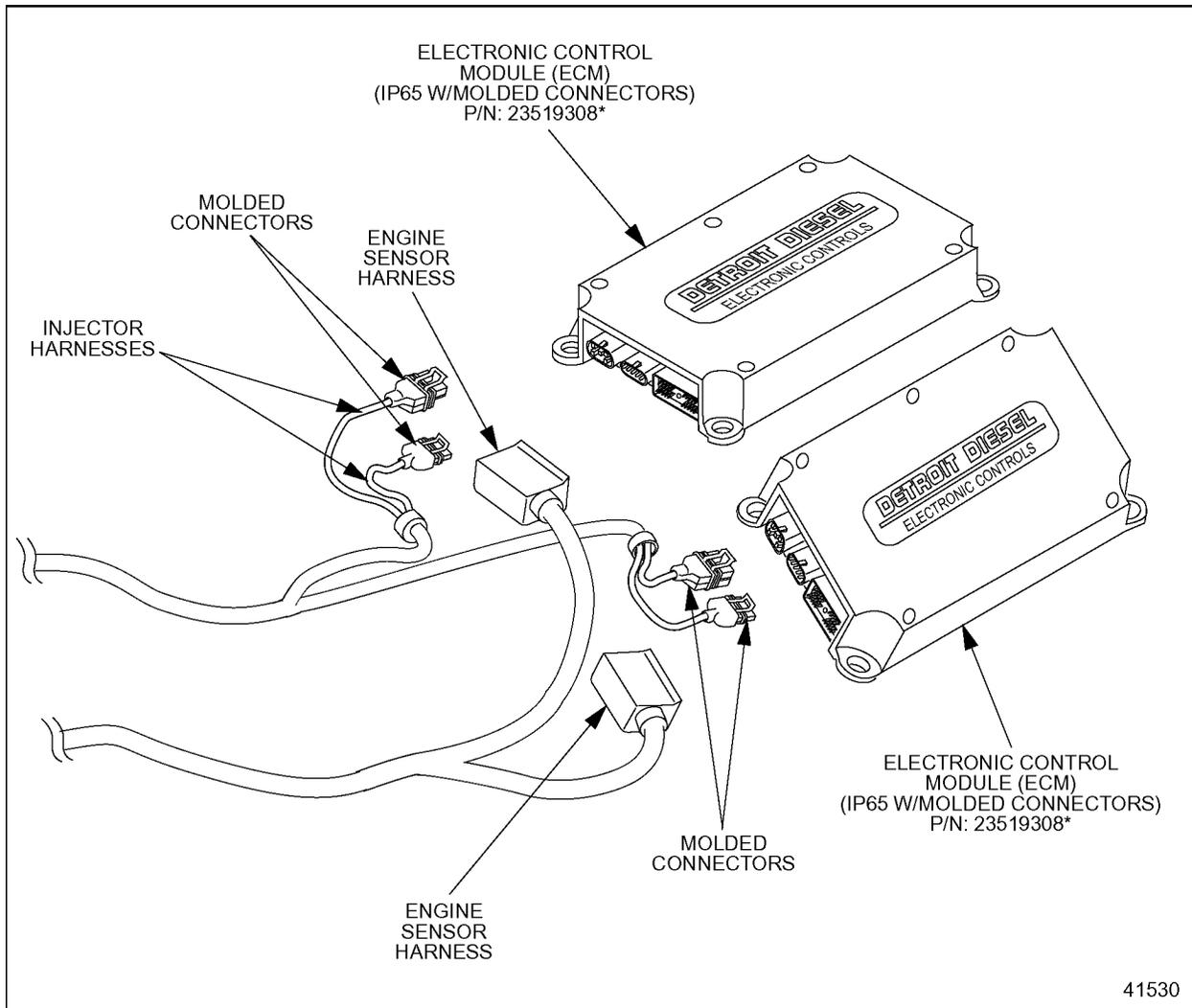
**Figure 3-126 Series 2000 Engine Side Connectors and Cables**
