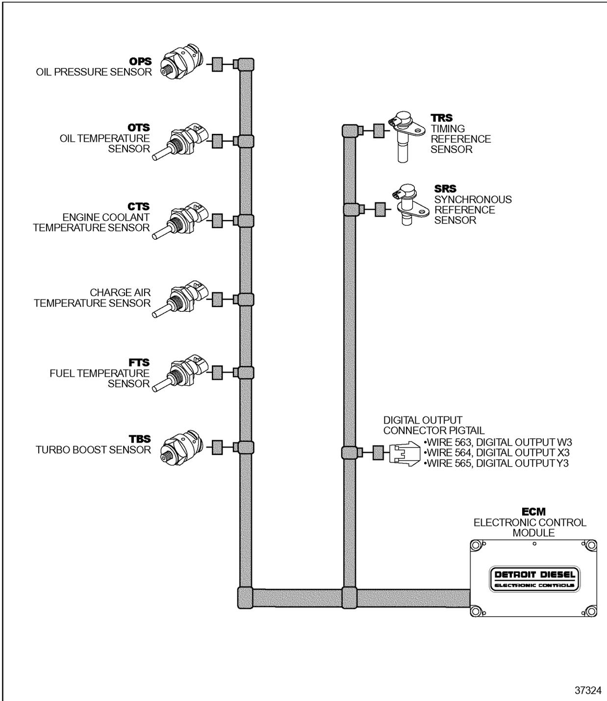
Figure 3-5 Series 2000 Single ECM Genset Engine Sensor Harness
