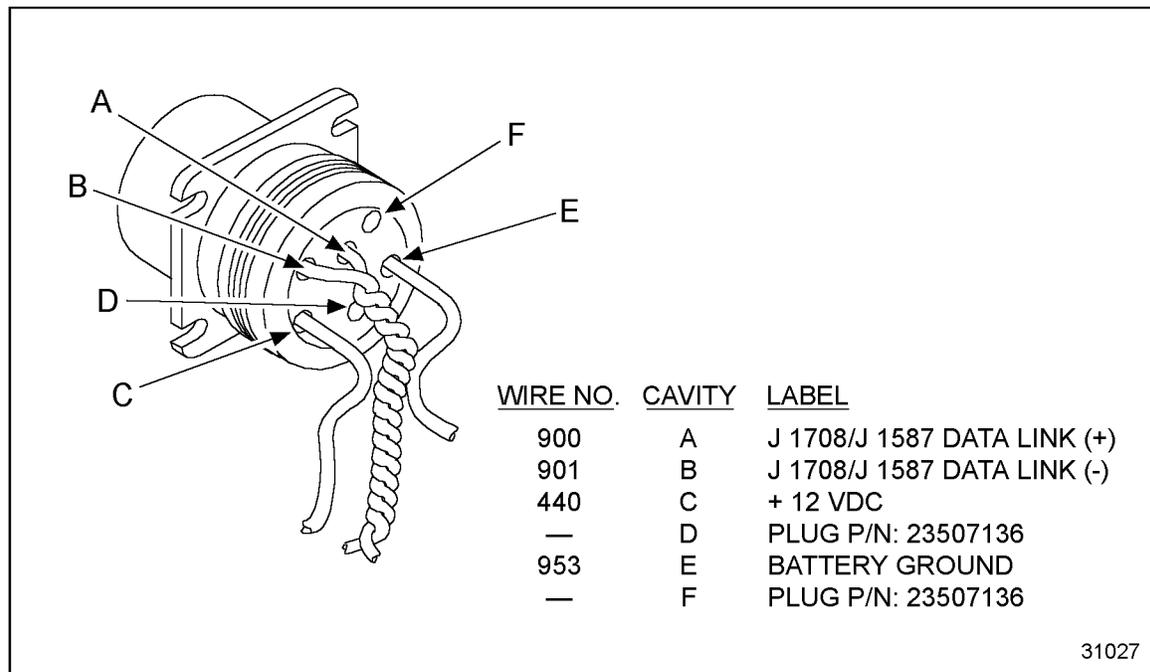
**Figure 3-38 Wiring for Six-pin Data Link Connector**
