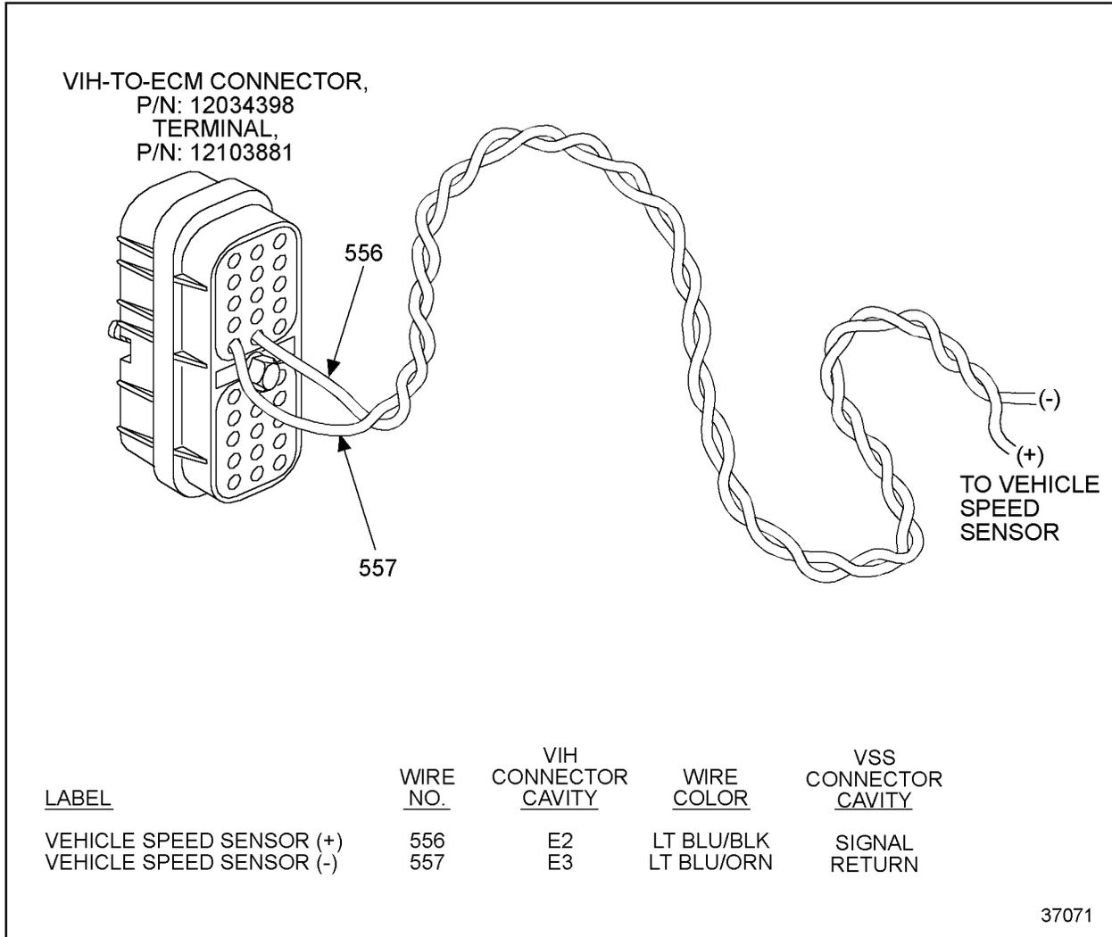
**Figure 3-112 Magnetic Pickup Vehicle Speed Sensor Installation**
