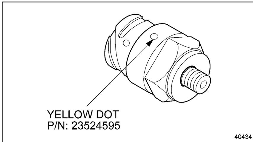
**Figure 3-72 Coolant Pressure Sensor - Series 2000 and Series 4000**
