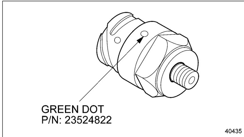
**Figure 3-77 Fuel Pressure Sensor - Series 2000**
