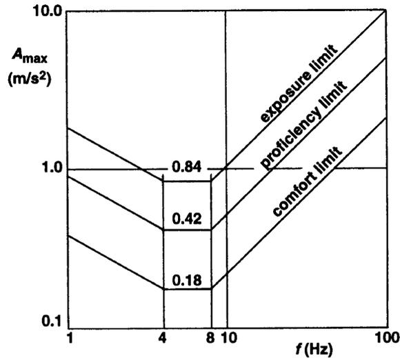
**Figure 3.4.2** Average tolerance of a seated human to vertical vibration at a single frequency, variation with frequency, 8 hour exposure (ISO 2631, 1974).
