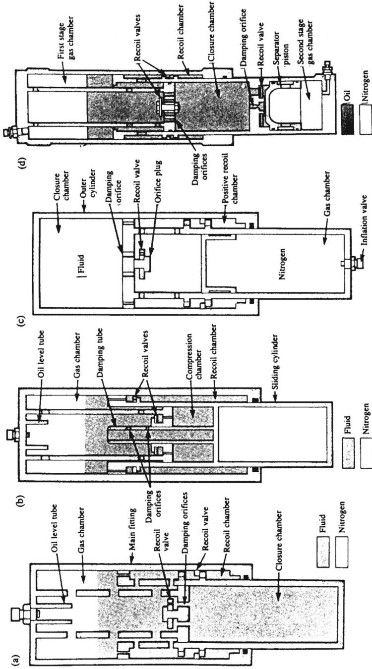
**Figure 6.12.1** Aircraft oleo dampers: (a) unseparated oleo with positive recoil control; (b) unseparated oleo with three level damping position dependent; (c) separator type oleo; (d) two-stage damper oleo (Young, 1986).
