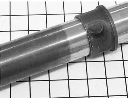
**Plate 8.08** Mild, and insignificant, discoloration and slight corrosion on the steel part of a damper rod, terminating at the chromium plating region.
