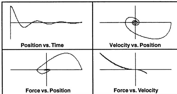
**Figure 11.2.8** Natural vibration of spring + mass + damper from  $X = X_0, V = 0$ . Friction type is asymmetrical quadratic.
