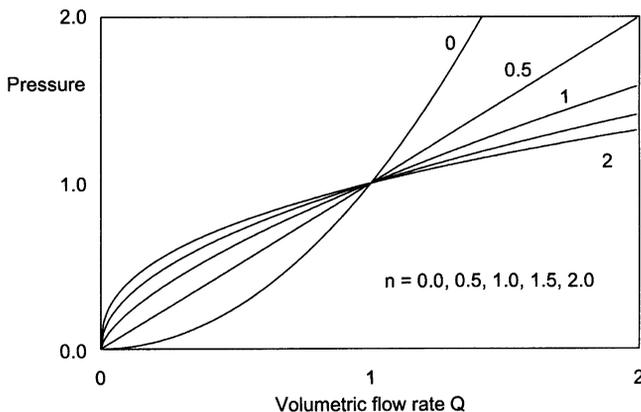
**Figure 6.8.1** Basic variable-area valve  $P(Q)$  characteristic with pressure index  $n$ .
