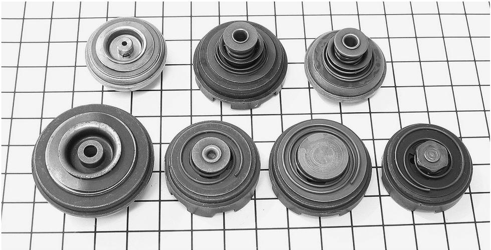
**Plate 4.02** Foot Valves 2. The same seven foot valves seen from the top (compression chamber side). The active valves on this side are for extension, so all must be low pressure loss. The weak springs are apparent. At top left and bottom left, the spring is a single curved shim (planar curvature). At centre and top right may be seen concentric coil springs, the inner one controlling a spool valve, the outer one the expansion seal-shim.
