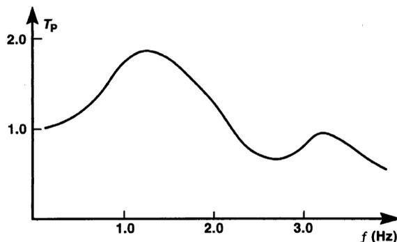
**Figure 3.5.1** Hypothetical transmissibility factor from road to passenger, showing frequency dependence including resonances.
