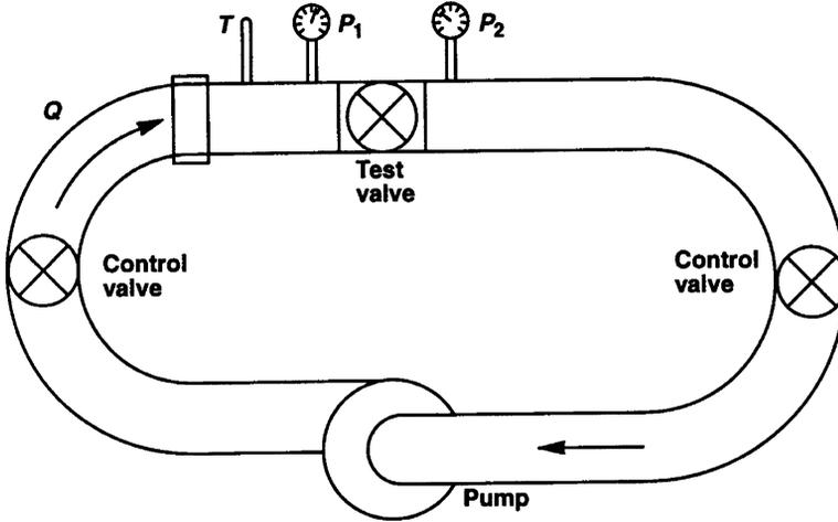
Figure 6.7.1 Valve test circuit.
