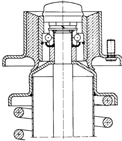
Figure 1.7.8 Strut top mounting (INA).
