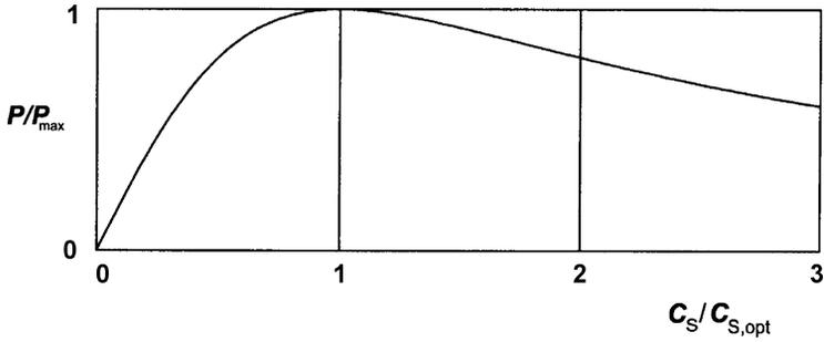
**Figure 2.8.3** Variation of system power dissipation with damping coefficient, with a series spring.
