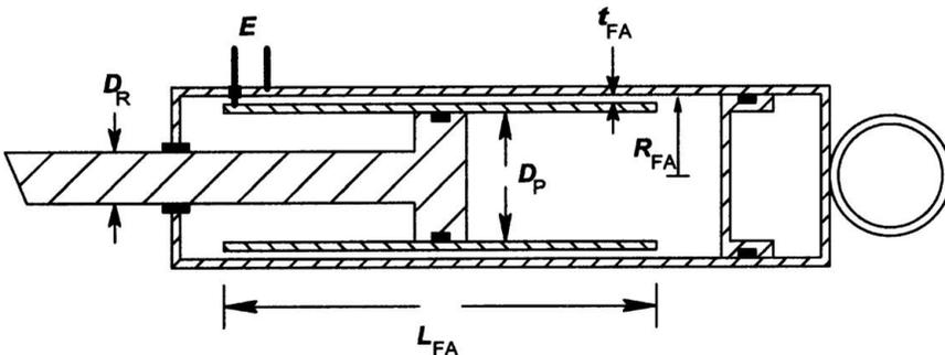
**Figure 9.4.1** Basic design of an ER (electrorheological) damper, showing the fluid flow annulus of length  $L_{FA}$ .
