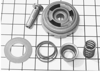
**Plate 7.01** Foot Valve Set 1. Top row: spool valve, to be inserted upwards into the cast or sintered foot valve body seen extension valve side up. Note the large extension flow area moulded into the body. Bottom row: extension valve sealing shim, conical extension valve spring, locating pressing, compression coil spring to go around and retain the stem of the spool valve. A small washer, absent, would be peened onto the top of the spool to retain the spring.
