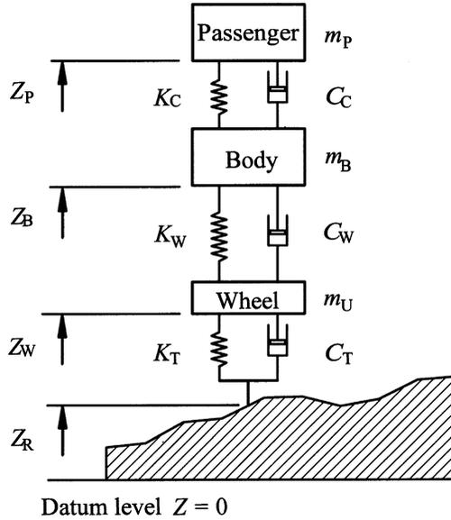
**Figure 3.3.2** Heave ride model including passenger, defining inertia, stiffness and damping coefficient notation and ride positions.
