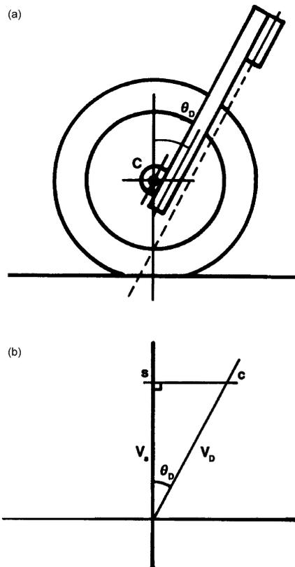
Figure 4.14.1 Motorcycle sliding forks: (a) position diagram; (b) velocity diagram.
