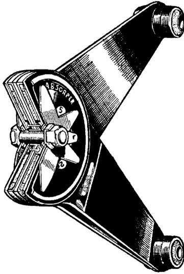
**Figure 1.1.4** The Andre-Hartford scissor-action dry friction damper.
