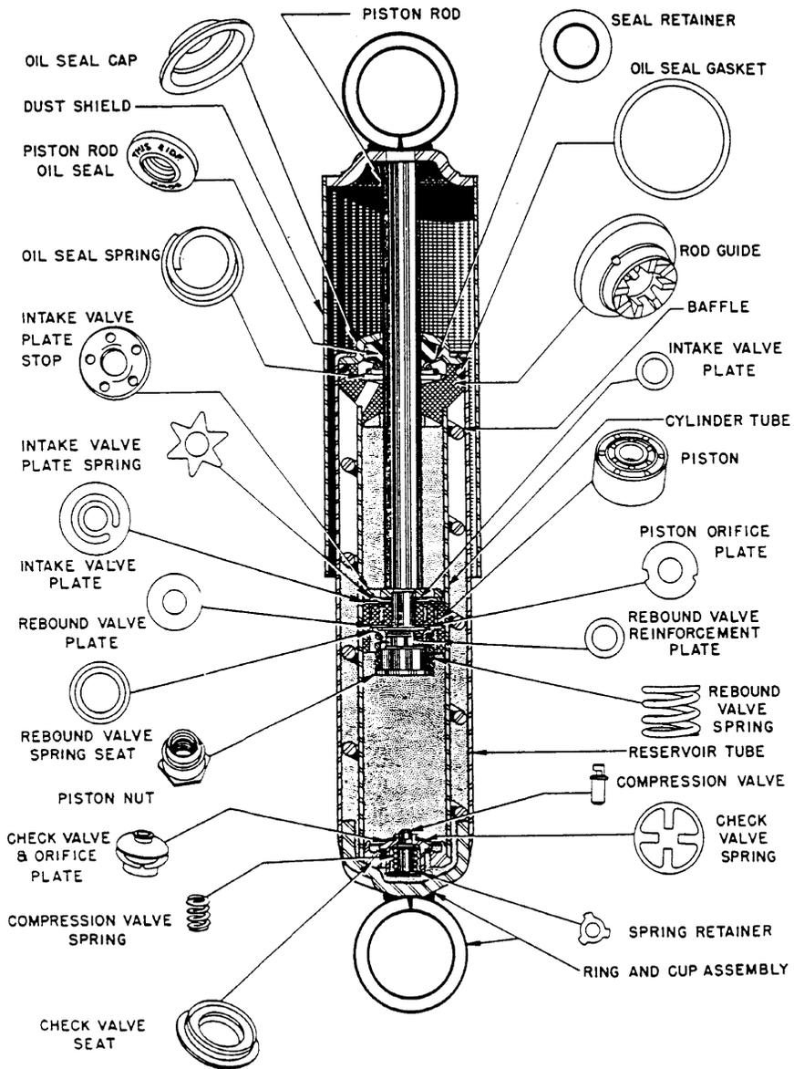
**Figure 1.3.14** Parts of typical conventional telescopic damper of 1950. Note the four-coil air/oil separation rod in the reservoir to discourage the effects of agitation. Reproduced from Peterson (1953) *Proc. National Conference on Industrial Hydraulics*, 7, 23–43.
