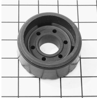
**Plate 5.04** Piston 2, extension valve side. Again, the extension seal shim/disc reaches only the raised rim.
