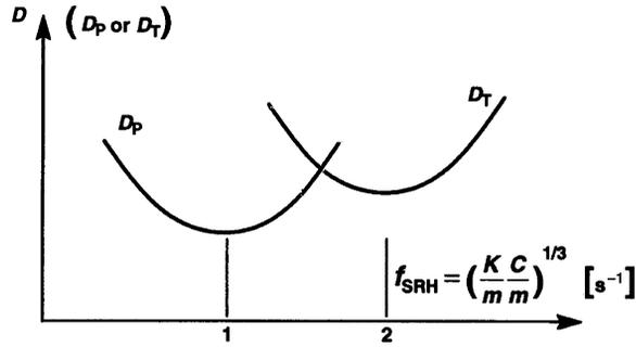
Figure 3.11.4 The effect of the ride-handling parameter on passenger and tyre discomfort.
