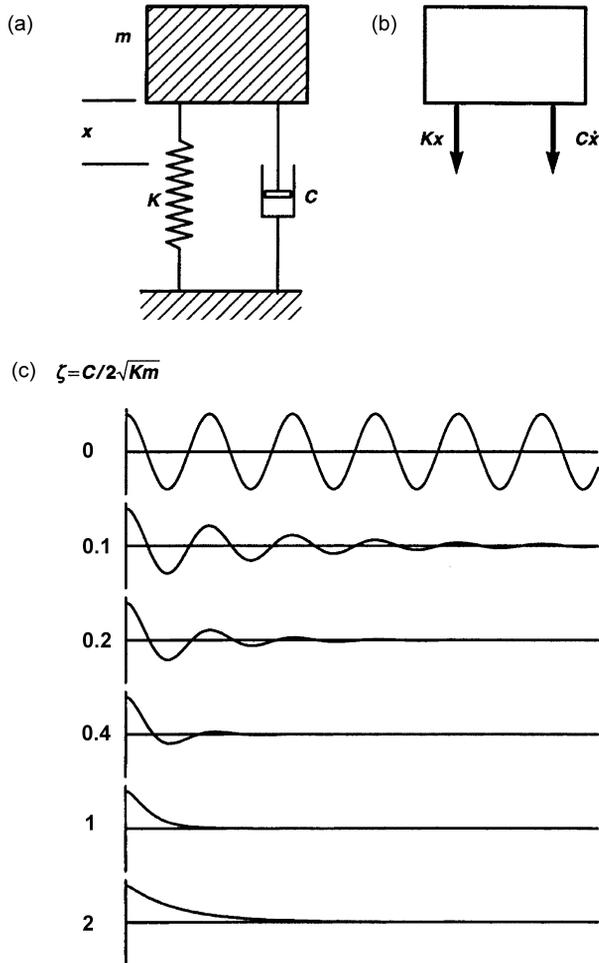
**Figure 2.3.1** Basic linearly-damped 1-dof system: (a) definition sketch; (b) free body diagram; (c) free vibration of system with linear damping for various damping ratios  $\zeta$ .
