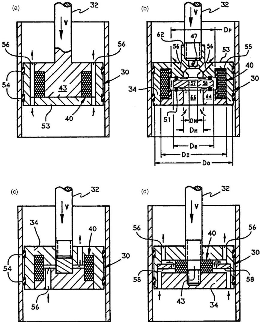
**Figure 9.7.5** Proposed designs of MR damper piston with various fluid paths and magnetic configurations (Carlson and Chrzan, 1994a).
