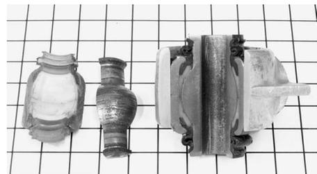
**Plate 2.06** Header 6. Section of the ball joint connector of the previous item, showing metal ball-rod plus various elastomeric supports and seals.
