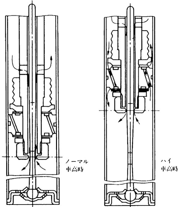
**Figure 6.12.2** Position-sensitive damper using tapered rods. Reproduced from Komamura and Mizumukai (1987) History of Shock Absorbers, *JSAE*, 41(1), pp. 126–131.
