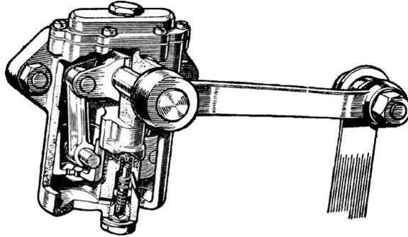
**Figure 1.3.6** Double-piston lever-arm damper with removable valve (Armstrong).
