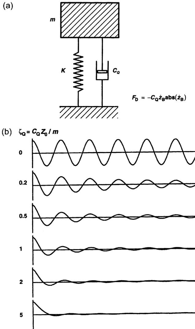
**Figure 2.7.1** (a) Definition sketch of 1-dof system with quadratic damping; (b) free vibration of system with quadratic damping.
