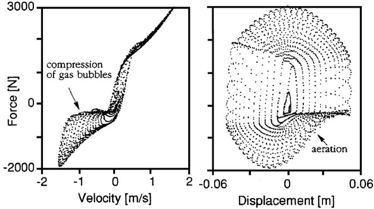
**Figure 7.11.1** The effect of compressibility and cavitation on the damper  $F(V)$  curve, due to bad valve settings, as measured experimentally (from Duym *et al.*, 1997).
