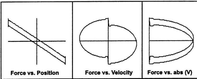
Figure 7.12.7  $F(X)$ ,  $F(V)$  and  $F(\text{abs}(V))$  for a sinusoidal test. Force type: linear spring + stiction.
