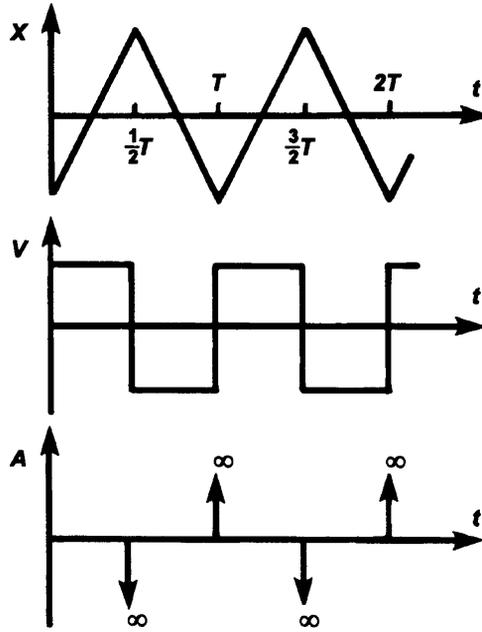
**Figure 11.9.1** Kinematics of ideal triangular waveform displacement test.
