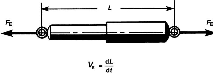
**Figure 7.1.1** Positive velocity and force in extension. The damper is in tension, with its length increasing.
