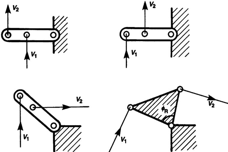
Figure 4.9.3 Simple rockers with various motion ratios.
