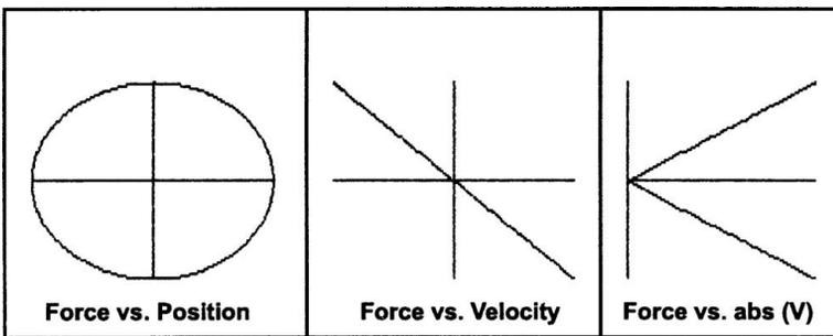
Figure 7.12.8  $F(X)$ ,  $F(V)$  and  $F(\text{abs}(V))$  for a sinusoidal test. Force type:  $-cV$  (linear damper), repeated.
