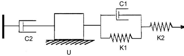
**Figure 9.3.4** A mechanical analogue for an ER material. Reproduced from Gamota and Filisko (1991) Dynamic mechanical studies of electrorheological materials: Moderate frequencies, *Journal of Rheology*, 35, 3.
