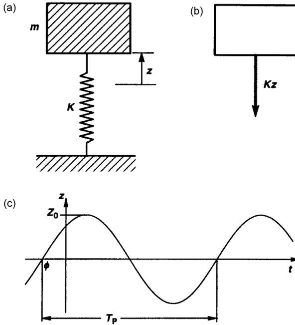
**Figure 2.2.1** Basic undamped 1-dof (degree-of-freedom) vibrating system, position parameter  $z$  from the equilibrium position: (a) definition sketch; (b) free body diagram of mass; (c) free vibration motion  $z(t)$ .
