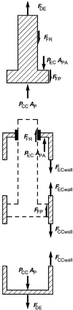
**Figure 7.14.1** Wall forces for a single-tube damper in extension motion (wall force actually distributed circumferentially).
