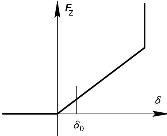
**Figure 3.13.1** Tyre vertical force against tyre vertical deflection, for constant stiffness.
