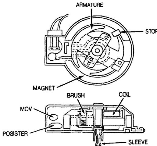
**Figure 6.19.1** Solenoid actuator for adjustable barrel valve (Soltis, 1987).
