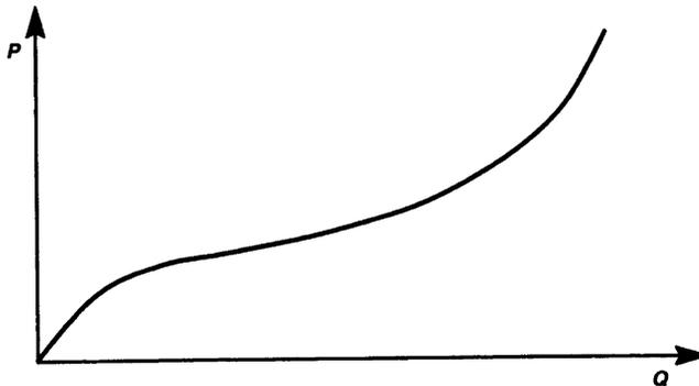
Figure 6.7.2 Typical valve test result.
