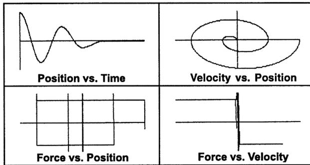
Figure 11.2.2 Natural vibration of spring + mass + damper from  $X = X_0, V = 0$ . Friction type is static + dynamic.
