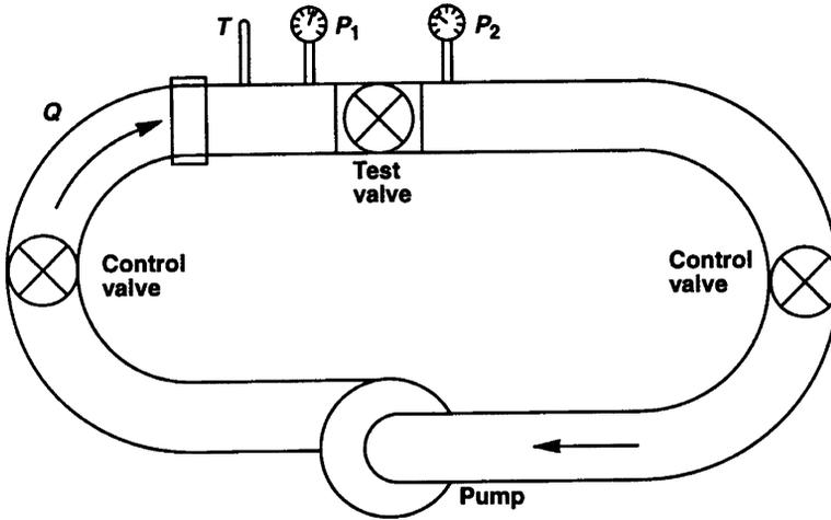
Figure 6.7.1 Valve test circuit.
