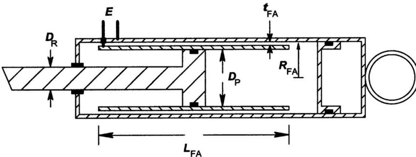
**Figure 9.4.1** Basic design of an ER (electrorheological) damper, showing the fluid flow annulus of length  $L_{FA}$ .
