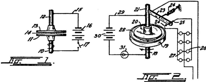
**Figure 9.2.1** The original concept of electrofluid control, of a clutch or a rotary relay, W.M. Winslow (1947) US Patent 2,417,850.
