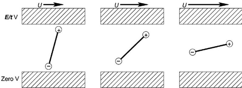
**Figure 9.3.1** Polar particle subject to a constant electric field in varying fluid shear rates.
