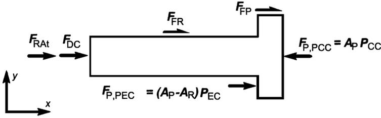
Figure 7.5.2 Free body diagram of piston and rod.
