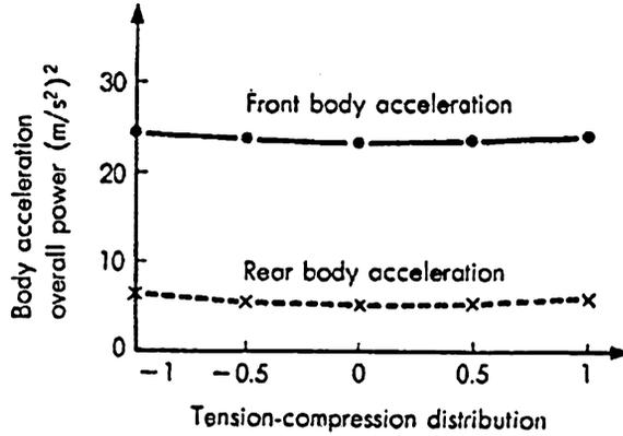
**Figure 3.13.2** The effect of damper force transfer factor  $e_D$  on vehicle body vertical acceleration when driving on a rough road, simulation results. Reproduced from Fukushima, Hidaka and Iwata (1983) Optimum characteristics of automotive shock absorbers under various driving conditions and road surfaces, *JSAE Review*, pp.62–69.
