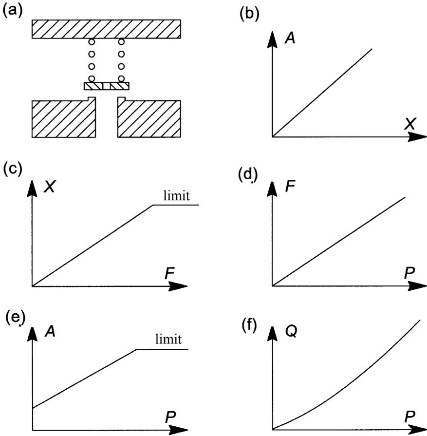
**Figure 6.8.2** Valve  $A(x)$ ,  $x(F)$ ,  $F(P)$ ,  $A(P)$  and  $Q(P)$  characteristics: (a) valve physical configuration; (b) area vs displacement; (c) displacement vs force; (d) force vs pressure; (e) area vs pressure; (f) resulting flowrate vs pressure.
