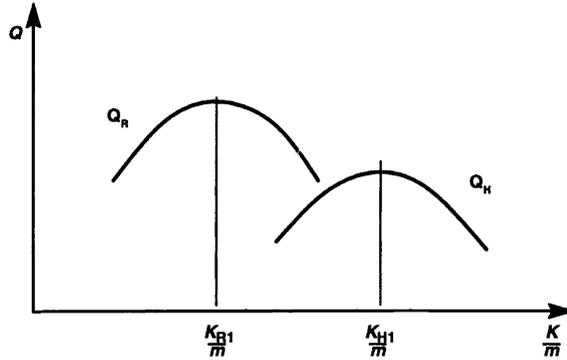
Figure 3.11.1 The influence of suspension stiffness on the quality of ride and handling.
