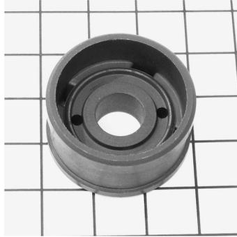
**Plate 5.02** Piston 1, extension valve side. The sealing shim/disc reaches only the raised rim here, so flow into the outer holes, for compression, is free.
