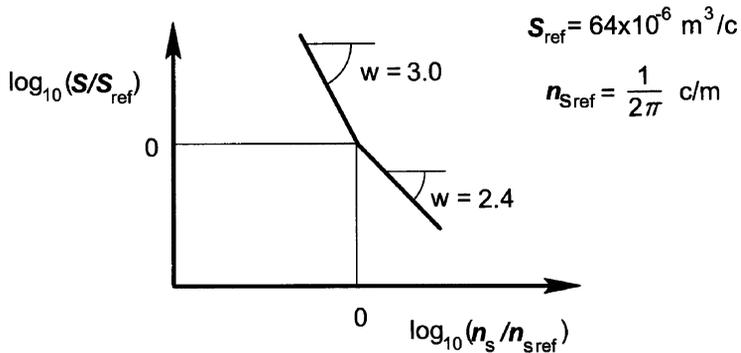
Figure 3.2.3 The ISO spectral road model.
