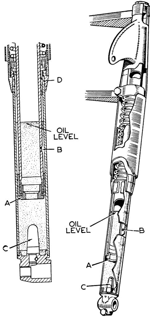
Figure 1.5.1 The BSA Telefork motorcycle spring-damper unit.
