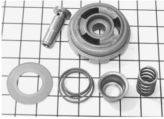
**Plate 7.01** Foot Valve Set 1. Top row: spool valve, to be inserted upwards into the cast or sintered foot valve body seen extension valve side up. Note the large extension flow area moulded into the body. Bottom row: extension valve sealing shim, conical extension valve spring, locating pressing, compression coil spring to go around and retain the stem of the spool valve. A small washer, absent, would be peened onto the top of the spool to retain the spring.
