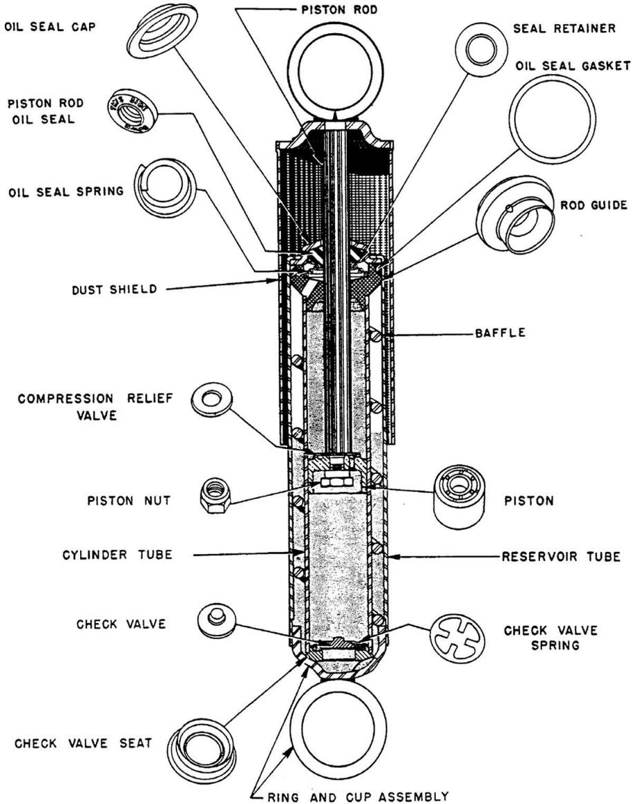
**Figure 7.1.4** The Chrysler Oriflow damper introduced in 1951 was an attempt to move away from the simple abrupt hydraulic blow-off characteristic to something nearer to a linear  $F(V)$  curve. Reproduced from Peterson (1953) *Proc. National Conference on Industrial Hydraulics*, 7, 23–43.
