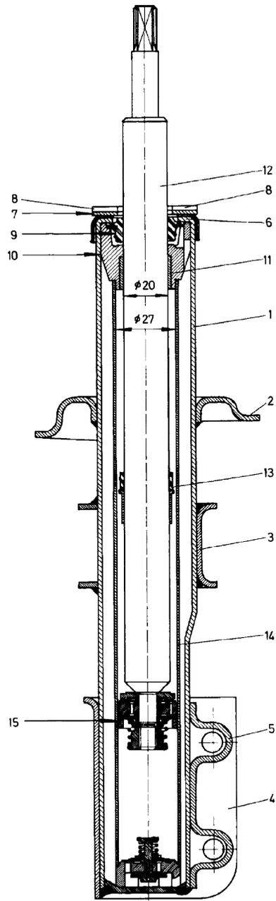
**Figure 1.3.20** Sectional view of a front strut for a small car. Piston diameter 27 mm, rod diameter 20 mm. 1 outer cylinder; 2 spring seat; 3 guard; 4, 5 wheel hub fixture; 6 rolled closure; 7, 8 bump stop seat; 9 seal; 10 upper moulding; 11 bearing; 12 rod; 13 stroke limiter (?); 14 inner (working) cylinder; 15 piston (Fiat/Monroe).
