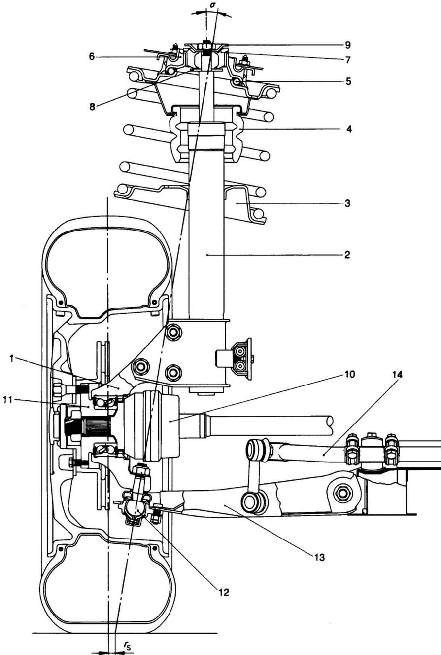
**Figure 7.3.2** An example front strut, illustrating how the vertical and cornering forces at the base of the tyre give a moment about the bottom ball joint applied to the strut, reacted at the piston and rod bearing (Lancia).
