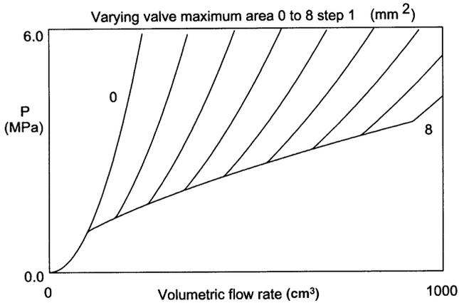
Figure 8.2.4 Effect of adjustment to maximum area.
