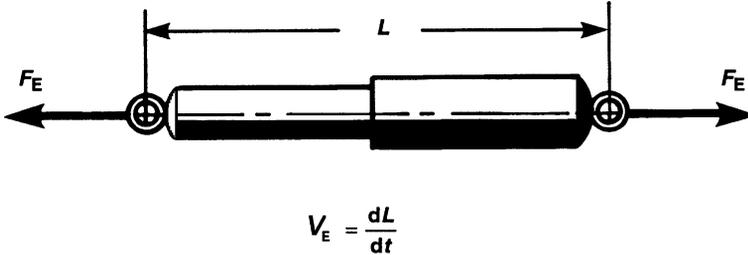
**Figure 7.1.1** Positive velocity and force in extension. The damper is in tension, with its length increasing.
