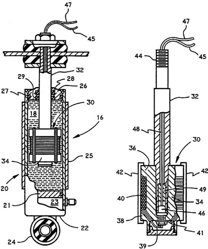
**Figure 9.7.4** Proposed design of MR damper with a magnetic path through both piston and cylinder (Carlson and Chrzan; 1994a). J.D. Carlson and M.J. Chrzan (1994) US Patent 5,277,281.
