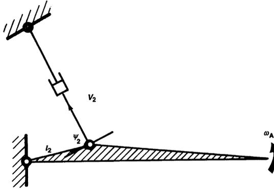
Figure 4.10.2 Rigid arm suspension shown in elevation.
