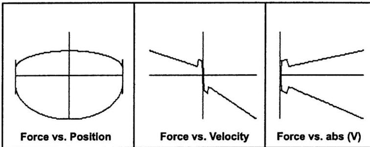
Figure 7.12.13  $F(X)$ ,  $F(V)$  and  $F(\text{abs}(V))$  for a sinusoidal test. Force type: bilinear + stiction.
