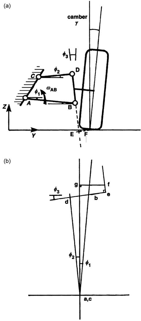
Figure 4.11.1 Double wishbone suspension: (a) position diagram; (b) velocity diagram.
