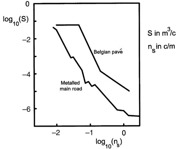
Figure 3.2.1 The spectral analysis of two example roads (spectral density versus spatial frequency).
