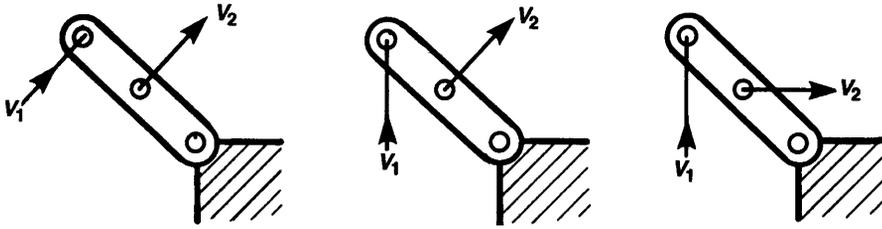
Figure 4.9.4 Simple rockers with various rising rates (zero in the first case).
