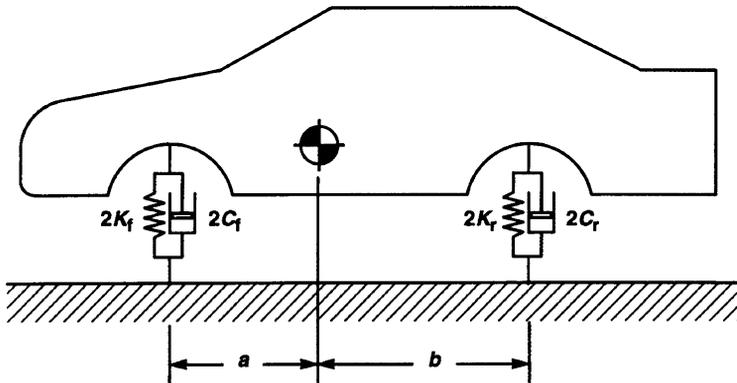
**Figure 2.18.1** Vehicle with longitudinal asymmetry, i.e. centre of mass not at the mid-wheelbase, and/or different front and rear suspension parameters (with zero damping in Section 2.18).
