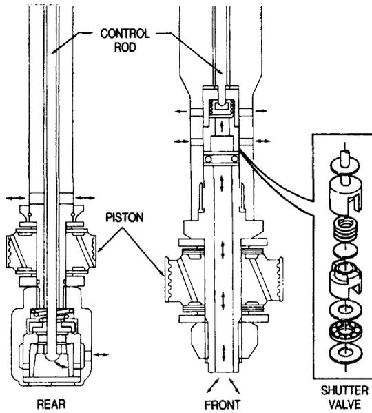
Figure 6.19.4 Rotary barrel valve, flow shown in soft position (Soltis, 1987).
