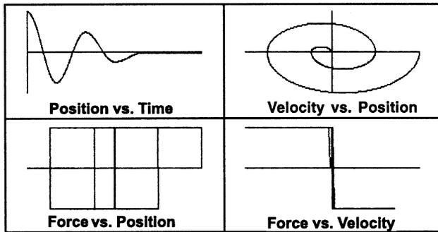
Figure 11.2.1 Natural vibration of spring + mass + damper from  $X = X_0, V = 0$ . Friction type is Coulomb.
