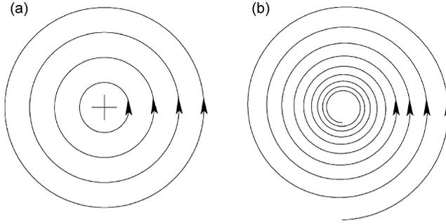
**Figure 5.24.1** The circular flow pattern of a vortex (a) simple, (b) spiralling in.
