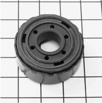
**Plate 5.03** Piston 2, compression valve side. Similar operating principle to Piston 1, but with detail changes. Three holes for compression flow up into the outer annulus, six holes for extension flow down.
