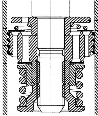
**Figure 6.3.3** Piston with coil-spring disc valves for compression and conical spring for compression. The extension disc in some cases acts as a shim at low pressures. Reproduced from Duym (2000) Simulation tools, modelling and identification, for an automotive shock absorber in the context of vehicle dynamics, *Vehicle System Dynamics*, 33, pp. 261–285, with permission from Taylor and Francis Ltd, [www.informaworld.com](http://www.informaworld.com)
