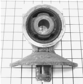
**Plate 8.03** Rubber bush in a damper eye, featuring cavities at the top and bottom to give reduced rigidity in the line of action of the damper.
