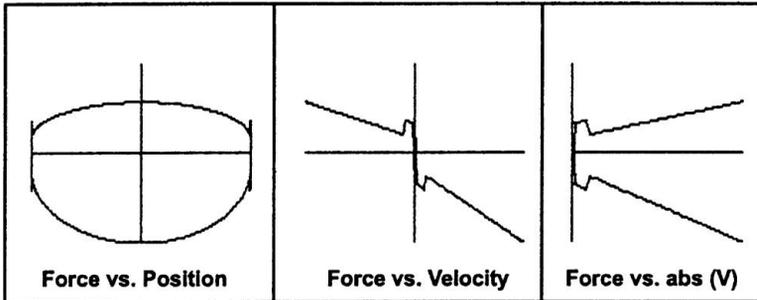
Figure 7.12.13  $F(X)$ ,  $F(V)$  and  $F(\text{abs}(V))$  for a sinusoidal test. Force type: bilinear + stiction.
