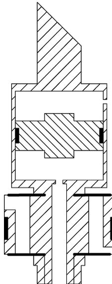
**Figure 6.16.4** Use of a floating secondary piston in a chamber, to give a stroke-sensitive parallel flow and force.
