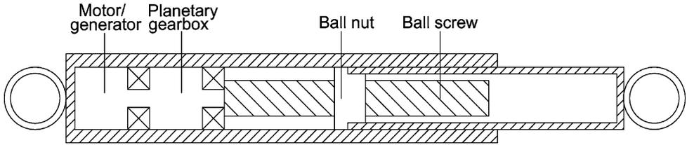
**Figure 1.3.29** Electromagnetic damper configuration (after Suda *et al.*, 2004).
