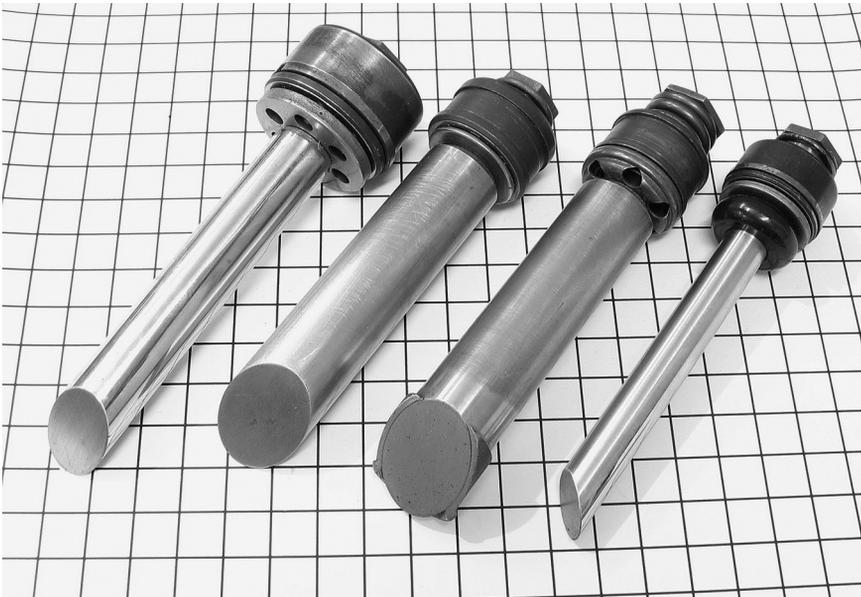
**Plate 3.02** Piston Valves 2. The same pistons and rods as in the previous figure, seen from the rod (extension chamber) side.
