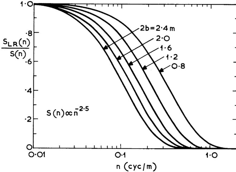
**Figure 3.2.5** Coherence between adjacent tracks, on the assumption of a spectral density with  $W = 2.5$  and isotropy. The track spacing is  $2b$ . Reproduced from Robson (1979) Road surface description and vehicle response, *IJVD*, 1(1), pp.25–35.
