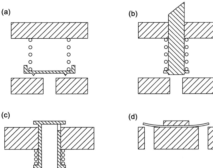
**Figure 6.2.1** Basic valve types: (a) disc valve supported by coil spring; (b) rod valve with coil spring; (c) spool valve with coil spring; (d) shim valve.
