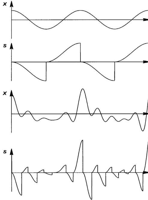
**Figure 6.16.1** Instantaneous stroke derived from displacement: top sinusoidal, bottom random.
