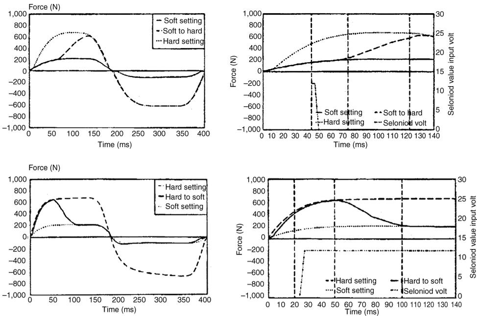
Figure 8.8.4 Delays on a three-state switchable damper. Reproduced from Abd-El-Tawwab, Crolla and Plummer (1998) The characteristics of a three-state switchable damper, *Journal of Low Frequency Noise, Vibration and Active Control*, 17(2), pp. 85–96.
