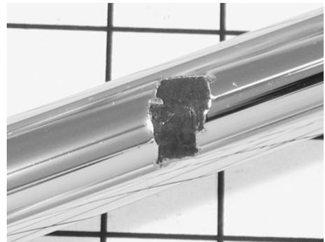
**Plate 8.11** Flaking of chromium plating on a damper rod, probably caused by inadequate preparation of the base metal and poor adhesion of the plating.
