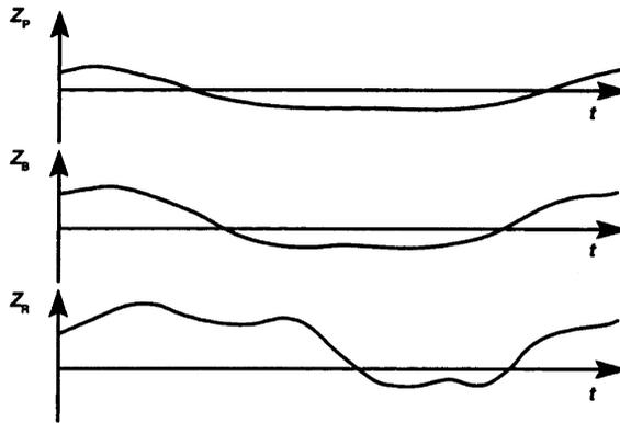
**Figure 3.4.1** Passenger and vehicle body ride positions in response to road position, as functions of time.
