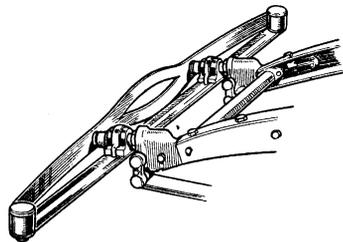
**Figure 2.11.2** An early Frahm-type torsional vibration absorber. The bumper vibrated in ‘roll’ on the rubber mountings, reducing scuttle shake (Wilmot Breeden, 1938).
