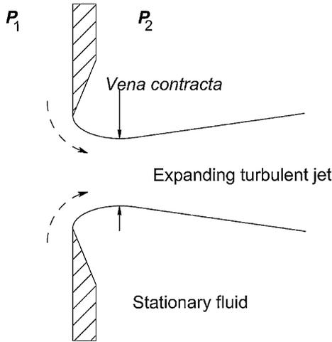
Figure 5.22.1 Flow through a sharp-edged orifice.
