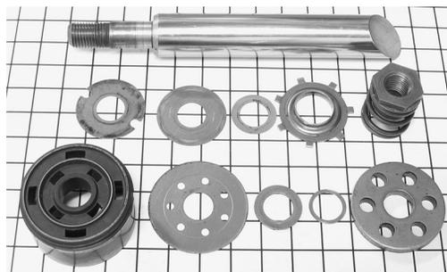
**Plate 6.03** Piston Valve Set 3. Middle row: extension valve parts, notched 0.20 mm sealing shim, 0.20 mm support shim, a small 0.20 m spacer, 0.9 mm backing plate, coil spring and sleeve nut. Bottom row: piston, compression valve side up, 0.35 mm compression shim with holes for extension feed from the inner ring seal and feed to inner annulus during extension, two spacers of 0.9 mm and 0.20 mm, rigid 3.7 mm backing plate with feed holes.
