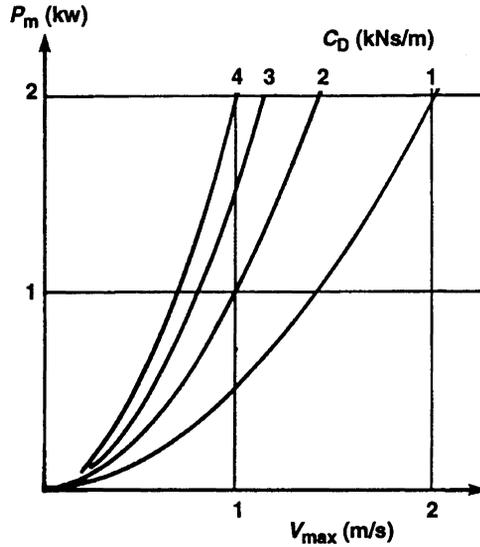
Figure 11.7.1 Damper mean power dissipation versus velocity amplitude, for sinusoidal motion.
