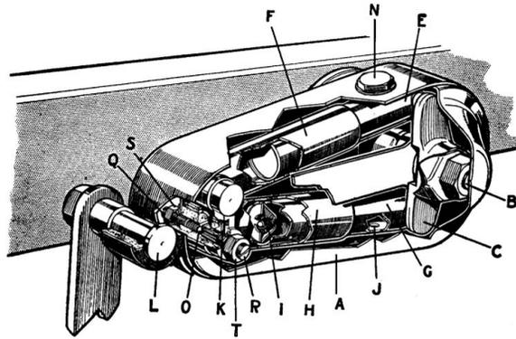
**Figure 1.1.21** The Armstrong 'double telescopic lever arm' damper.
