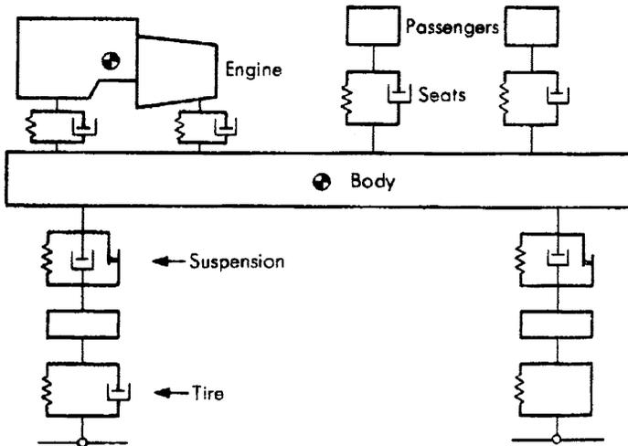
**Figure 3.12.3** Simulation model used in velocity and stroke damper studies. Reproduced from Fukushima, Hidaka and Iwata (1983) Optimum characteristics of automotive shock absorbers under various driving conditions and road surfaces, *JSAE Review*, pp.62-69.
