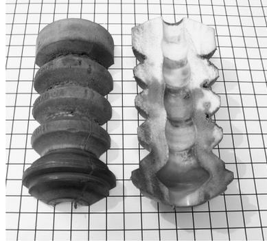
**Plate 8.02** Sectioned polyurethane bump stop from a strut, after 10 years service showing significant deterioration, with mechanical degradation and oil soaking, but still fully functional. 73 g, lower density than natural rubber.
