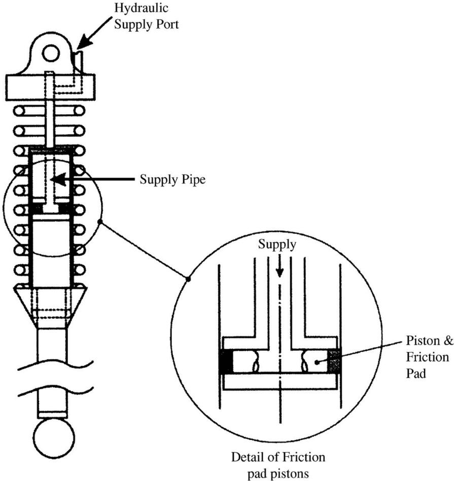
**Figure 7.3.1** A dry friction telescopic damper in which the normal force is controlled hydraulically. Reprinted from *Control Engineering Practice*, 12, Guglielmino and Edge. A controlled friction damper for vehicle applications, pp.431–443, Copyright 2004, with permission from Elsevier.
