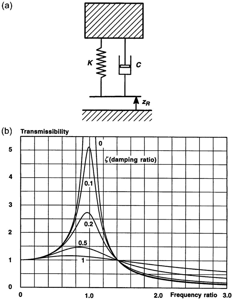
**Figure 2.5.1** (a) Damped 1-dof model vehicle stimulated by road displacements; (b) transmissibility of a damped 1-dof. suspension.
