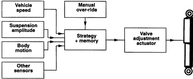
Figure 8.8.1 Automatic adjustment.
