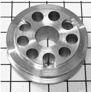
**Plate 5.11** Piston 6, compression valve side. A 3/6 hole shim-pack piston in machined bar-stock aluminium alloy. Six holes for compression flow. Three other holes with side notches allow extension flow without triangulating the shims.
