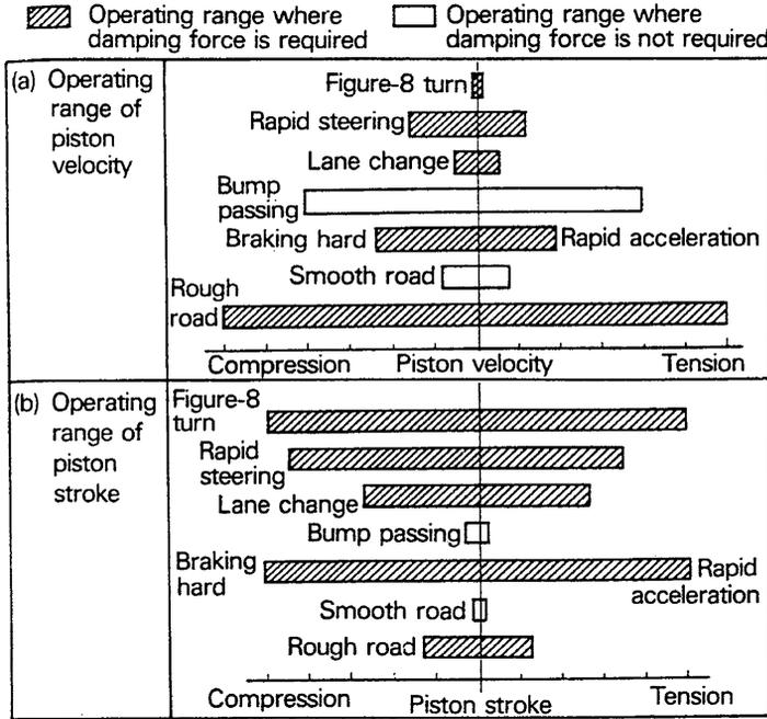
**Figure 3.12.2** Damper operating range analysed by: (a) damper velocity; (b) damper stroke. Reproduced from Fukushima, Hidaka and Iwata (1983) Optimum characteristics of automotive shock absorbers under various driving conditions and road surfaces, *JSAE Review*, pp.62-69.
