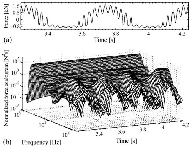
**Figure 7.16.2** Damper scalogram up to 100 Hz (Yung and Cole, 2005).
