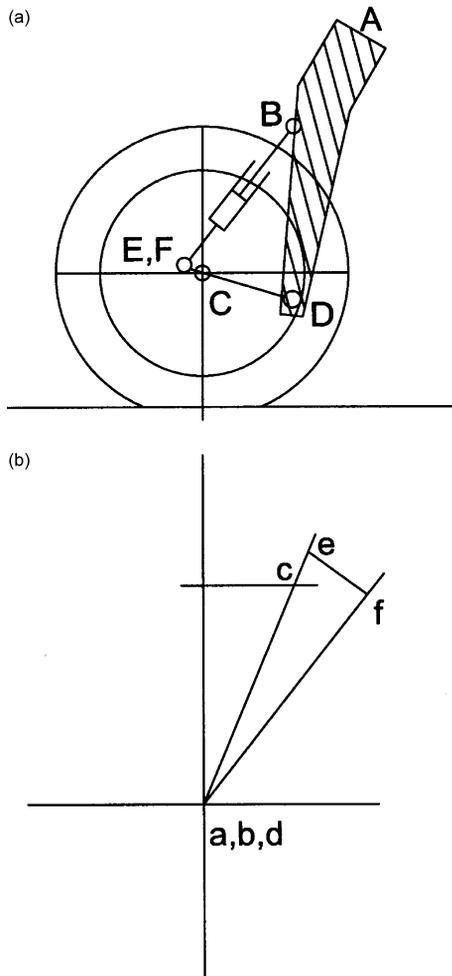
Figure 4.14.3 Motorcycle front leading link: (a) position diagram; (b) velocity diagram.
