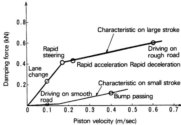
**Figure 3.12.4** Optimum damper characteristics. Reproduced from Fukushima, Hidaka and Iwata (1983) Optimum characteristics of automotive shock absorbers under various driving conditions and road surfaces, *JSAE Review*, pp.62–69.
