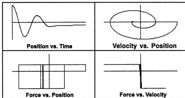
**Figure 11.2.5** Natural vibration of spring + mass + damper from  $X = X_0, V = 0$ . Friction type is asymmetrical Coulomb (fluid blow-off).
