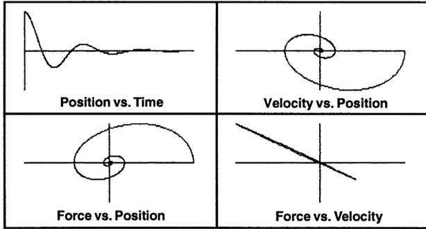
**Figure 11.2.3** Natural vibration of spring + mass + damper from  $X = X_0, V = 0$ . Friction type is linear symmetrical.
