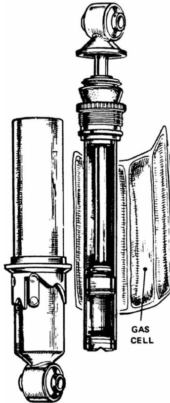
**Figure 5.15.1** The Girling Arcton damper, which used a nylon sleeve containing the gas to prevent emulsification of the oil.
