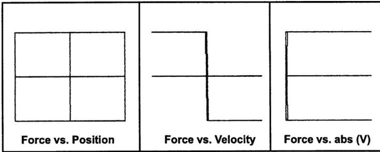
Figure 7.12.4  $F(X)$ ,  $F(V)$  and  $F(\text{abs}(V))$  for a sinusoidal test. Force type:  $-c\text{sgn}(V)$  (Coulomb friction).
