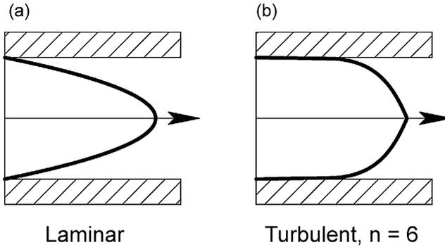
**Figure 5.20.1** Velocity profiles for: (a) laminar; (b) turbulent flow ( $n = 6$ ).
