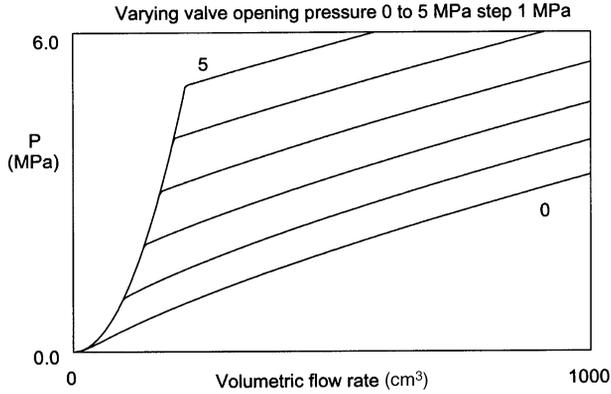
**Figure 8.2.5** Effect of adjustment to initial pressure  $P_{vfc}$ .
