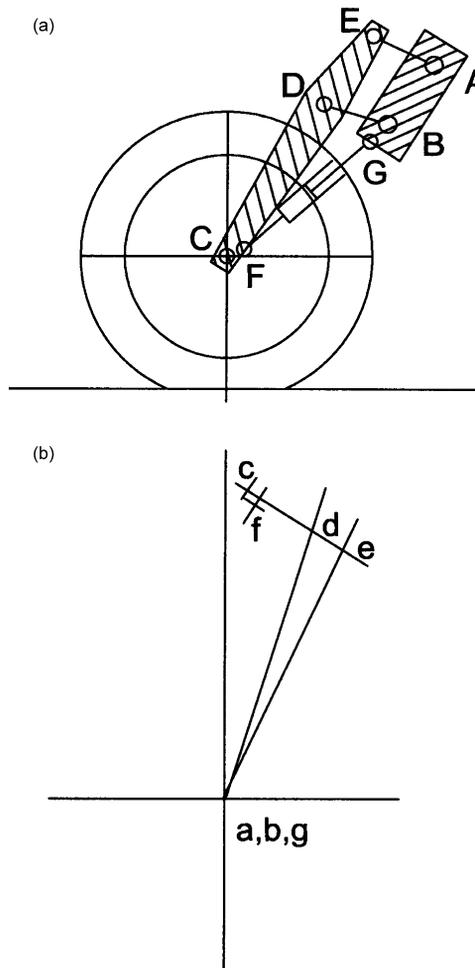
**Figure 4.14.4** Motorcycle front girder forks: (a) position diagram; (b) velocity diagram.
