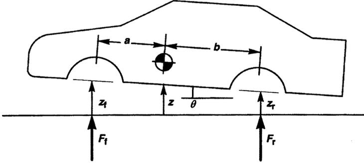
Figure 2.18.2 Vehicle body position with heave and pitch deflections.
