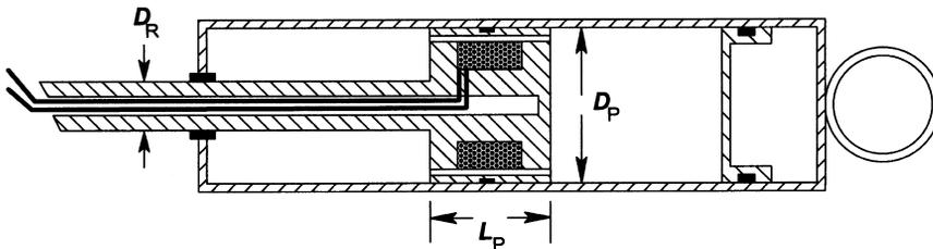
**Figure 9.7.1** A basic design for a single-tube MR damper.
