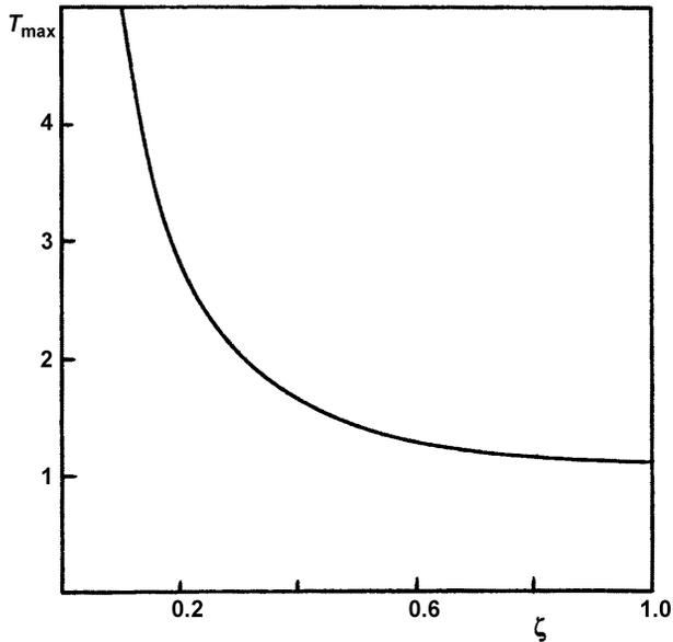
Figure 2.5.2 Peak transmissibility versus damping ratio.
