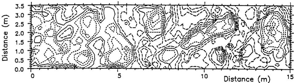
**Figure 3.2.6** Contour map of MIRA Belgian Pavé test track. This is similar to an isotropic surface. Long dashes are contours below datum, short ones above. Reproduced from Cebon and Newland (1984) The artificial generation of road surface topography by the inverse FFT method, *Proc. 8th IAVSD-IUTAM Symp.*, Taylor & Francis, 1984, pp.29–42.
