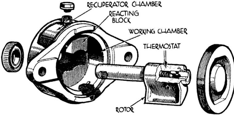
**Figure 1.3.3** The Luvax rotary vane hydraulic damper, which featured thermostatic compensation of variation of oil properties. This was a genuine improvement on earlier vane types. The vane shape results in a radial force that takes up any freedom in the bearing in a way that minimises vane leakage (The Motor Manual, 1939).
