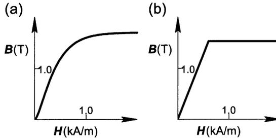
**Figure 9.7.3** Magnetic response of a damper piston steel: (a) real; (b) linear model with saturation.
