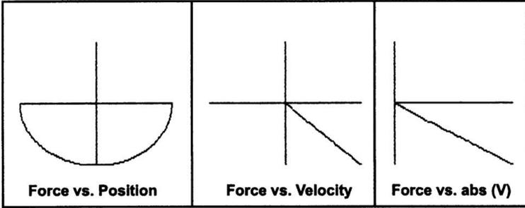
Figure 7.12.10  $F(X)$ ,  $F(V)$  and  $F(\text{abs}(V))$  for a sinusoidal test. Force type: unidirectional linear damper.
