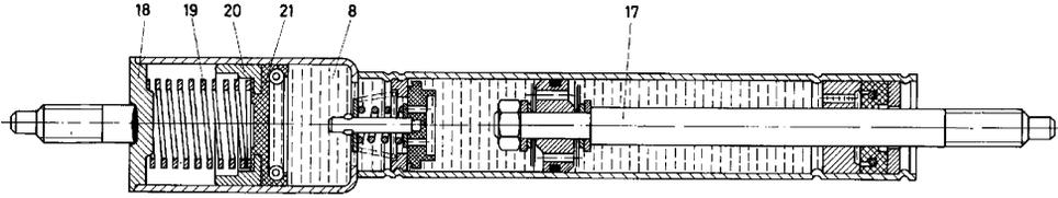
**Figure 1.3.26** Steering damper of basic de Carbon layout, having a free piston separating the oil from the gas chamber, but with spring assistance. The piston has two shim packs. The foot valve has a coil spring blow-off valve (Stabilus).
