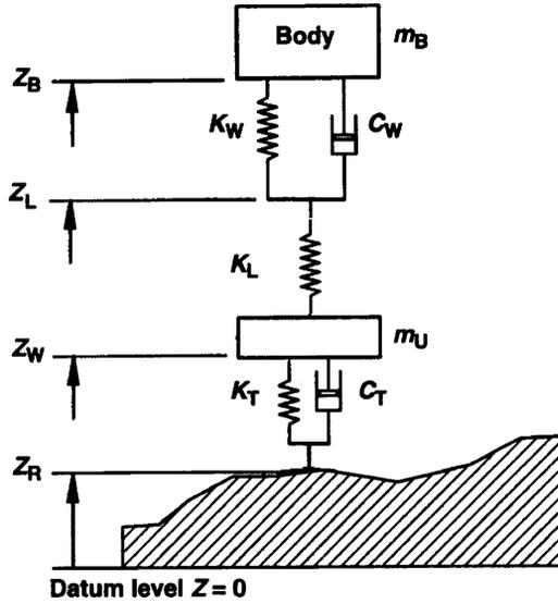
Figure 4.6.1 Heave-only suspension model including link compliance  $K_L$ .
