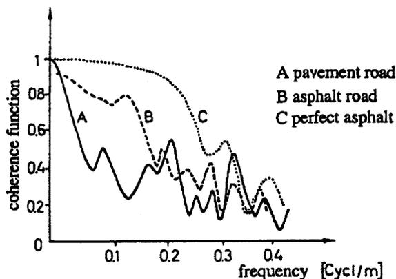
**Figure 3.2.4** Coherence between two adjacent tracks. Reproduced with permission from Verschoore, Duquesne and Kermis (1996) Determination of the vibration comfort of vehicles by means of simulation and measurement, *Eur. J. Mech. Eng.*, 41(3), pp.137–143.
