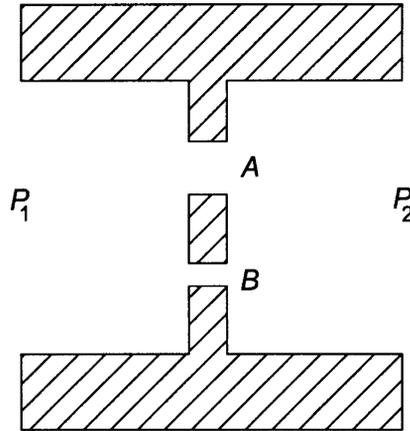
Figure 5.23.1 Parallel orifices.
