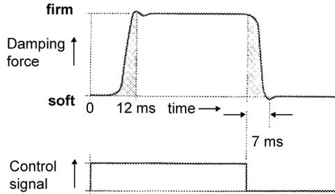
Figure 8.8.3 Response of a switchable damper (Decker *et al.*, 1990).
