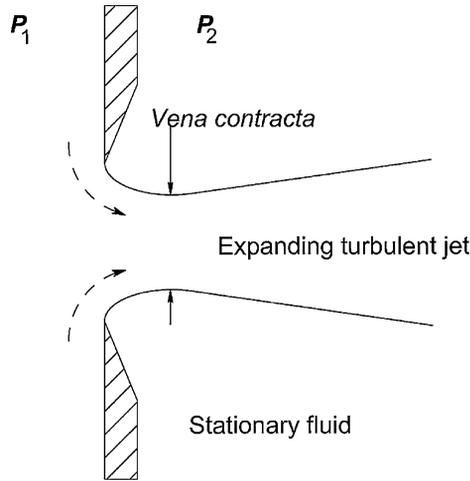
Figure 5.22.1 Flow through a sharp-edged orifice.
