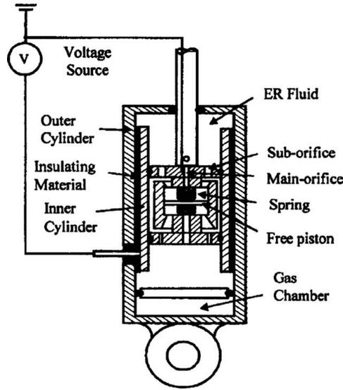
Figure 9.5.1 Configuration of a damper with an ER-controlled valve (Choi, 2003).
