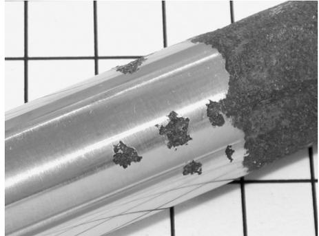
**Plate 8.10** Severe pitting and general corrosion at and near the exposed end of a damper rod.
