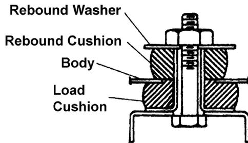
Figure 1.7.7 Asymmetrical damper bushing (Puydak and Auda, 1966).
