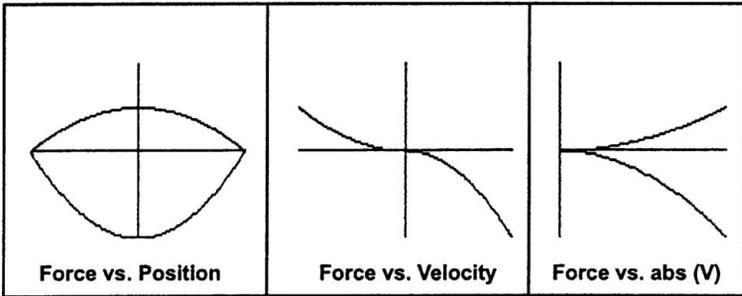
Figure 7.12.12  $F(X)$ ,  $F(V)$  and  $F(\text{abs}(V))$  for a sinusoidal test. Force type: asymmetrical fixed orifices,  $F = -cV\text{abs}(V)$ .
