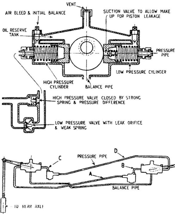
**Figure 1.3.13** The German Stabilus damping system for commercial vehicles. Actuation was by the central eccentric circular cam, driven by a drop arm to each wheel. The two plugs at the top of each unit allow independent adjustment of bump and rebound forces. This forms a conventional independent system of unusual actuation. In addition, the two sides of an axle are interconnected through a balance pipe and by relief valves effective in roll only (asymmetrical action).
