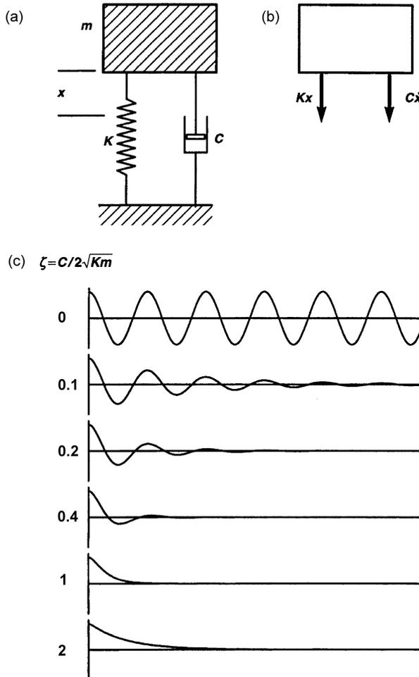
**Figure 2.3.1** Basic linearly-damped 1-dof system: (a) definition sketch; (b) free body diagram; (c) free vibration of system with linear damping for various damping ratios  $\zeta$ .
