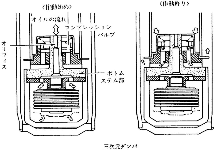
**Figure 6.20.1** Foot valve with bellows: (a) the bellows contracts to accommodate a limited volume of fluid from the extension chamber in the bellows chamber, or vice versa; (b) at higher pressure or longer stroke the parallel shim valve operates normally. Reproduced from Komamura and Mizumukai (1987) *History of Shock Absorbers*, *JSAE*, 41(1), pp. 126–131.
