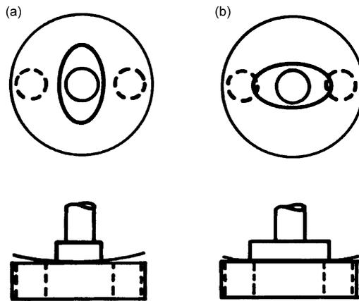
**Figure 8.7.1** Variable stiffness valve by rotating a cam, changing the length of the shim cantilever: (a) soft position; (b) hard position.
