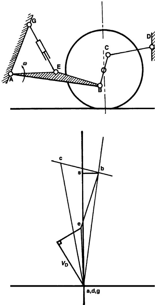
Figure 4.16.1 Axle with link location.
