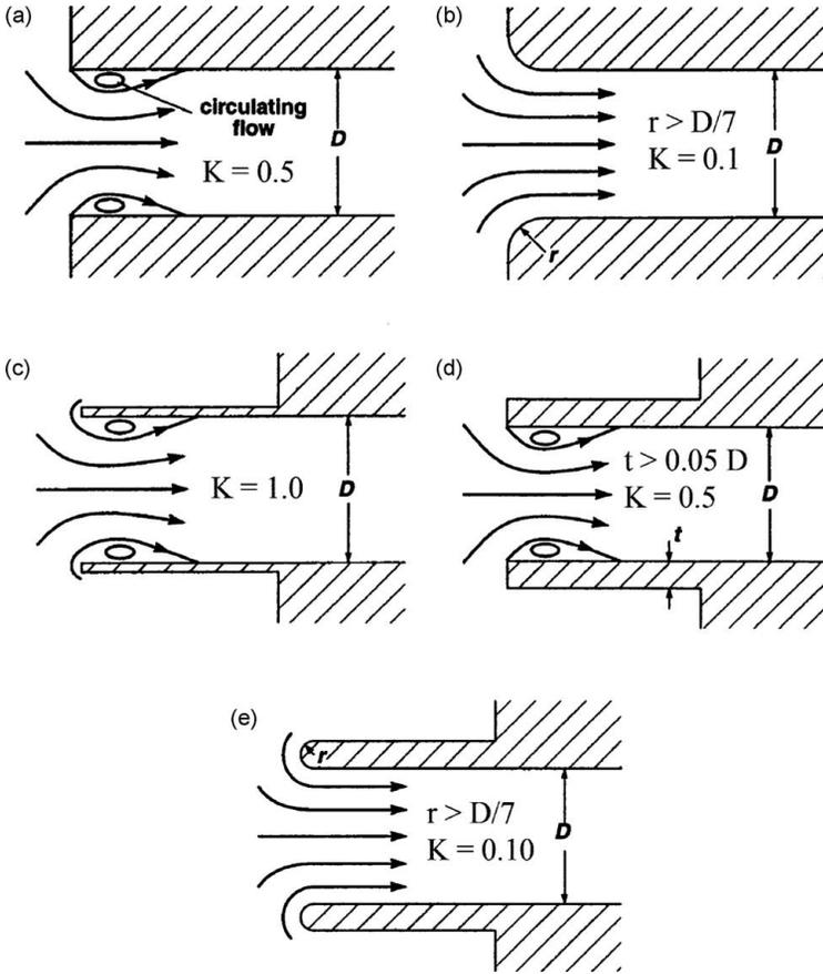
**Figure 5.21.1** Entry losses: (a) Sharp-edged,  $K = 0.5$  (separation), (b) Bell-mouthed,  $r \geq 0.14D$ ,  $K = 0.10$  (no separation), (c) Sharp re-entrant,  $K = 1.0$  (separation), (d) Sharp thick-edged re-entrant,  $t \geq 0.05D$ ,  $K = 0.5$  (separation as in (a)), (e) Rounded re-entrant,  $r \geq 0.14D$ ,  $K = 0.10$  (no separation).
