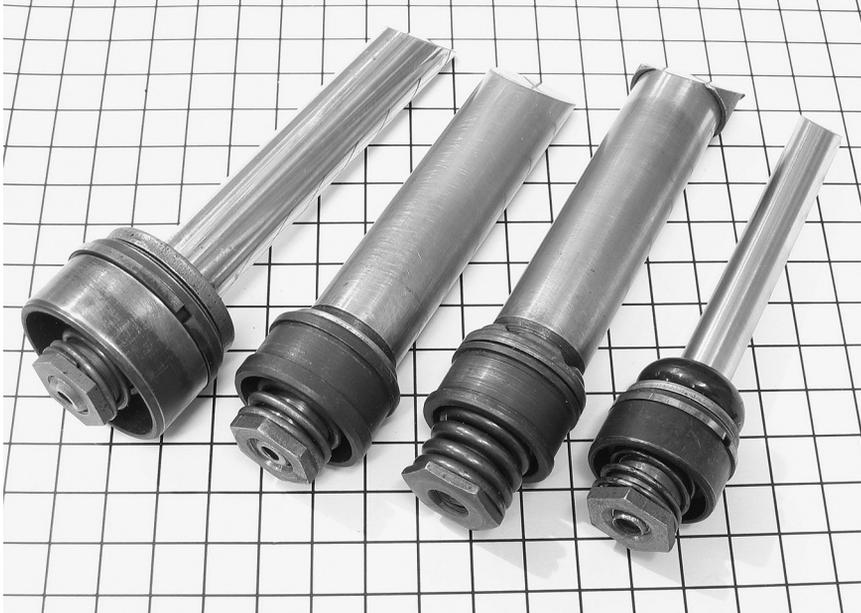
**Plate 3.01** Piston Valves 1. Four example pistons of traditional configuration., with simple star-shim controlled compression valves (not visible) and coil-spring controlled extension valves. The first and fourth exhibit cast iron piston rings. Piston and rod diameters are (1) 35.0/15.8, (2) 28.3/20.0., (3) 26.6/20.0, (4) 25.4/10.8 mm. The large rod/piston diameter ratios shown by the centre two reveal them as from struts. Wear patterns are visible on the first piston.
