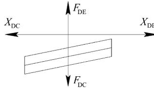
**Figure 7.4.1** The force loop for creeping motion reveals the gas pressure force and friction forces only.
