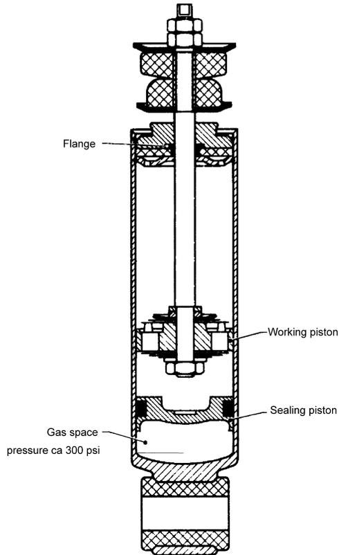
**Figure 1.3.16** DeCarbon type of telescopic damper with floating secondary ('sealing') piston and high pressure in the gas chamber. The secondary piston must have sufficient free movement to accommodate the rod displacement volume and oil thermal expansion. A disadvantage is that the main rod seal is continuously subject to high pressure so good manufacturing quality is required to prevent long-term leakage. Also, in some applications (off road), the single tube is prone to damage.
