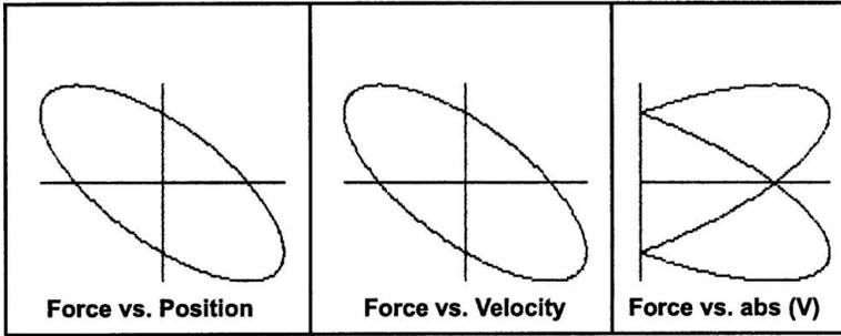
Figure 7.12.3  $F(X)$ ,  $F(V)$  and  $F(\text{abs}(V))$  for a sinusoidal test. Force type:  $-0.5(kx + cV)$  (linear spring + damper).
