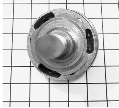
**Plate 3.05** Piston Valves 5. A different shim-pack piston seen from the rod (expansion chamber) side. Again, triangulation of the bottom shim has been used. This also facilitates three-wing bending. Six active shims in uniform diametral steps.
