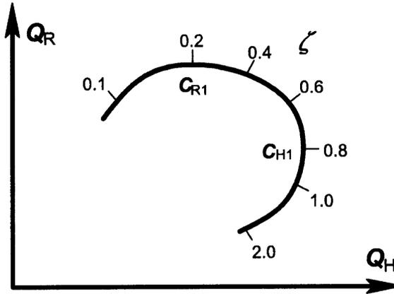
Figure 3.11.3 The ride-handling quality loop with varying damping.
