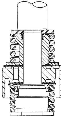
**Figure 6.3.2** Piston with coil-spring disc valves for both compression and extension.
