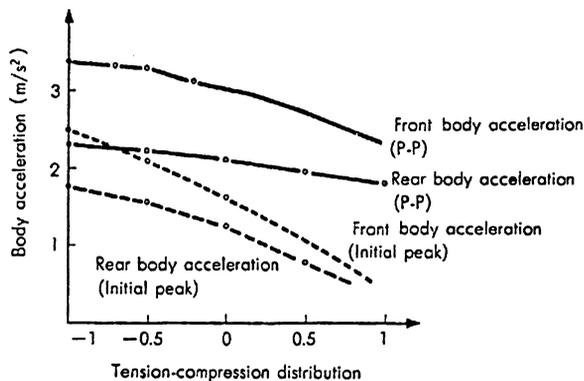
**Figure 3.13.3** The effect of damper force transfer factor  $e_D$  on vehicle body vertical acceleration when driving over a solitary positive bump, simulation results. Reproduced from Fukushima, Hidaka and Iwata (1983) Optimum characteristics of automotive shock absorbers under various driving conditions and road surfaces, *JSAE Review*, pp.62–69.
