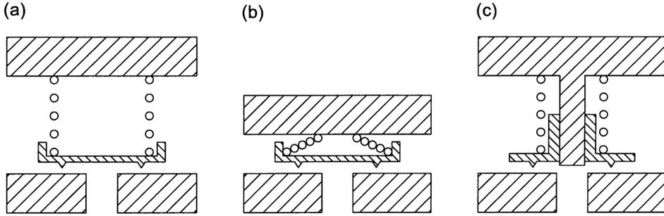
**Figure 6.3.1** Disc valves: (a) disc with coil spring; (b) with spiral spring (when free); (c) guided disc with coil spring.
