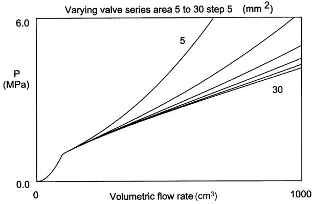
Figure 8.2.3 Effect of adjustment to series area.
