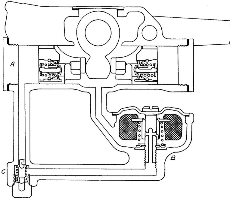
Figure 6.13.1 Inertial valve for opposed-piston damper (Kindl, 1933).
