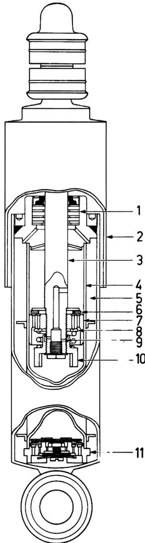
**Figure 1.3.18** A double-tube damper showing various features. 1 seal; 2 shroud; 3 rod; 4 inner cylinder; 5 annular foot and gas chambers; 6 piston compression valve; 7 piston; 8 extension valve; 9 parallel hole feed; 10 adjuster; 11 foot valve. The adjuster screws along the rod compressing the valve preload spring. This is achieved by fully compressing the damper to engage the adjuster in the bottom of the cylinder, and rotating the two body parts (Koni).
