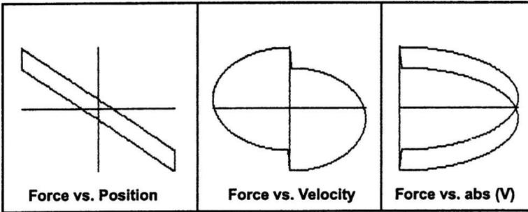
Figure 7.12.6  $F(X)$ ,  $F(V)$  and  $F(\text{abs}(V))$  for a sinusoidal test. Force type: linear spring + Coulomb friction.
