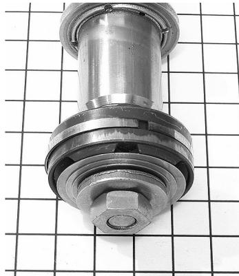
**Plate 3.06** Piston Valves 6. A third shim-pack piston showing the compression chamber side. Counter-flow is achieved in this case by the angled perimeter face. Three shims with spacer and rigid backing washer.
