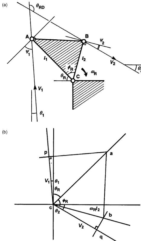
**Figure 4.9.1** General rocker configuration; (a) geometry, (b): velocity diagram.
