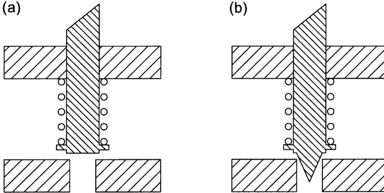
Figure 6.4.1 Rod valves: (a) basic flat-ended; (b) tapered.
