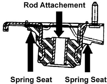
Figure 1.7.12 Dual-path damper/strut mounting (Lewitske and Lee, 2001).
