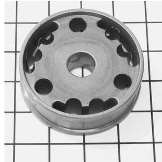
**Plate 5.10** Piston 5, extension valve side. Three holes for extension flow controlled by the shims on this side. Again, triangulated shims are required to facilitate counter-flow.
