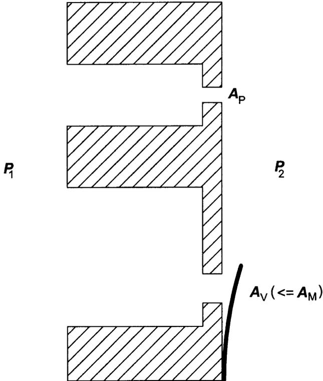
**Figure 6.9.3** Basic valve model.
