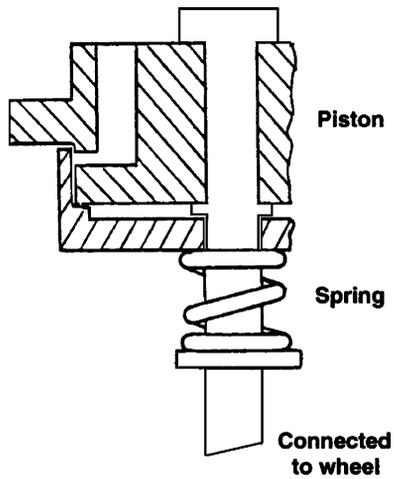
Figure 6.13.2 Inertial valve (from Speckhart and Harrison, 1968, modified for clarity of function).
