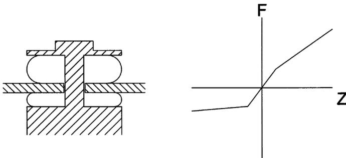
Figure 1.7.6 Asymmetrical type of damper or strut bushing.
