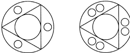
**Figure 6.6.3** Shim valve flow hole positions as typically used for three-wing bending mode.
