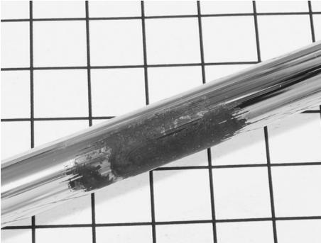
**Plate 8.07** Severe wear on a damper rod, resulting in complete removal of the chromium plating, of inadequate thickness for the in-service side load.
