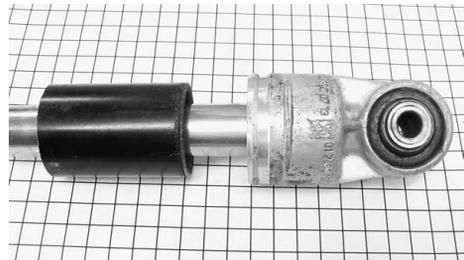
**Plate 2.05** Header 5. Cast aluminium header unit incorporating ball joint connector.
