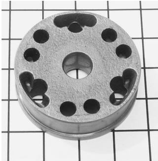
**Plate 5.09** Piston 5, compression valve side. Basically a flat surface, with six holes for compression flow controlled by the shims on this side. The more complex holes are for extension flow down. The flat surface requires a triangulated bottom shim to clear the extension flow holes.
