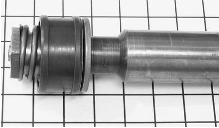
**Plate 3.03** Piston Valves 3. A strut piston and rod, somewhat unusual in using a diametral reduction above the piston. Piston diameter 25 mm, rod 17.0 and 12.2 mm. Conventional compression star-shim and extension coil spring.
