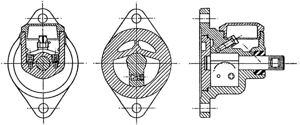
Figure 1.3.2 Early vane-type damper (Kinchin and Stock, 1951/1952).
