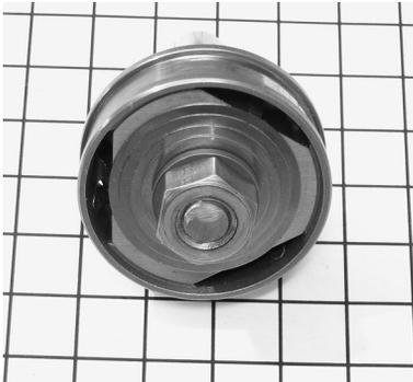
**Plate 3.04** Piston Valves 4. A shim-pack piston seen from the compression chamber side. The sealing shim is triangulated to allow free flow through this pack during compression. Five shims and a rigid washer.
