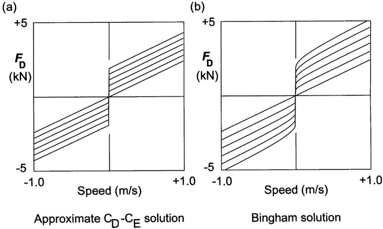
**Figure 9.4.2** Theoretical characteristics of an example design of ER damper: (a) approximate CD–CE solution; (b) Bingham flow solution.
