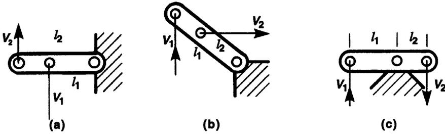
Figure 4.9.2 Simple rockers with various deflection angles.
