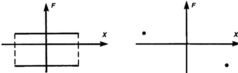
**Figure 11.9.2**  $F(X)$  and  $F(V)$  curves for an ideal bilinear damper subject to idealised triangular waveform displacement.
