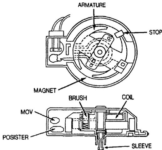
**Figure 6.19.1** Solenoid actuator for adjustable barrel valve (Soltis, 1987).
