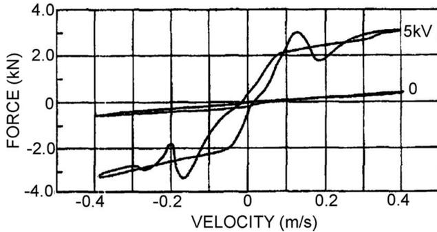
Figure 9.3.3 Stick-slip phenomenon of ER liquid (Petek *et al.*, 1995).
