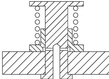
Figure 6.5.1 Spool valve variation with slider.
