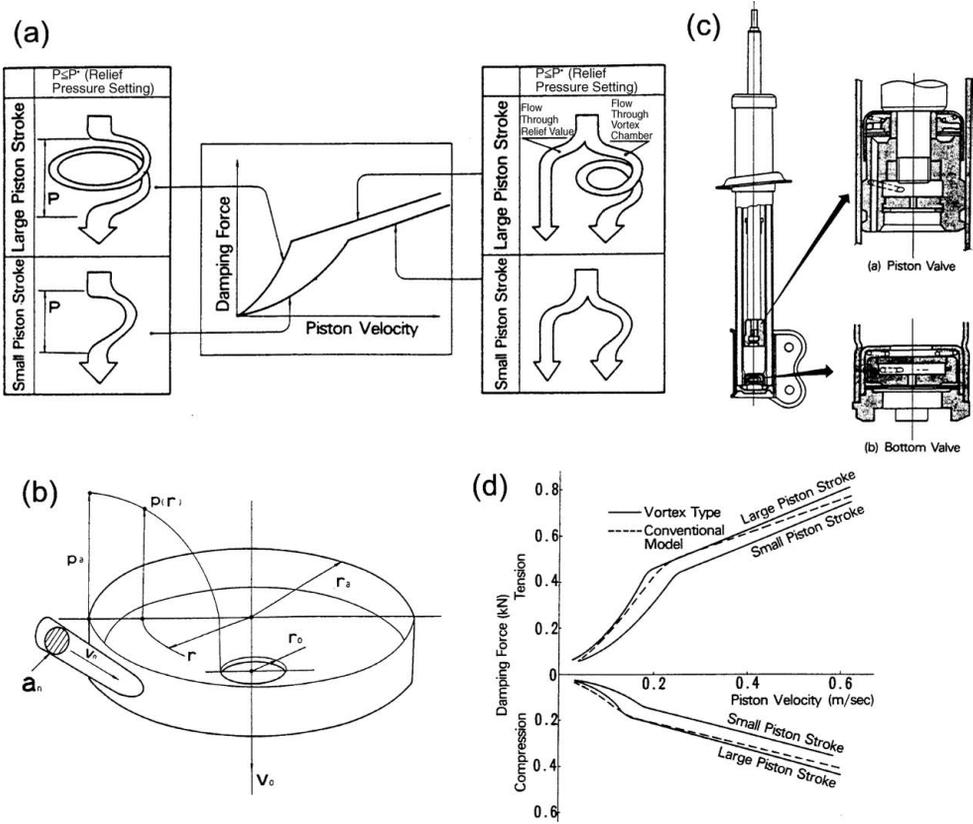
**Figure 6.16.2** Vortex valve for stroke sensitive damping: (a) vortex effect on resistance pressure; (b) vortex chamber geometry; (c) damper structure; (d) experimental damper characteristics. Reproduced from Fukushima, Idia and Hidaka (1984) Development of an automotive shock absorber that improves riding comfort without impairing steering stability, *Proc. 20th FISITA Conference*, pp. 218–223.
