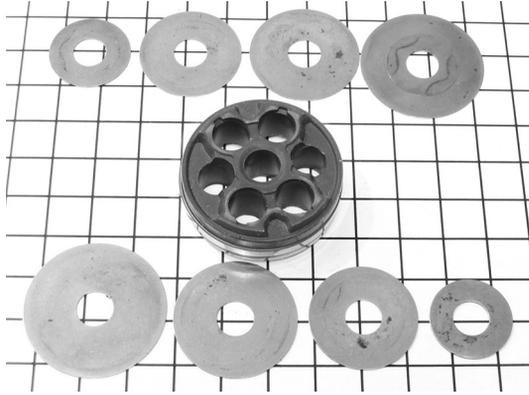
**Plate 6.04** Piston Valve Set 4. A 2/4 shim-pack piston shown compression side up, with four compression holes and two extension holes, with, top and bottom rows. The compression shims are  $30.6 \times 0.40$ ,  $28.0 \times 0.30$ ,  $25.0 \times 0.30$ ,  $20.0 \times 0.40$ . The extension shims are  $31.4 \times 0.40$ ,  $27.0 \times 0.40$ ,  $24.0 \times 0.4$  and  $18.5 \times 0.60$ .
