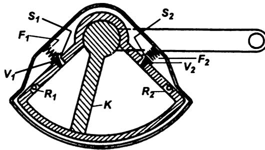
Figure 1.3.1 Double-acting vane type damper (Fuchs, 1933).
