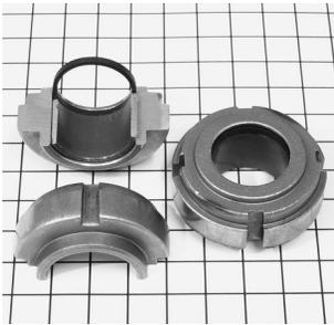
**Plate 2.02** Header 2. Sectioned at left, complete unit at the right. The bearing material insert and the seal are visible. The protruding lower ring fits into the pressure tube.
