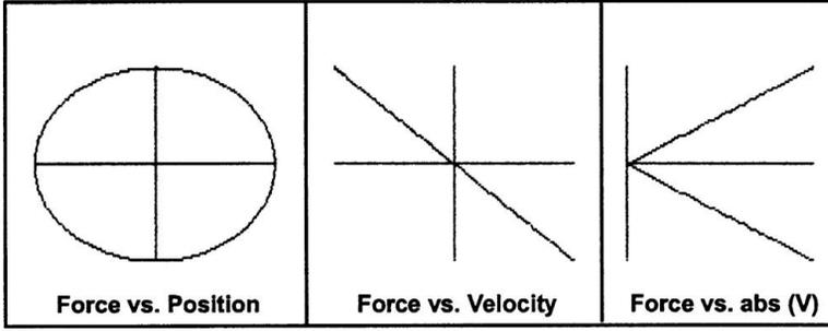
Figure 7.12.2  $F(X)$ ,  $F(V)$  and  $F(\text{abs}(V))$  for a sinusoidal test. Force type:  $-kV$  (linear damper).
