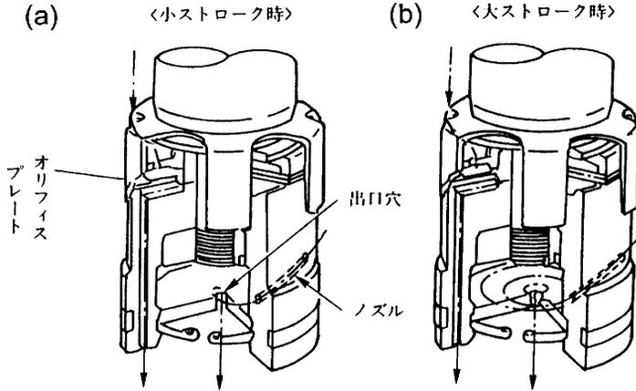
**Figure 6.16.3** Vortex valve: (a) short stroke radial flow; (b) long stroke spiral flow. Reproduced from Komamura and Mizumukai (1987) History of Shock Absorbers, *JSAE*, 41(1), pp. 126–131.
