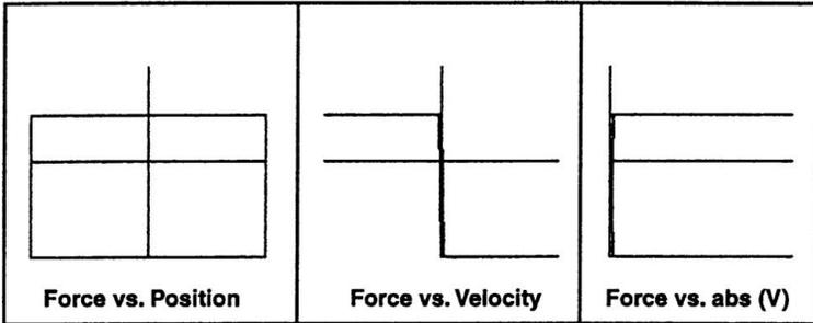
Figure 7.12.11  $F(X)$ ,  $F(V)$  and  $F(\text{abs}(V))$  for a sinusoidal test. Force type: asymmetrical blow-off valves.
