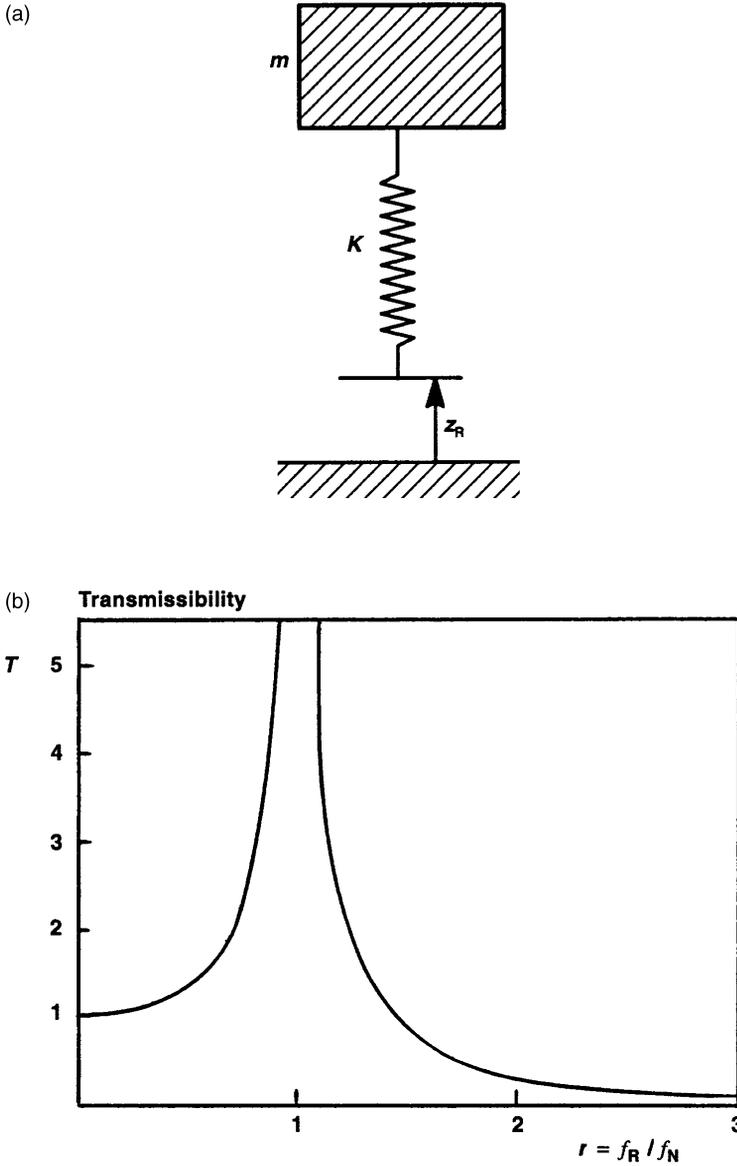
**Figure 2.4.1** (a) Undamped 1-dof model vehicle stimulated by road displacement, (b) Transmissibility of an undamped 1-dof suspension.
