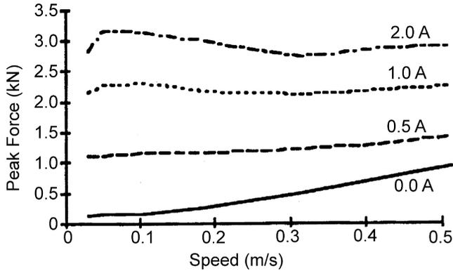
**Figure 9.6.1** Controllable MR damper force versus extension speed, illustrating the effect of field on the effective Bingham parameters yield stress and marginal viscosity (Weiss *et al.*, 1993).
