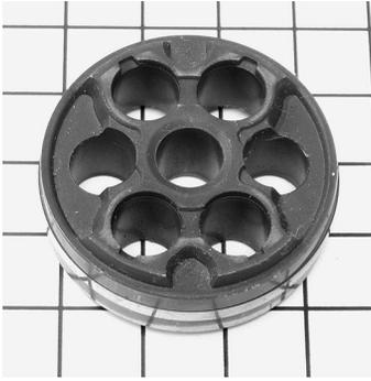
**Plate 5.07** Piston 4, compression valve side. A 2/4 hole shim-pack type piston with four holes for compression flow, up into the raised area. The other two holes, from the lower area below shim level, on the left and right, are for downward extension flow.
