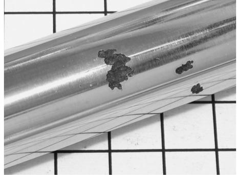
**Plate 8.09** Bad pitting corrosion of a chromium-plated rod, probably caused by inadequate rod preparation before plating, with consequent poor adhesion of the chromium.
