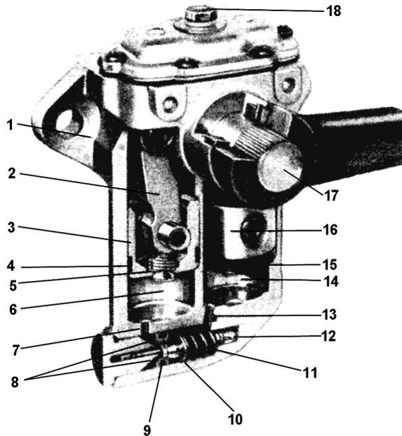
**Figure 1.1.18** The double parallel-piston damper was the ultimate lever-arm configuration, overcoming the problems of the vane lever-arm type (Lucas) (see also Figure 1.3.7).
