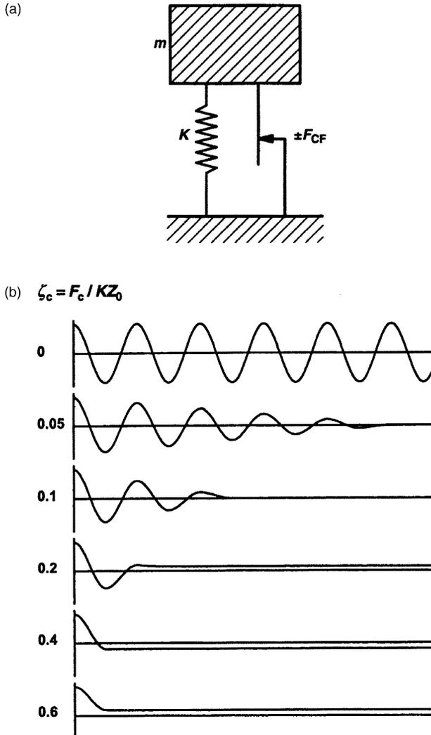
**Figure 2.6.1** (a) Definition sketch of 1-dof vibration model with Coulomb friction; (b) free vibration of system with Coulomb friction damping.
