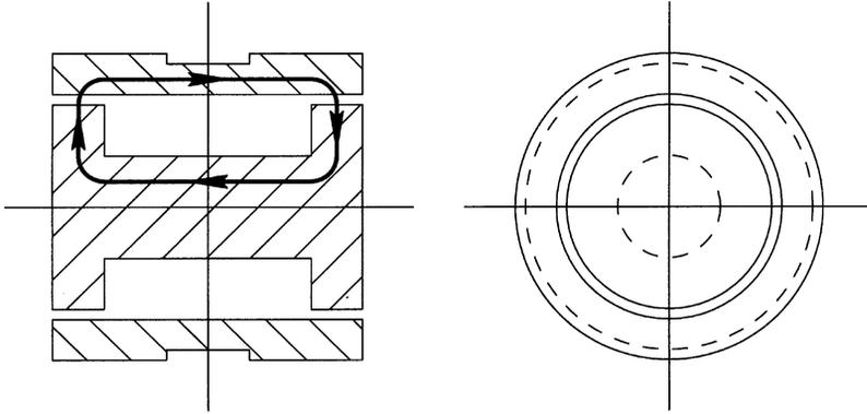
**Figure 9.7.2** Magnetic circuit in an MR damper piston.
