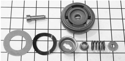
**Plate 7.03** Foot Valve Set 3. Top row: pin with axial hole and also cross-drilling (hardly visible), and body, extension valve side up. Bottom row: extension valve sealing shim, curved shim spring, locating pressing, sleeve seal, spring for sleeve seal, retaining washer (peened on). The lower left three parts fit on top of the piston as shown, held by the pin head. On the compression valve side, the sleeve slides on the pin, opening against the coil spring.
