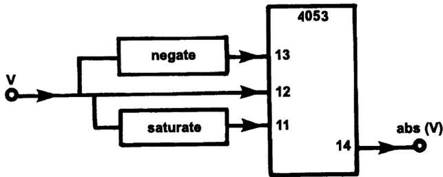
**Figure 11.6.2** Velocity signal rectification using a multiplexer chip.
