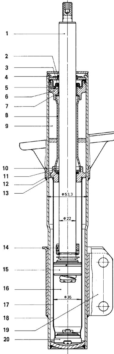
**Figure 1.3.21** Sectional view of a front strut for a larger car. Piston diameter 36 mm, rod diameter 22 mm. 1 rod; 2 seal; 3 bush; 4 rolled closure; 5 bush; 6 top moulding; 7 bearing bush; 8 sleeve; 9 gas chamber; 11 centre moulding; 12 hole; 13 seal; 14 impact guard; 15 piston; 16 compression chamber; 17 inner (working) cylinder; 18 annular foot chamber; 19 wheel hub fixture; 20 foot valve (Boge).
