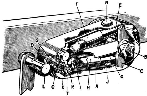
**Figure 1.1.21** The Armstrong 'double telescopic lever arm' damper.
