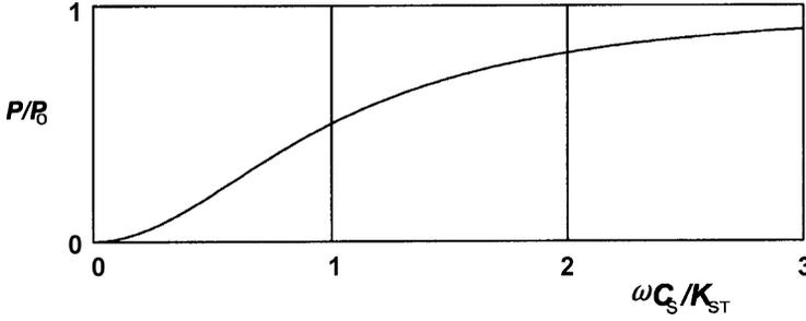
**Figure 2.8.2** Variation of system power dissipation with frequency, with a series spring.
