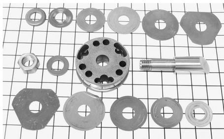
**Plate 6.06** Piston Valve Set 6. Centre row: retaining nut, washer, piston compression valve side up, and rod. Top row: compression shims, triangulated sealing shim with conventional sequence of reducing diameter support shims and washer, 0.20, 0.25, 0.25, 0.30, 0.35 mm thickness largest to smallest. Bottom row: similar shims for extension, 0.30, 0.30, 0.35, 0.45 and 0.50 mm thickness largest to smallest.
