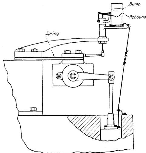
**Figure 11.3.1** Early tester shown with a rotary vane damper (James and Ullery, 1932).
