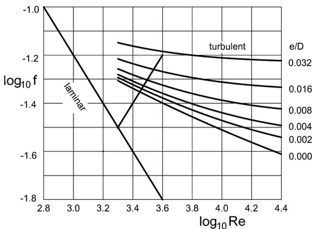
**Figure 5.19.2** The Colebrook Diagram for pipe friction factor  $f$  (Moody diagram using Colebrook's equation).
