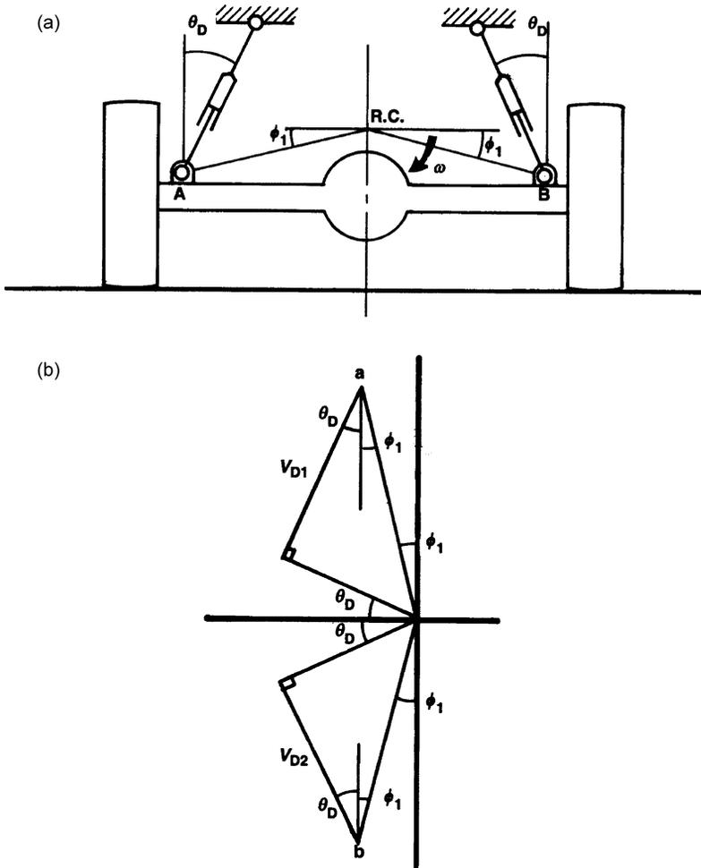
**Figure 4.16.2** Inclined dampers on an axle, for axle sway vibration damping: (a) rear view; (b) velocity diagram.
