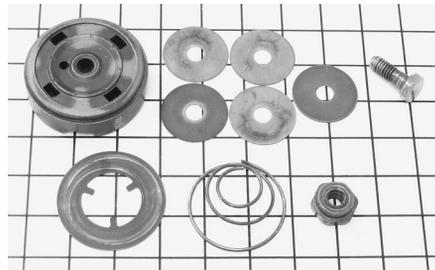
**Plate 7.04** Foot Valve Set 4. Top row: foot valve body, shown extension valve side up, five extension valve shims to fit underneath and retaining screw. Bottom row: extension valve sealing shim with internal clearance for compression flow and locating points, conical spring, retaining sleeve nut, which locates the spring and the shim on its sleeve length, shown inverted.
