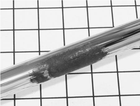
**Plate 8.07** Severe wear on a damper rod, resulting in complete removal of the chromium plating, of inadequate thickness for the in-service side load.
