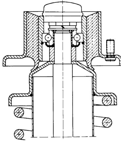
Figure 1.7.8 Strut top mounting (INA).
