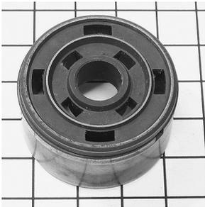
**Plate 5.05** Piston 3, compression valve side. The standard operating principle, four holes in each direction.
