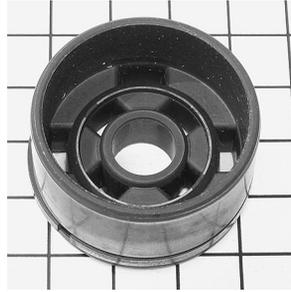
**Plate 5.06** Piston 3, extension valve side.
