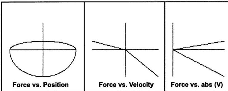
Figure 7.12.9  $F(X)$ ,  $F(V)$  and  $F(\text{abs}(V))$  for a sinusoidal test. Force type: bilinear damper (25/75).
