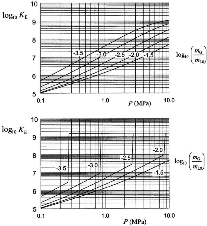
Figure 5.15.3 The bulk modulus of oil/air emulsion: (a) without absorption; (b) with absorption.
