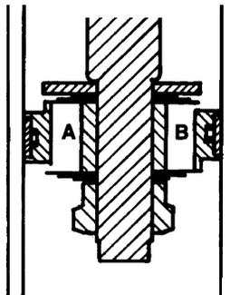
**Figure 6.6.1** Complete double-acting shim valve as used in practice.
