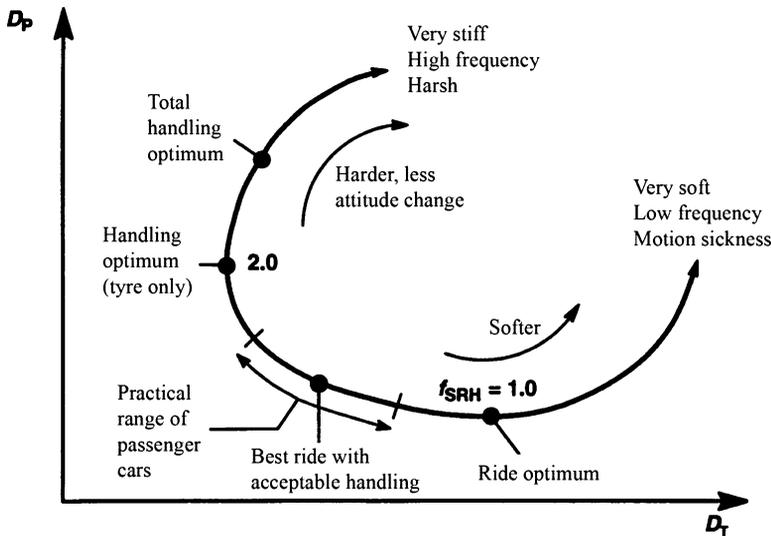
Figure 3.11.6 The passenger-tyre discomfort loop.
