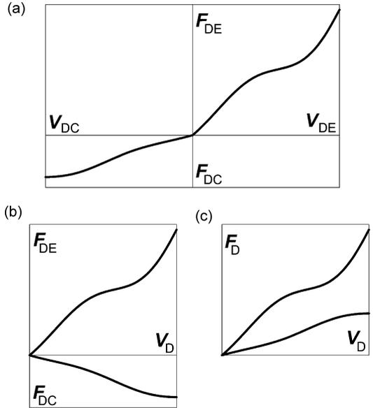
**Figure 7.1.2** Damper characteristics: (a) force vs velocity; (b) force vs absolute velocity; (c) absolute force vs absolute velocity.
