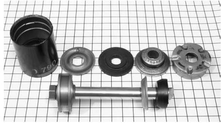
**Plate 2.04** Header 4. This header unit is for a pressurised single-tube damper, requiring elaborate sealing for reasonable life. The various parts of the head bearing and seal are held in the main tube by circlips, visible in the tube at top left.
