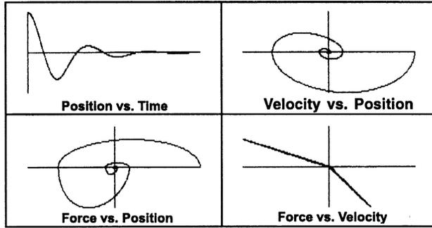
**Figure 11.2.6** Natural vibration of spring + mass + damper from  $X = X_0, V = 0$ . Friction type is asymmetrical linear (bilinear).
