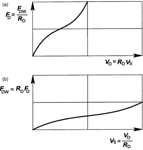
**Figure 4.7.1** Damper forces with motion ratio: (a) at the damper; (b) at the wheel.
