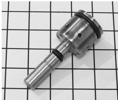
**Plate 8.05** Barrel from an adjustable damper. Rotation of the barrel brings one of six holes into registration with the body flow channel.
