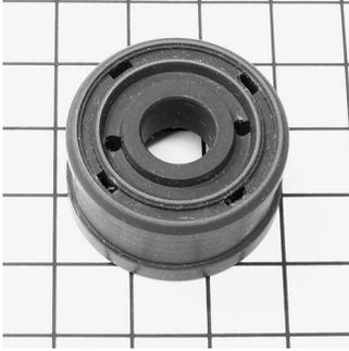
**Plate 5.01** Piston 1, compression valve side. Compression flow is up and out of the four holes in the outer annulus. This is sealed by a shim, with holes in its inner part to allow flow inwards over the inner rim during compression, and also down during extension to pass through the two holes in the inner annulus.
