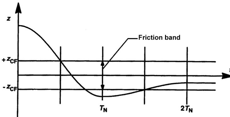
Figure 2.6.2 Free response with Coulomb friction.
