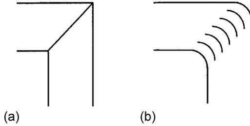
Figure 5.21.3 (a) Sharp-corner losses; (b) ameliorated by a faired bend with vanes.
