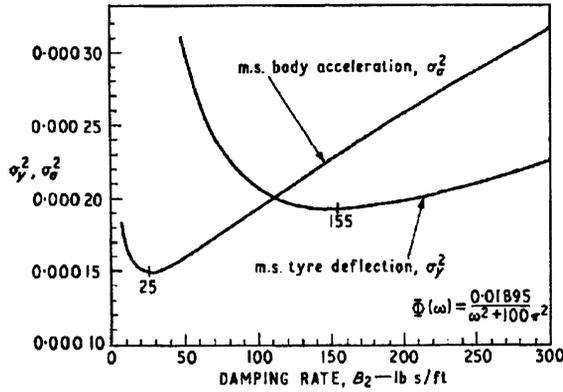
Figure 3.11.5 Body acceleration and tyre deflection variation against damping coefficient as seen at the wheel (Thompson, 1969).
