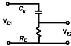
Figure 11.6.1 Differentiation circuit.
