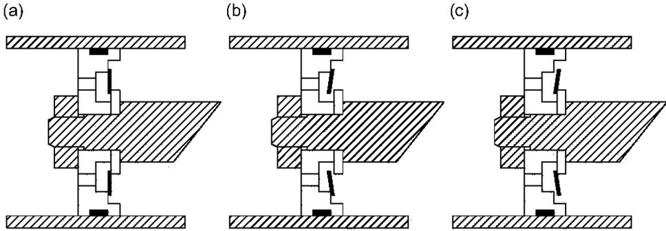
**Figure 6.18.1** Example configuration of a double-acting shim valve, showing: (a) closed; (b) extension flow opening; (c) compression flow opening. Radial location of the shim is required at three points, not shown.
