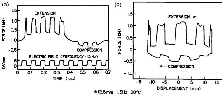
**Figure 9.4.3** Laboratory tests of an ER damper with square-wave control voltage applied: (a) force vs time; (b) force vs position (Petek, 1992a,b,c).
