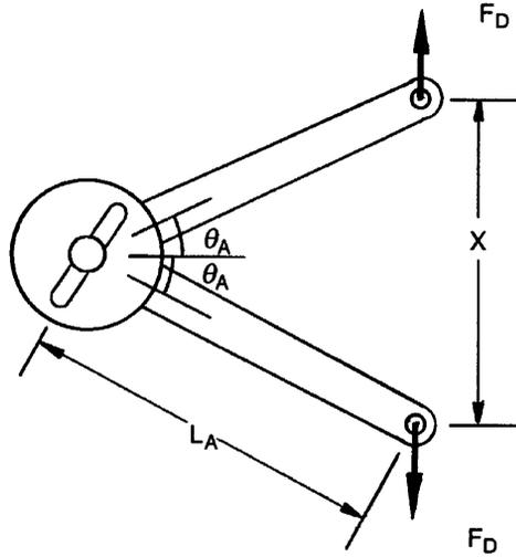
Figure 4.17.1 Geometry of the scissor-type snubber.
