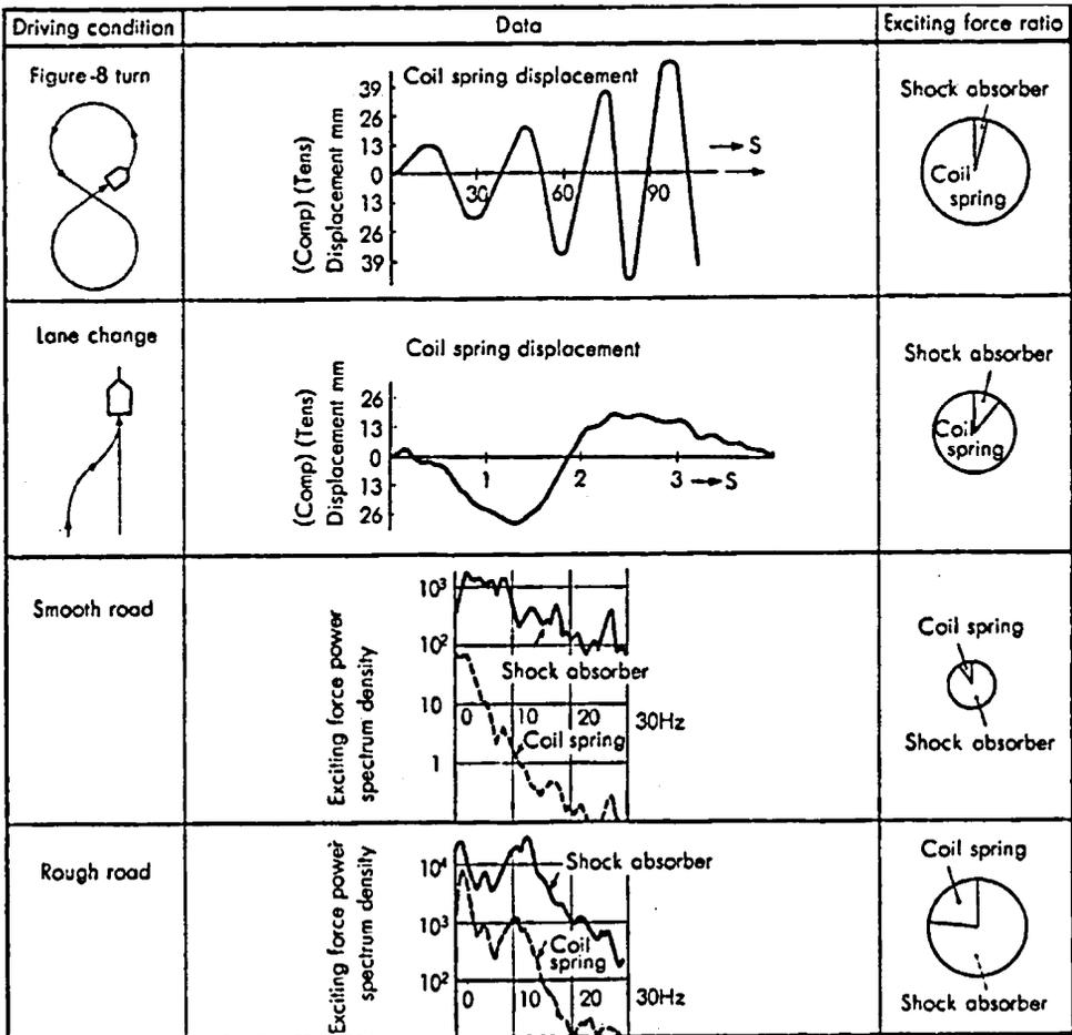
**Figure 3.12.1** Optimum damper characteristics under various driving conditions and road surfaces; (a) figure-8 turns at increasing speed; (b) lane change; (c) straight driving on a smooth road; (d) straight driving on a rough road. Reproduced from Fukushima, Hidaka and Iwata (1983) Optimum characteristics of automotive shock absorbers under various driving conditions and road surfaces, *JSAE Review*, pp.62–69.
