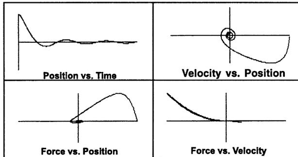
**Figure 11.2.4** Natural vibration of spring + mass + damper from  $X = X_0, V = 0$ . Friction type is quadratic symmetrical.
