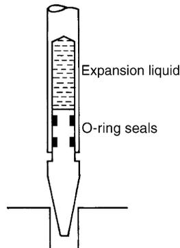
**Figure 6.11.3** Liquid expansion method of temperature compensation.
