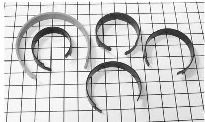
**Plate 8.04** A selection of plastic piston rings, typically graphite-loaded PTFE. Cast iron, Tufnol and other materials have also been used.
