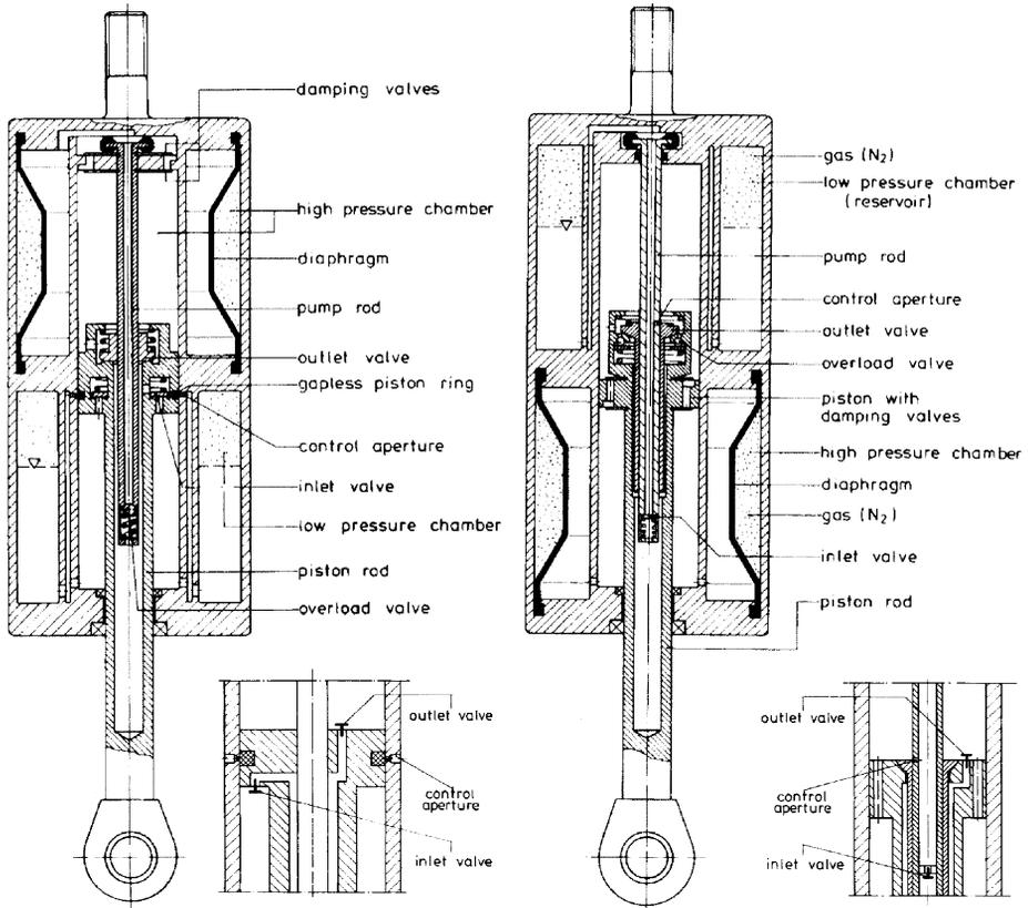
Figure 1.4.3 Boge Hydromat (left) and Nivomat (right) height-adjusting dampers.
