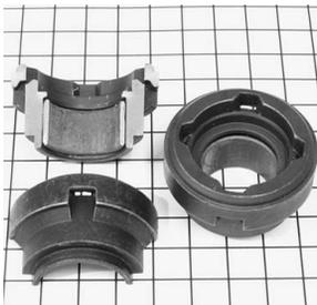
**Plate 2.03** Header 3. Sectioned at the left, complete at the right. A separate seal is used in this case. The bearing material insert is visible. The section shows two leakage return channels, of a total of four visible at the right and one on the bottom left.
