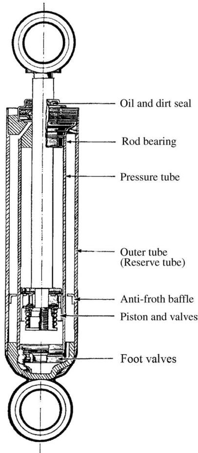
**Figure 1.1.22** Cross-section of a typical telescopic damper showing the general features, shown without the dust shroud (Woodhead–Monroe).
