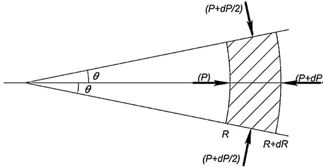
**Figure 5.24.3** An element of a free vortex, a sector of an annulus.
