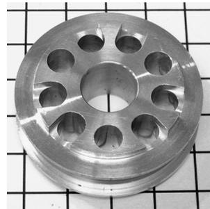
**Plate 5.12** Piston 6, extension valve side. Three holes for extension flow into the shim pack on this side. Six holes with side notches for downward compression flow.
