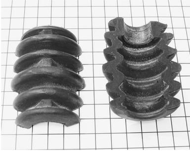
**Plate 8.01** Sectioned rubber bump stop from a strut, in perfect condition after 10 years in service. 63 g.
