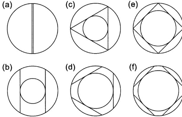
**Figure 6.6.2** Shim valve bending modes.
