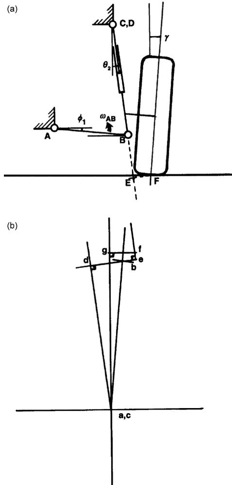
**Figure 4.12.1** Strut suspension: (a) position diagram; (b) velocity diagram.
