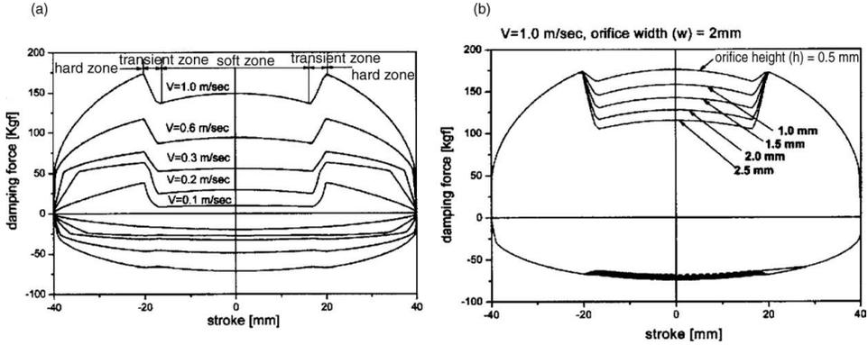
**Figure 6.12.4** Grooved cylinder damper  $F(X)$  force loops: (a) various speeds; (b) various groove depths (Lee and Moon, 2005).
