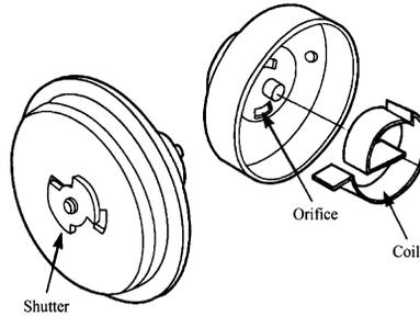
**Figure 6.11.2** Single spiral bimetallic strip operating a rotary shutter. Reproduced from *Design News* 10-2-89, p. 195.
