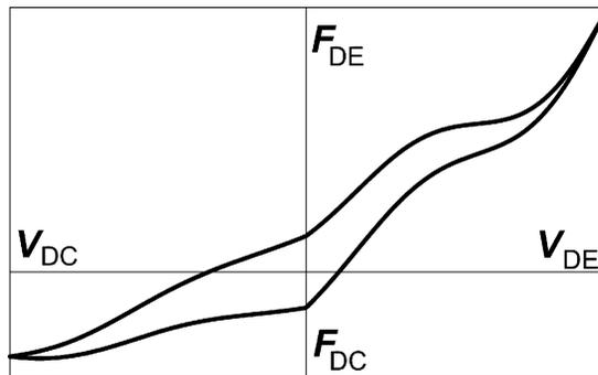
**Figure 7.1.3** Example damper  $F(V)$  loop resulting from stiffness.
