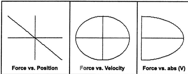
Figure 7.12.1  $F(X)$ ,  $F(V)$  and  $F(\text{abs}(V))$  for a sinusoidal test. Force type:  $-kx$  (linear spring).
