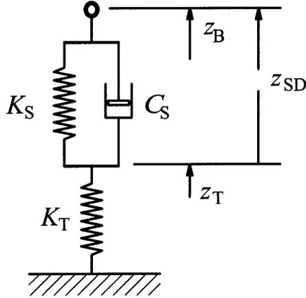
Figure 2.8.1 Suspension system  $K_S C_S$  with series spring  $K_T$ .
