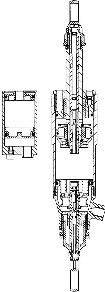
**Figure 11.11.1** This cross-section of a Penske racing damper shows the complexity of the modern hydraulic damper, with associated cost for precision manufacture. Features visible here include the remote reservoir on the right, with free-floating piston, adjustable spindle within the rod, and O-ring sealed assembly to permit easy rebuilding to achieve altered characteristics (by permission of Penske racing Shocks).
