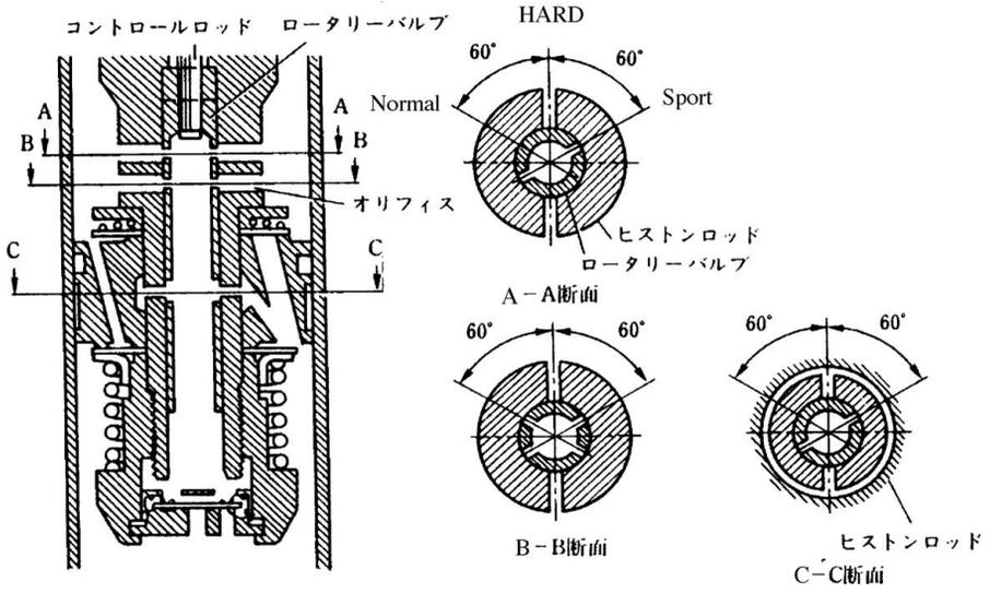
Figure 6.19.3 Rotary adjustable valve. Reproduced from Komamura and Mizumukai (1987) History of Shock Absorbers, *JSAE*, 41(1), pp. 126–131.
