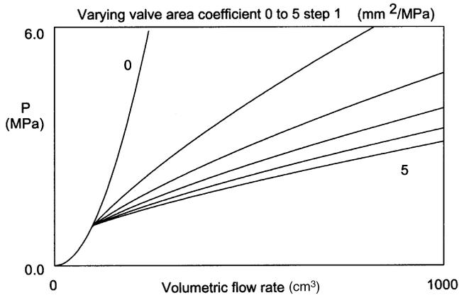
**Figure 8.2.6** Effect of adjustment to area coefficient.
