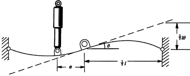
Figure 3.9.1 Axle pitch displacement with longitudinal leaf springs.
