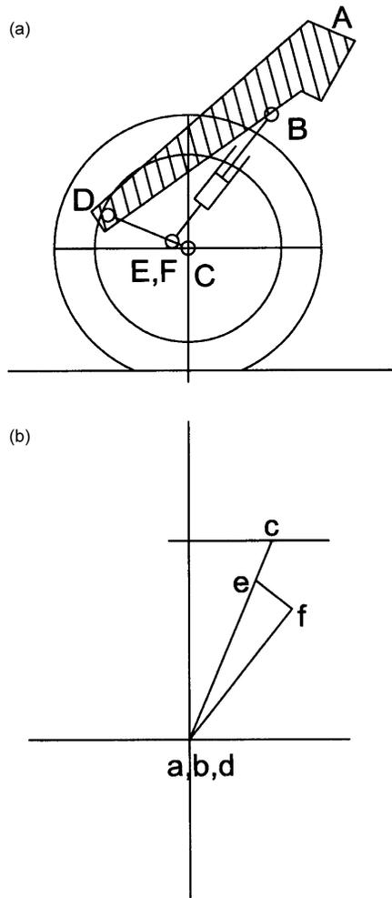
**Figure 4.14.2** Motorcycle front trailing link: (a) position diagram; (b) velocity diagram.
