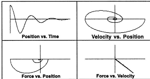
**Figure 11.2.7** Natural vibration of spring + mass + damper from  $X = X_0, V = 0$ . Friction type is unidirectional linear.
