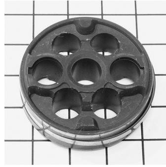
**Plate 5.08** Piston 4, extension valve side. Two holes into the raised area are subject to shim control on this side. Four holes down for compression flow to the other shim pack.
