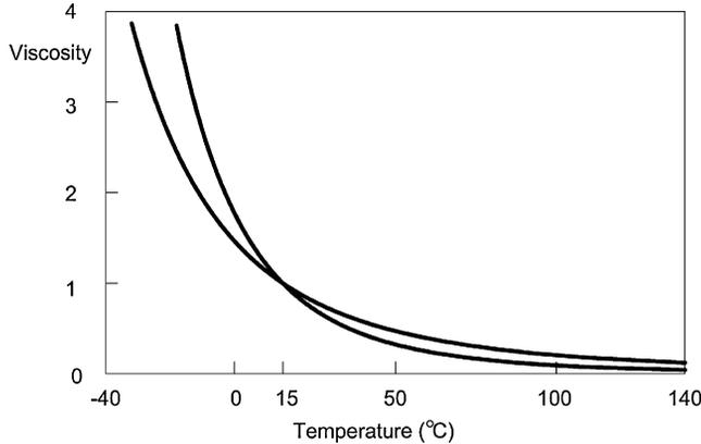
**Figure 5.7.1** Mineral oil viscosity relative to its room-temperature viscosity (viscosity sensitivity  $C = 2000$  and  $3000$  K).
