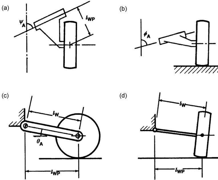
**Figure 4.10.1** Rigid arm suspensions: (a) plan view of semi-trailing arm; (b) rear view of semi-trailing arm; (c) side view of trailing arm; (d) rear view of swing axle.
