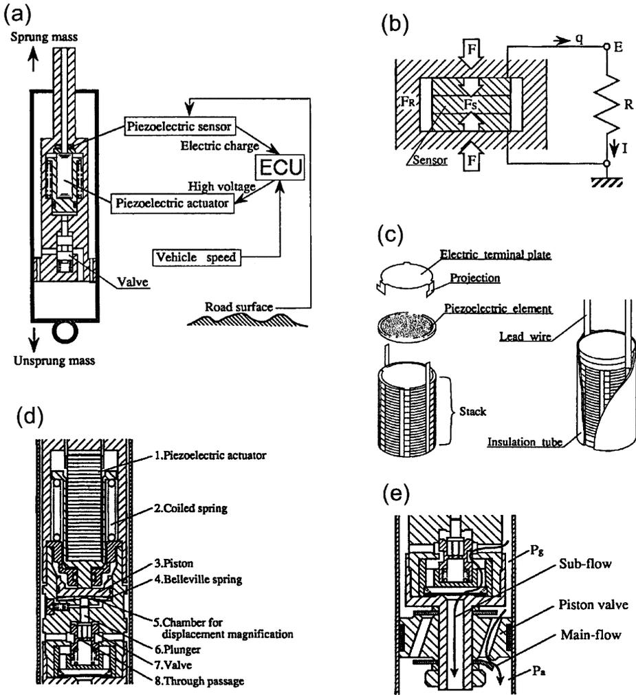
**Figure 6.17.1** Piezoelectric sensing and actuating damper valve: (a) general configuration; (b) piezoelectric sensor; (c) stack of elements; (d) construction of actuator including hydraulic amplification; (e) detail of flow through main valve and controlled supplementary parallel valve (sub-flow) (Shiozaki *et al.*, 1991).
