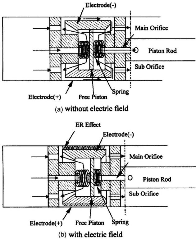
Figure 9.5.2 ER-controlled valve action: (a) field off; (b) field on (Choi, 2003).
