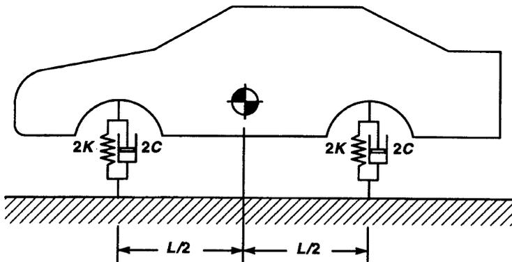
Figure 2.14.1 Vehicle with longitudinal symmetry (with zero damping for section 2.14).
