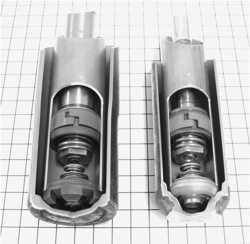
**Plate 1.01** Sectioned dampers from a small-medium family car (US compact). The front strut carries more load and takes side loads, so it is generally more robust, and in particular has a much larger rod diameter.
