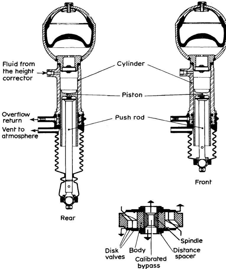
**Figure 1.3.22** Citroen air suspension. The valve, with two shim pack valves, is fixed in position. It is not in the piston, which ideally would pass no oil. The gas is held in the elastomeric rolling seal bag. Nitrogen is used, reducing oxidation ageing of the rubber.
