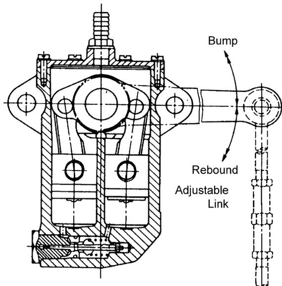
**Figure 1.3.7** The classic lever-arm parallel piston type shown in engineering section, with different valve position. Reproduced from Komamura and Mizumukai (1987) *History of Shock Absorbers*, *JSAE*, 41(1), pp.126–131.
