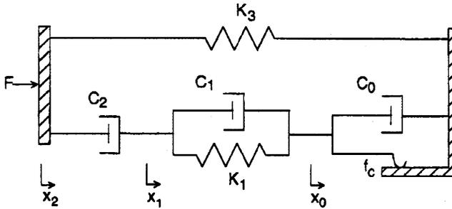
**Figure 9.7.6** Model of complete MR damper. Reproduced with permission from Maranville and Ginder (2003) *Proc. of SPIE*, Vol. 5056, pp.524–533.
