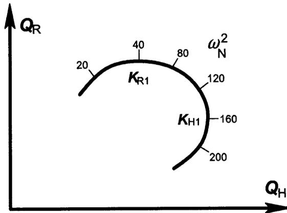
Figure 3.11.2 The ride-handling quality loop with varying stiffness.
