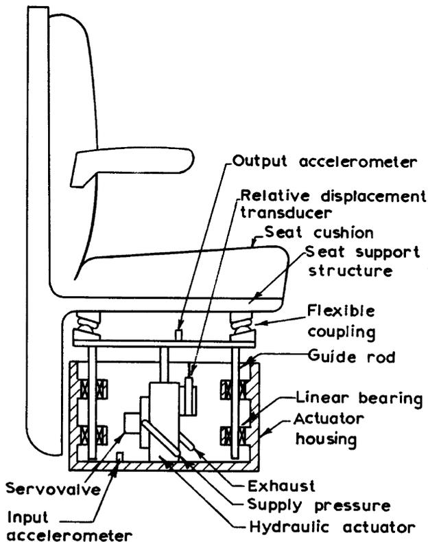
**Figure 3.6.1** Advanced vibration-isolating seat (Calcaterra, 1972, in Hunt, 1979). 3.6.1. Reprinted from *Journal of Sound and Vibration*, 6, Calcaterra, Active vibration isolation for aircraft seating, pp.18–23, Copyright 1972, with permission from Elsevier.
