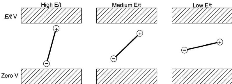
**Figure 9.3.2** Polar particle subject to a varying electric field in constant fluid shear rate.
