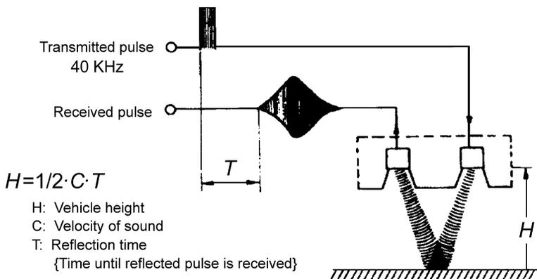
Figure 8.8.2 Ultrasonic height measurement at 40 kHz by detecting the time delay, similar to bats and dolphins (Sugasawa *et al.*, 1985).
