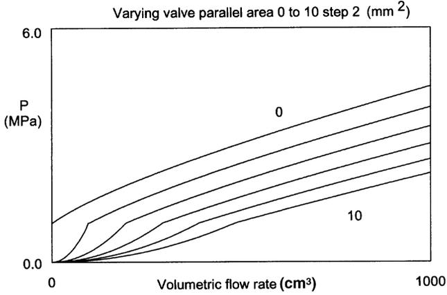
Figure 8.2.2 Effect of adjustment to parallel area.
