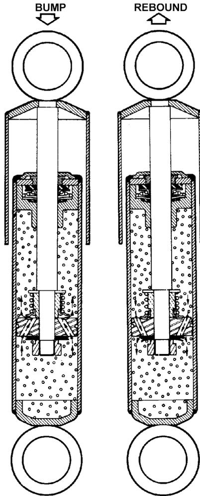
**Figure 1.3.17** To eliminate the free piston, an emulsified oil may be used, distributing the expansion and rod-accommodation volume throughout the main oil volume. Overall length is reduced. On standing, the gas separates, but quickly re-emulsifies on action. The valves must be rated to allow for the passage of emulsion rather than liquid oil (Woodhead).
