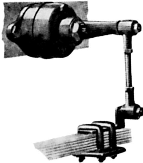
**Figure 1.1.12** The Houdaille rotary vane damper, the first large quantity production hydraulic damper. This originated in 1909 and was double-acting from 1921.
