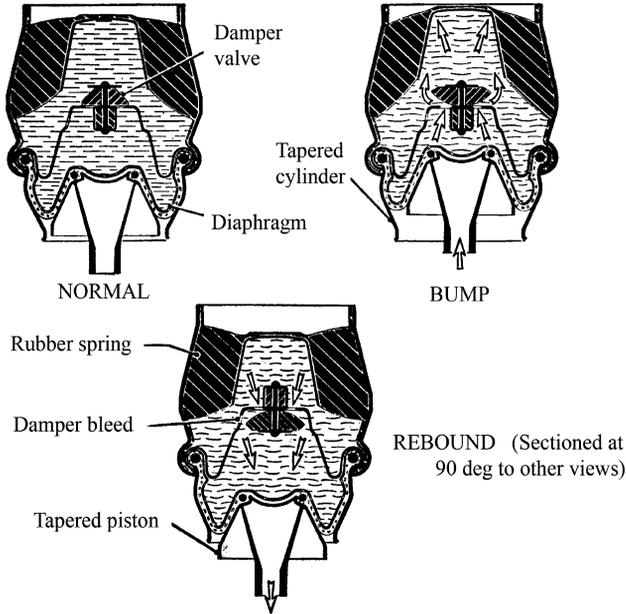
**Figure 1.3.23** The BMC Hydrolastic system had a somewhat similar operation to the Citroen gas system, but replaced the gas spring by a rubber-in-shear spring already well proven. Based on Campbell, C., *Automobile Suspensions*, Chapman and Hall, 1981.
