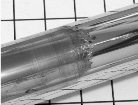
**Plate 8.06** Severe wear on a strut rod after about 10 years in service. The wear has penetrated the hard chromium plating, and there is evidence of consequent corrosion. Strut replacement was required.
