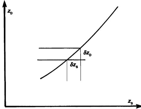
Figure 4.2.1 Damper displacement vs suspension displacement.
