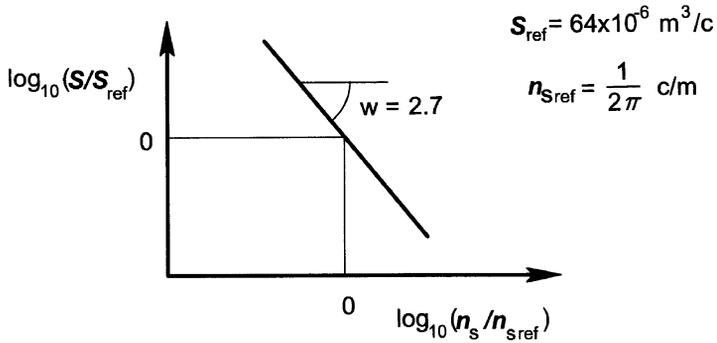
Figure 3.2.2 The basic spectral model of a representative road surface.
