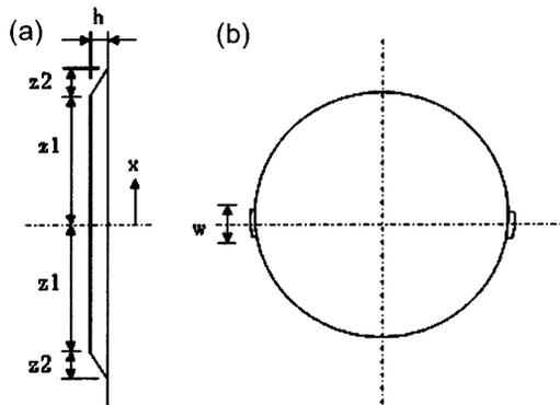
**Figure 6.12.3** Position-sensitive pressure cylinder design: (a) longitudinal groove section; (b) cross-section (Lee and Moon, 2005).
