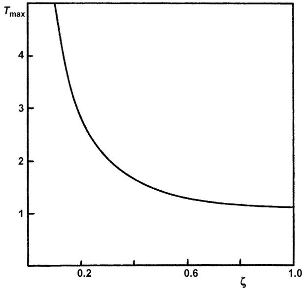
Figure 2.5.2 Peak transmissibility versus damping ratio.
