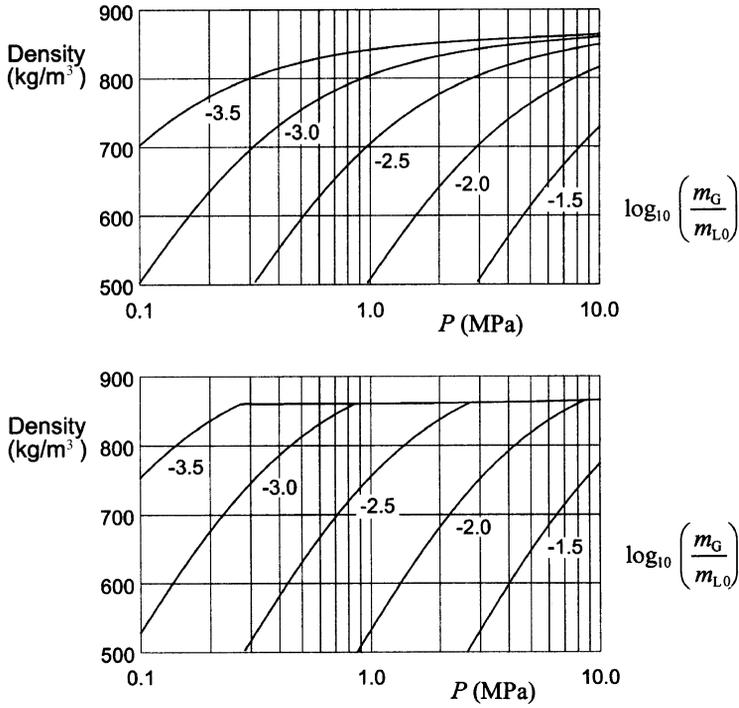
Figure 5.15.2 The mean density of an oil/air emulsion: (a) without absorption; (b) with absorption.
