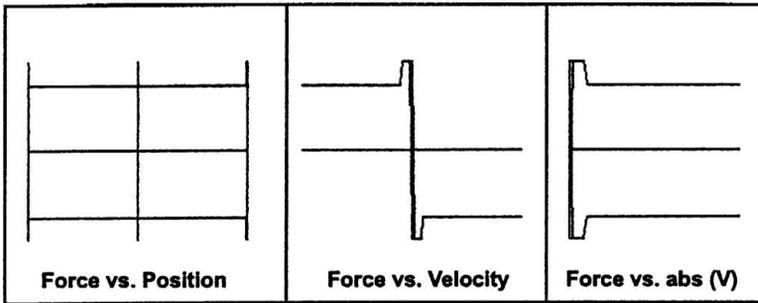
Figure 7.12.5  $F(X)$ ,  $F(V)$  and  $F(\text{abs}(V))$  for a sinusoidal test. Force type: stiction.
