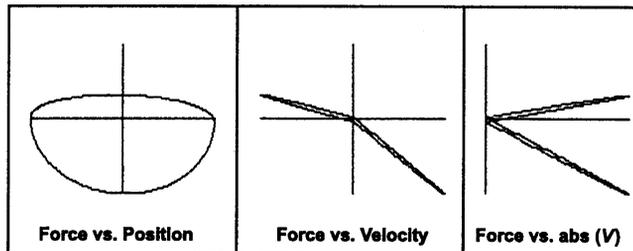
**Figure 11.7.2**  $F(X)$ ,  $F(V)$  and  $F(\text{abs}(V))$  for a sinusoidal test. Force type: bilinear damper plus small stiffness.
