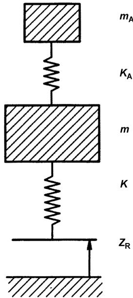
**Figure 2.11.1** ‘Resonant vibration absorber’ system (H. Frahm, 1909).
