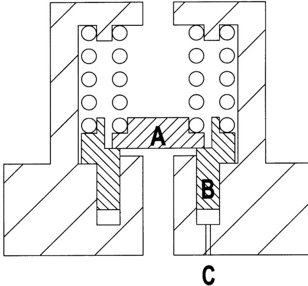
**Figure 6.14.1** Pressure-rate-sensitive valve (Potas, 2004, 2005, 2006).
