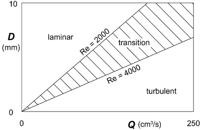
**Figure 5.19.1** Laminar / transition / turbulent flow regimes for various combinations of circular pipe diameter and volumetric flow rate. Density  $860 \text{ kg/m}^3$ , viscosity  $10 \text{ mPa s}$ .
