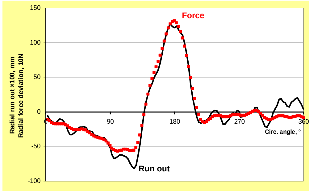
Figure 8.5 – Average of 4 measurements of radial force variation and radial run out in a new rejected 295/80R22.5 truck tire for tuned phases.
