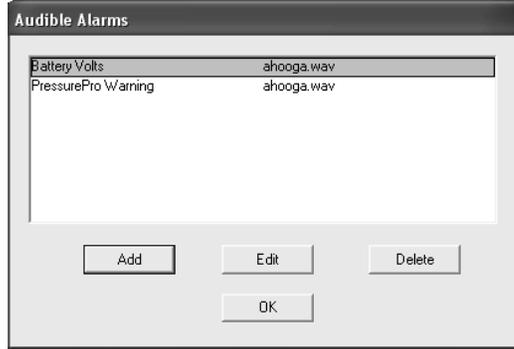
Choose the parameter and trigger value, whether the alarm sounds when the parameter is over or under the value, and how frequently the alarm should sound. For the sound you can use any ".WAV" file - there are a great many defined in the Windows Media directory.
