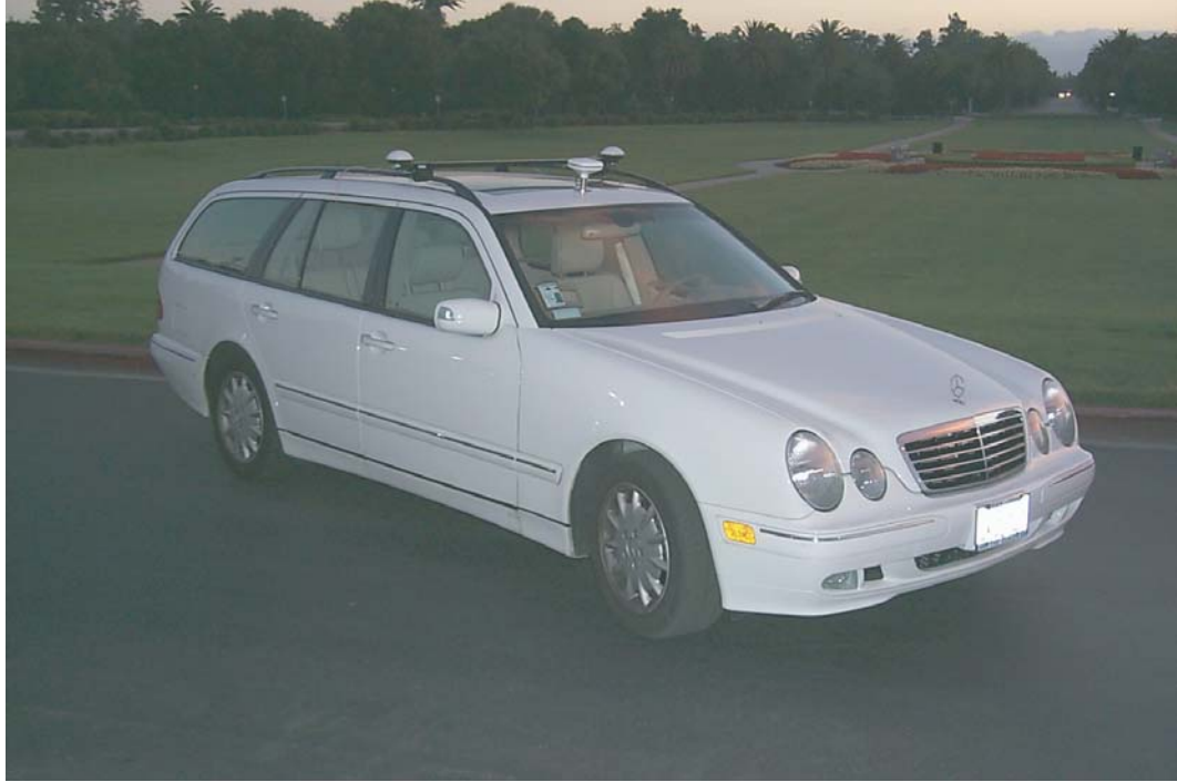
Figure 3.1: Test Vehicle with Two-Antenna GPS Set-up
