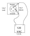
When measuring AC voltage NOR MAL procedure is from Hot to Neutral as shown above on a typical RV 50 AMP Park Power Pedestal receptacle.
